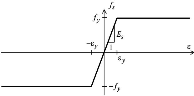
Figure 3. Stress-strain diagram of reinforcing steel in the MCFT
