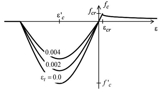
Figure 4. Stress-strain diagram of concrete in de MCFT
