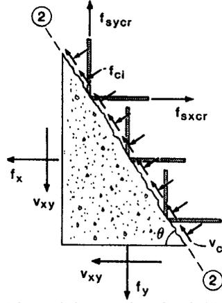
Figure 6. Stresses in a Crack (Vecchio 1986)
