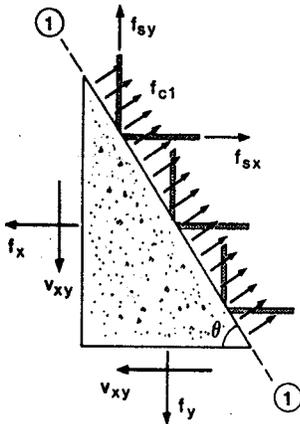
Figure 5. Average Stresses in a Section (Vecchio 1986)
