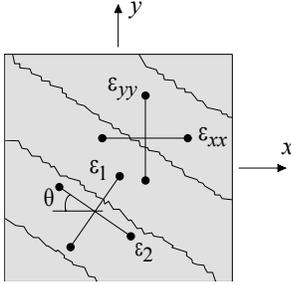
Figure 2. Strains in Reinforced Concrete
