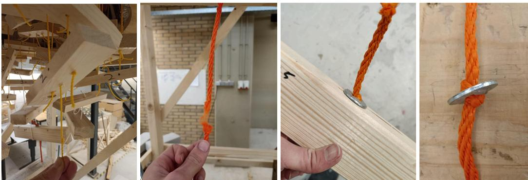
Figure 5.2.3: a) Yellow rope pulled through distribution block. b) Snapped orange rope. c) Knot in orange rope pulled through distribution block. d) Knot in orange rope pulled through metal ring
