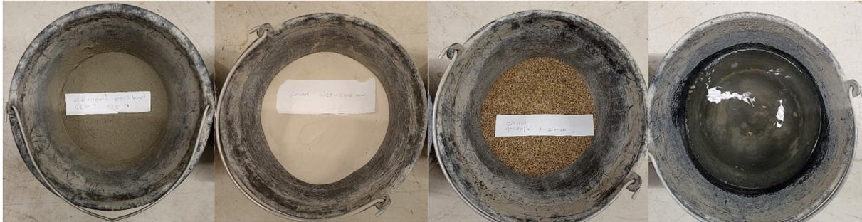
Figure 1.2.9: Ingredients concrete mixture
