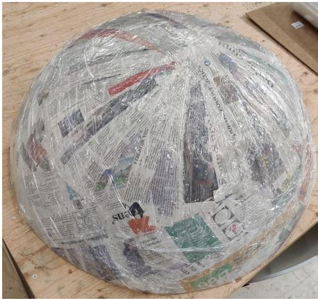
Figure 2.2.1: Mold covered in plastic foil
