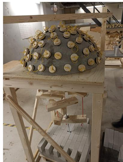
Figure 5.1.2: Shell loaded with 56 bricks
