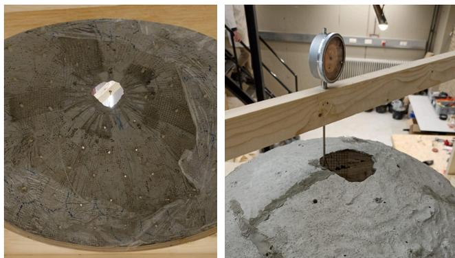
Figure 6.3.2: Failed shell (inside and top view)
