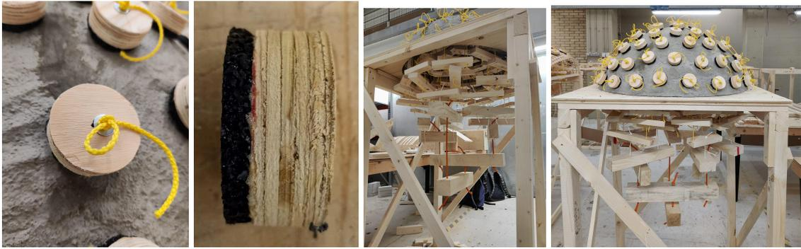
Figure 2.4.3: a) Distribution disk on the shell. b) Side view distribution disk. c) String-distribution block testing contraption. d) Final test set-up
