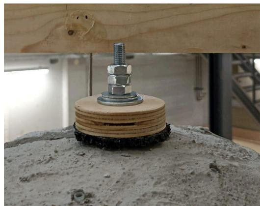
Figure 6.2.1: Steel bar attached to top dome
