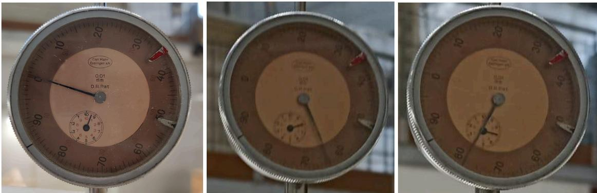
Figure 6.3.1: a) Reference at start of test. b) Deflection at 1,3 kN. c) Deflection at 2,2 kN
