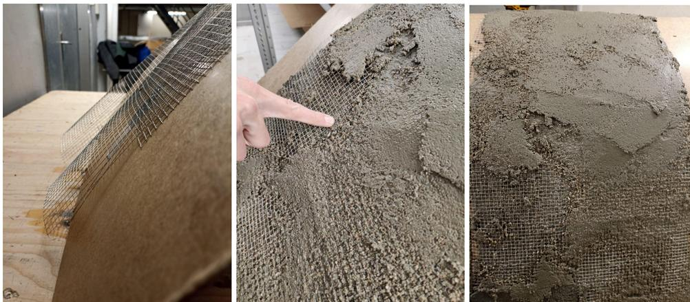
Figure 1.2.6: Testing of pouring concrete on a steep surface. a) Iron mesh. b) Iron mesh visible through concrete. c) Difference in results on the top and on the sides.
