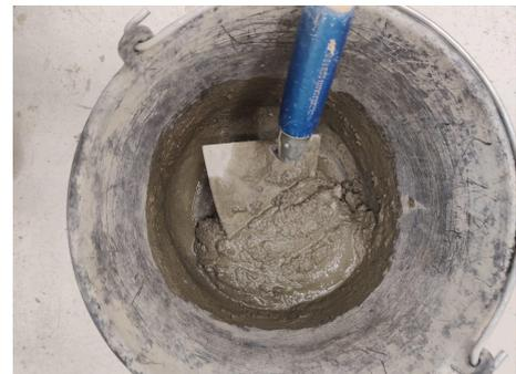
Figure 2.3.3: Consistency concrete
