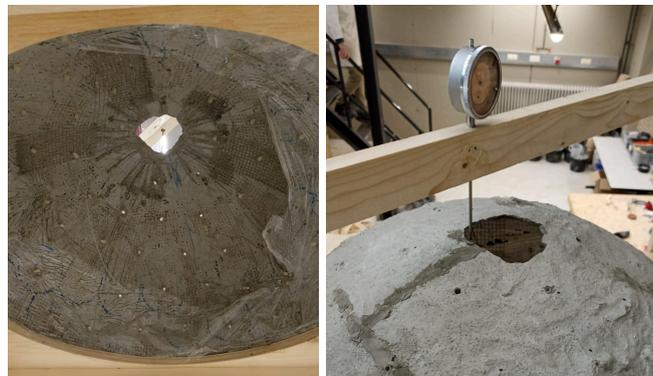
Figure 7.1.4: Shell failed due to punching of point load
