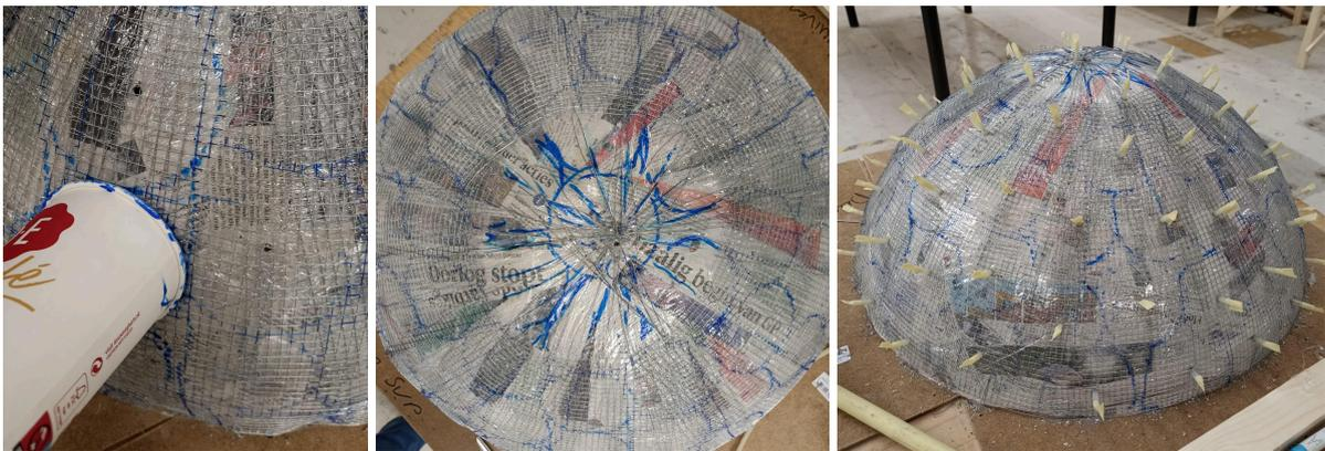
Figure 2.3.1: a) Using a cup to measure even areas. b) Shell mold divided in small areas. c) Tubes placed on shell mold
