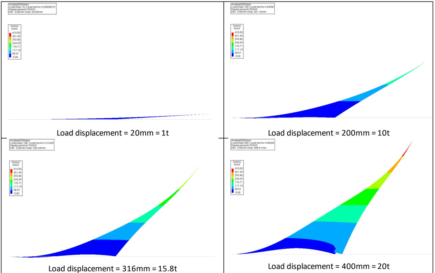
Figure 6: Displacement graphs for  $t = 20\text{mm}$  at different load steps, display scale = 2
