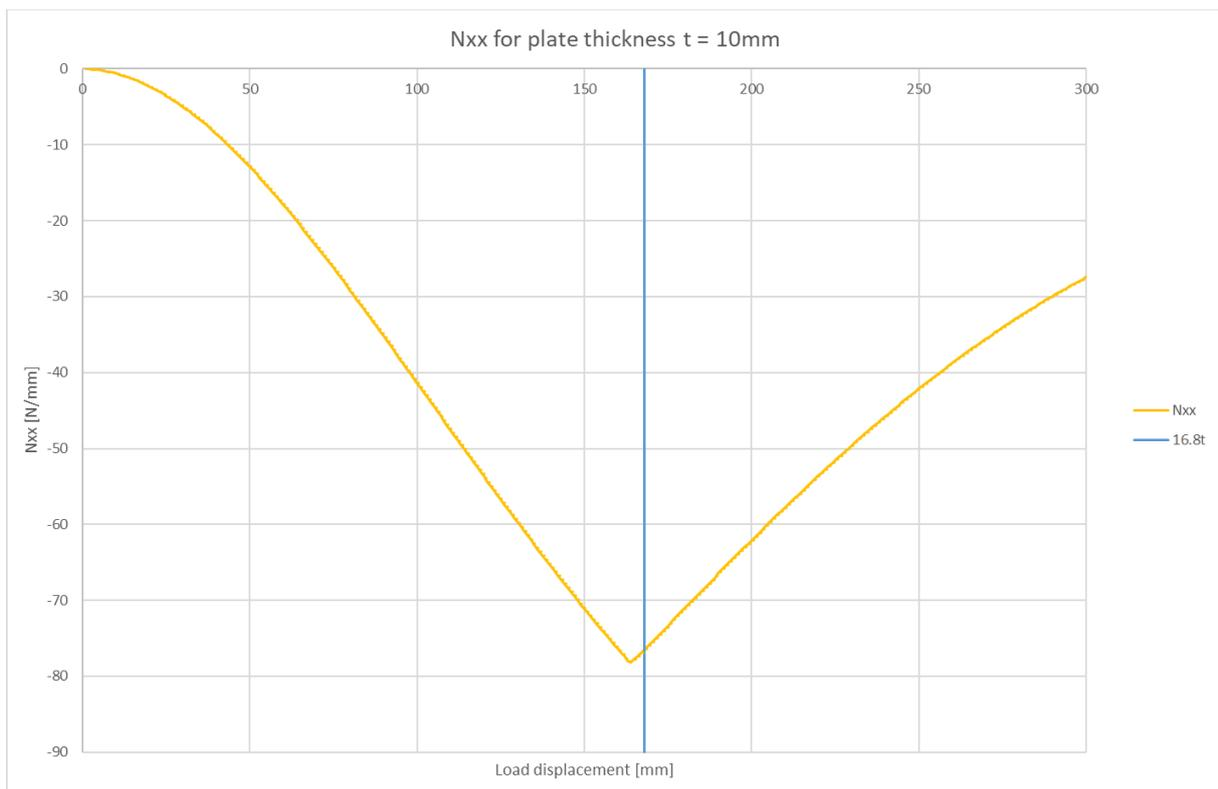
Figure 2:  $N_{xx}$  for  $t = 10\text{mm}$ , buckling point check
