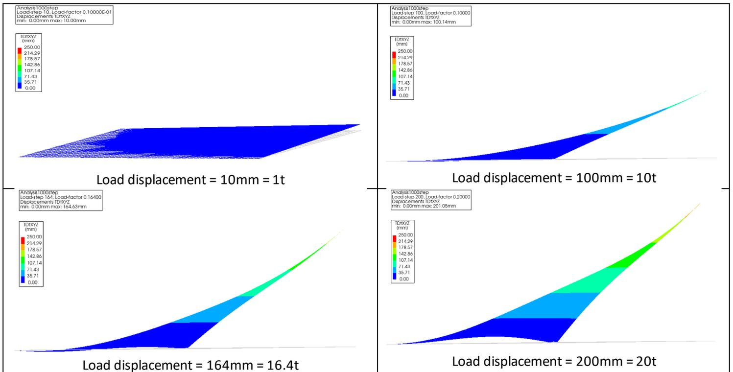
Figure 3: Displacement graphs for  $t = 10\text{mm}$  at different load steps, display scale = 3
