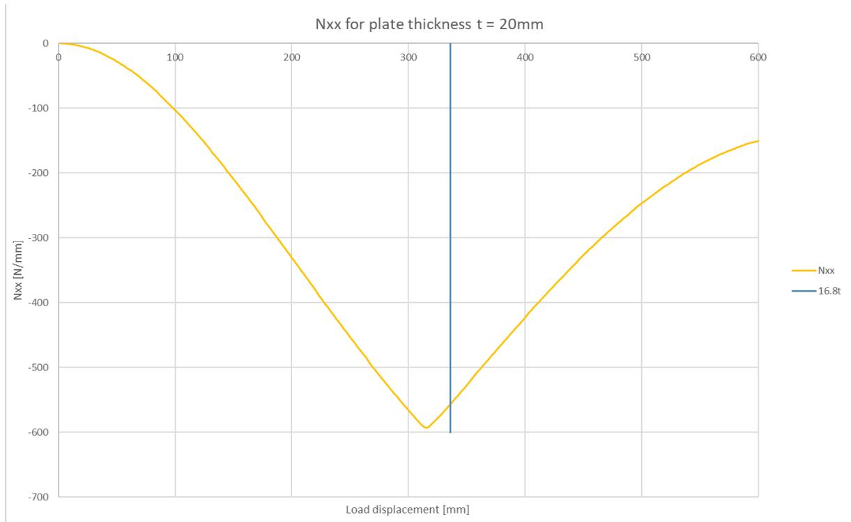
Figure 5:  $N_{xx}$  for  $t = 20\text{ mm}$ , buckling point check
