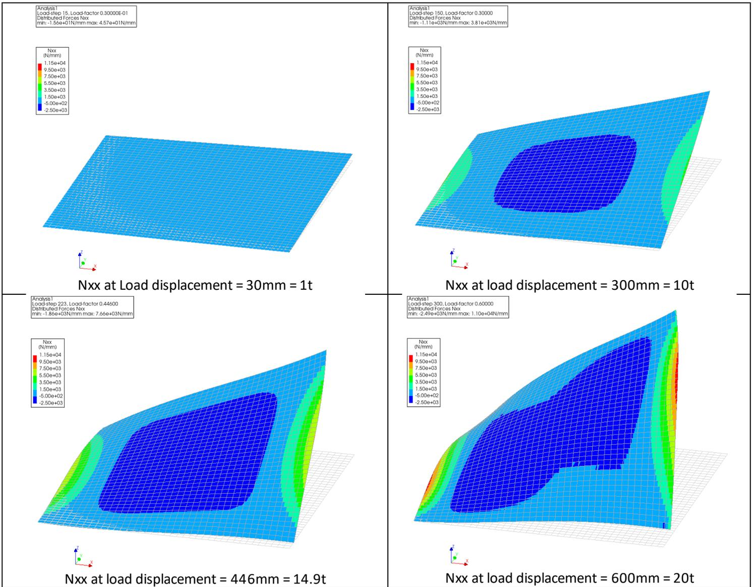
Figure 10:  $N_{xx}$  contour plot for  $t = 30\text{mm}$  at different load steps. Display scale = 1
