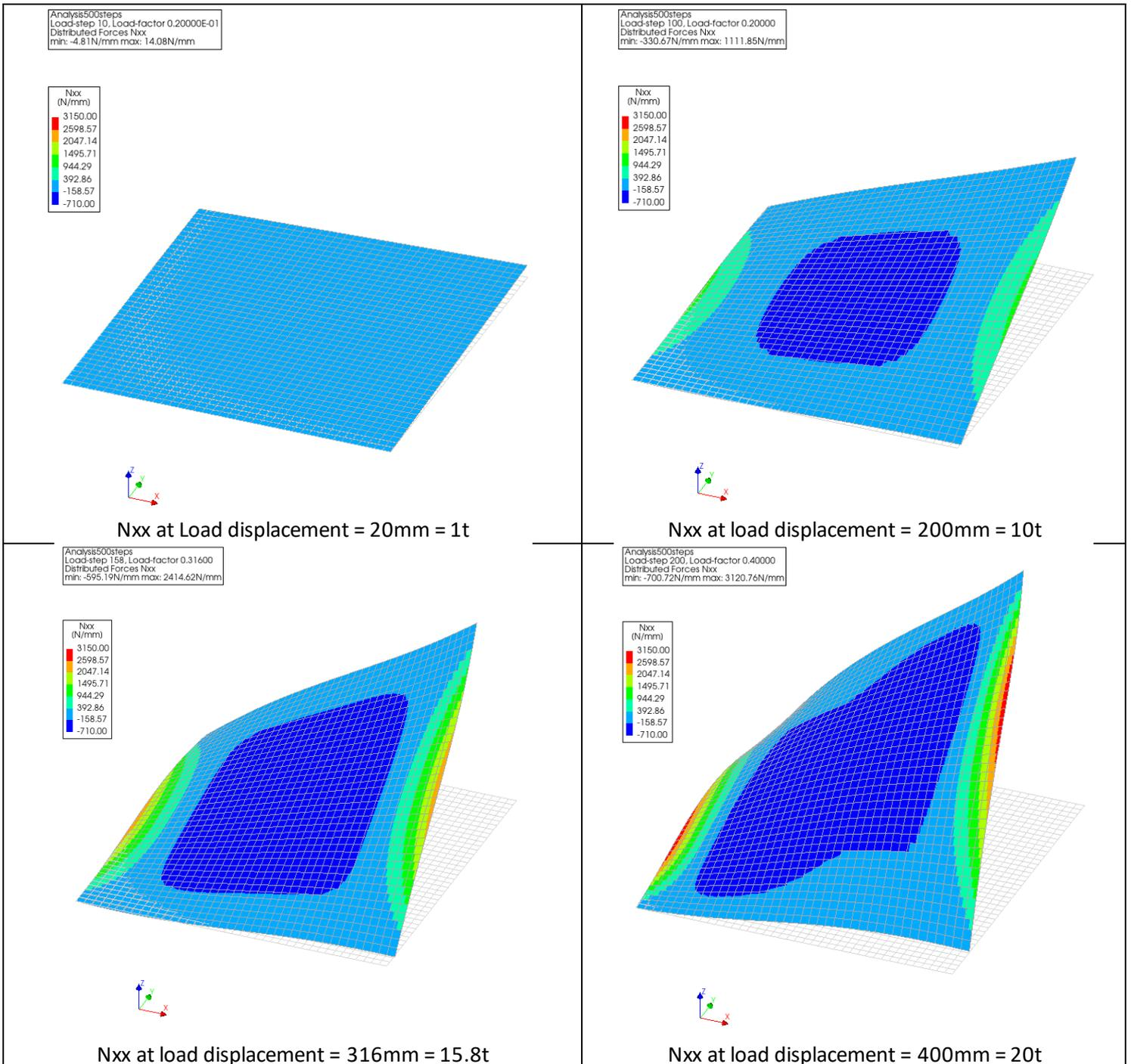
Figure 7: Nxx contour plot for  $t = 20\text{mm}$  at different load steps. Display scale = 3
