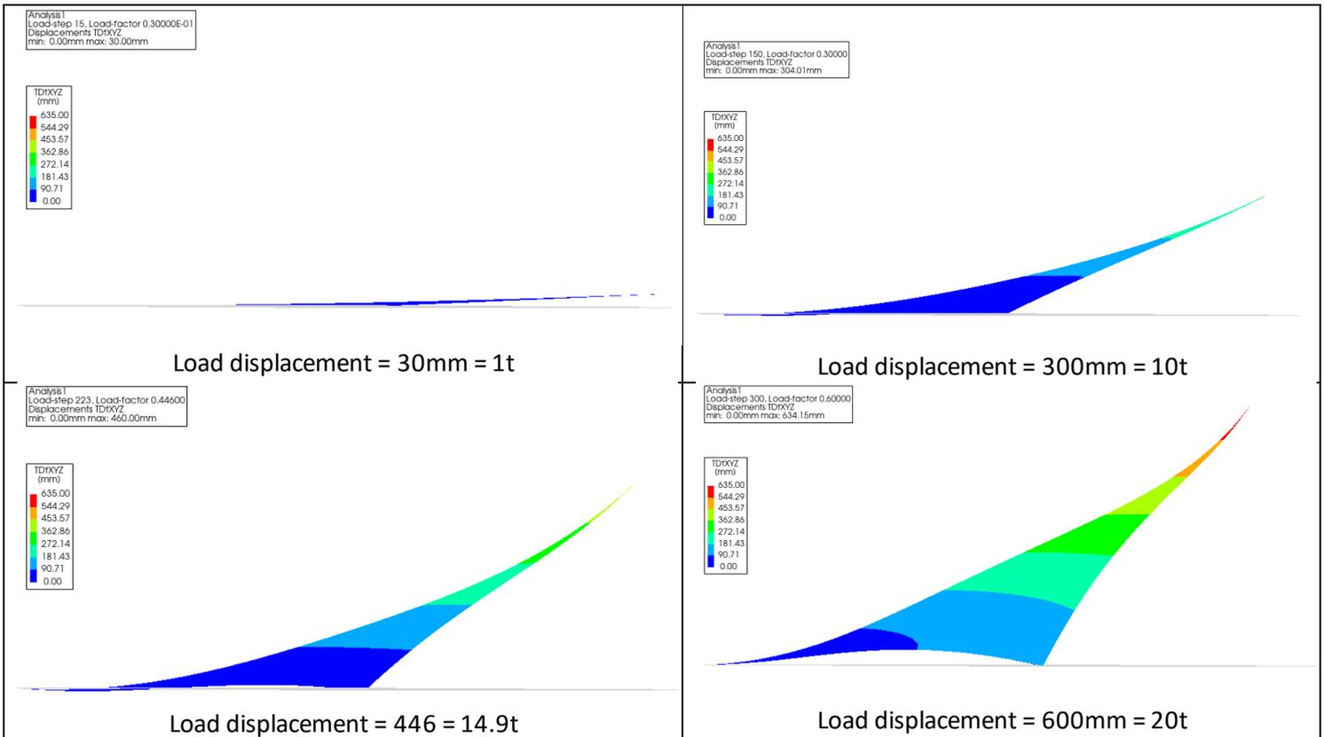
Figure 9: Displacement graphs for t = 30mm at different load steps, display scale = 1
