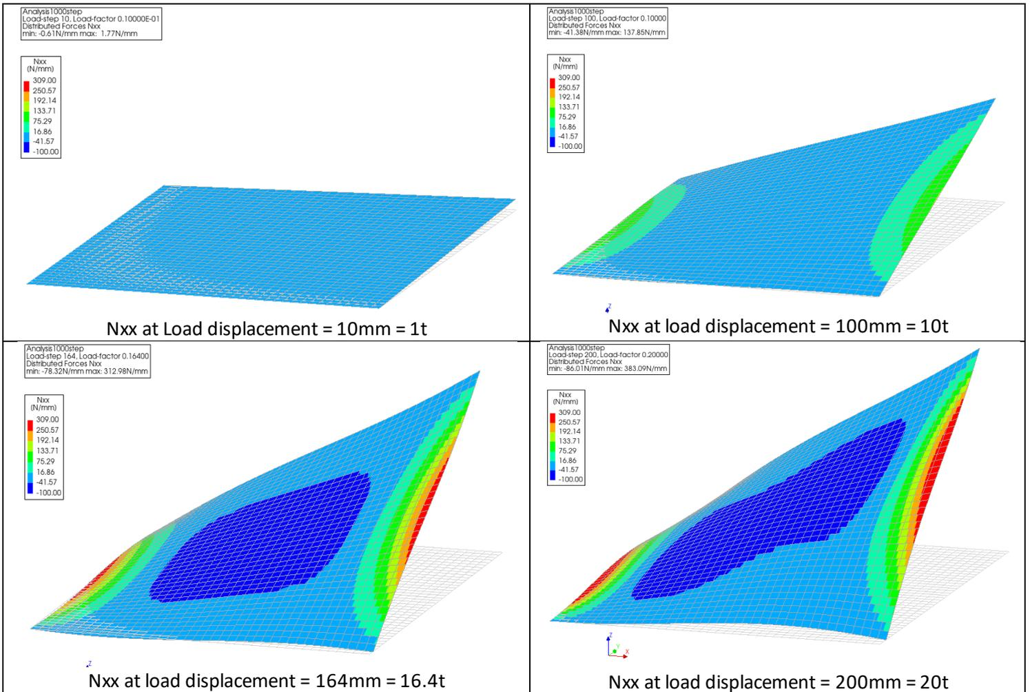
Figure 4: Nxx contour plot for  $t = 10\text{mm}$  at different load steps. Display scale = 3
