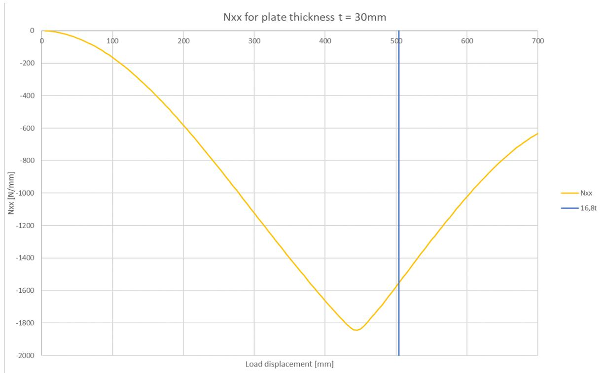
Figure 8:  $N_{xx}$  for  $t = 30\text{mm}$ , buckling point check
