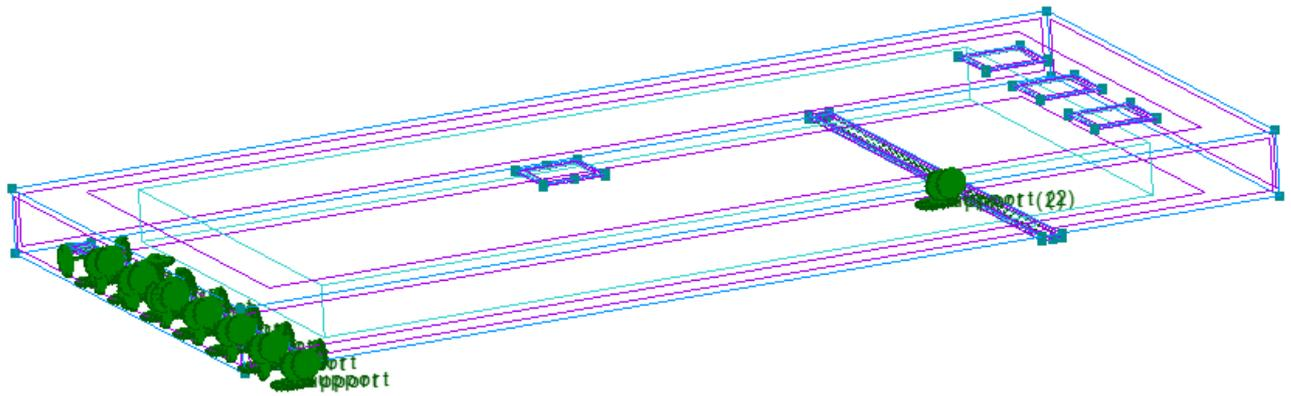
Figure 2.5: Supports and loading plates of the model.
