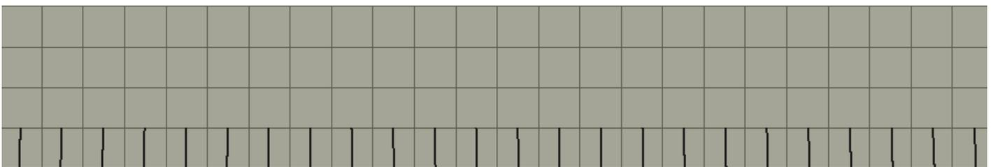
Figure 5.6: Crack forming at 1100 kN with element size of 75 mm.
