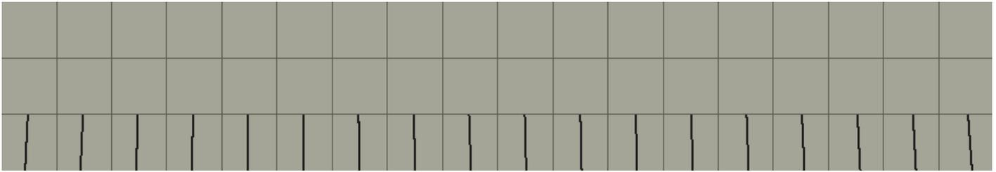
Figure 5.5: Crack forming at 1100 kN with element size of 100 mm.
