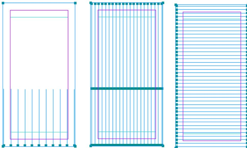
Figure 2.4: Top view of the 10 mm diameter stirrups, the 20 mm diameter stirrups, and the longitude reinforcement.
