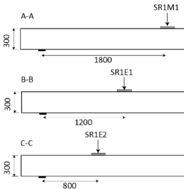
Figure 4.2: : Load locations side view. Units in mm (Zarate Garnica & Lantsoght, 2021).
