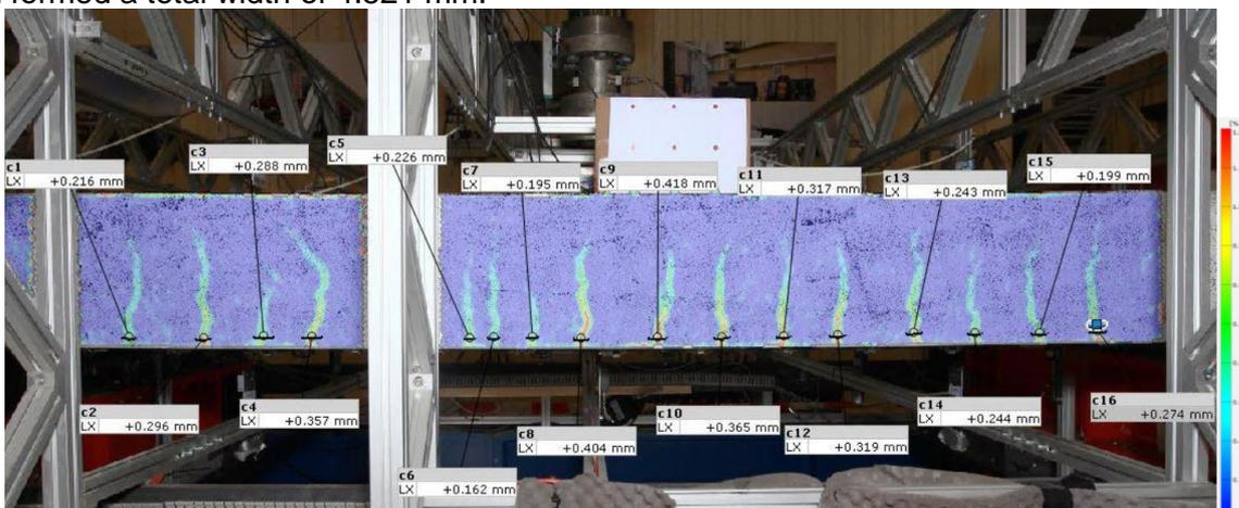
Figure 5.3: Crack width at 1100 kN (Zarate Garnica & Lantsoght, 2021).
