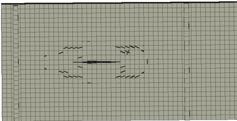
Figure 4.7: Bottom view of crack forming after failure.
