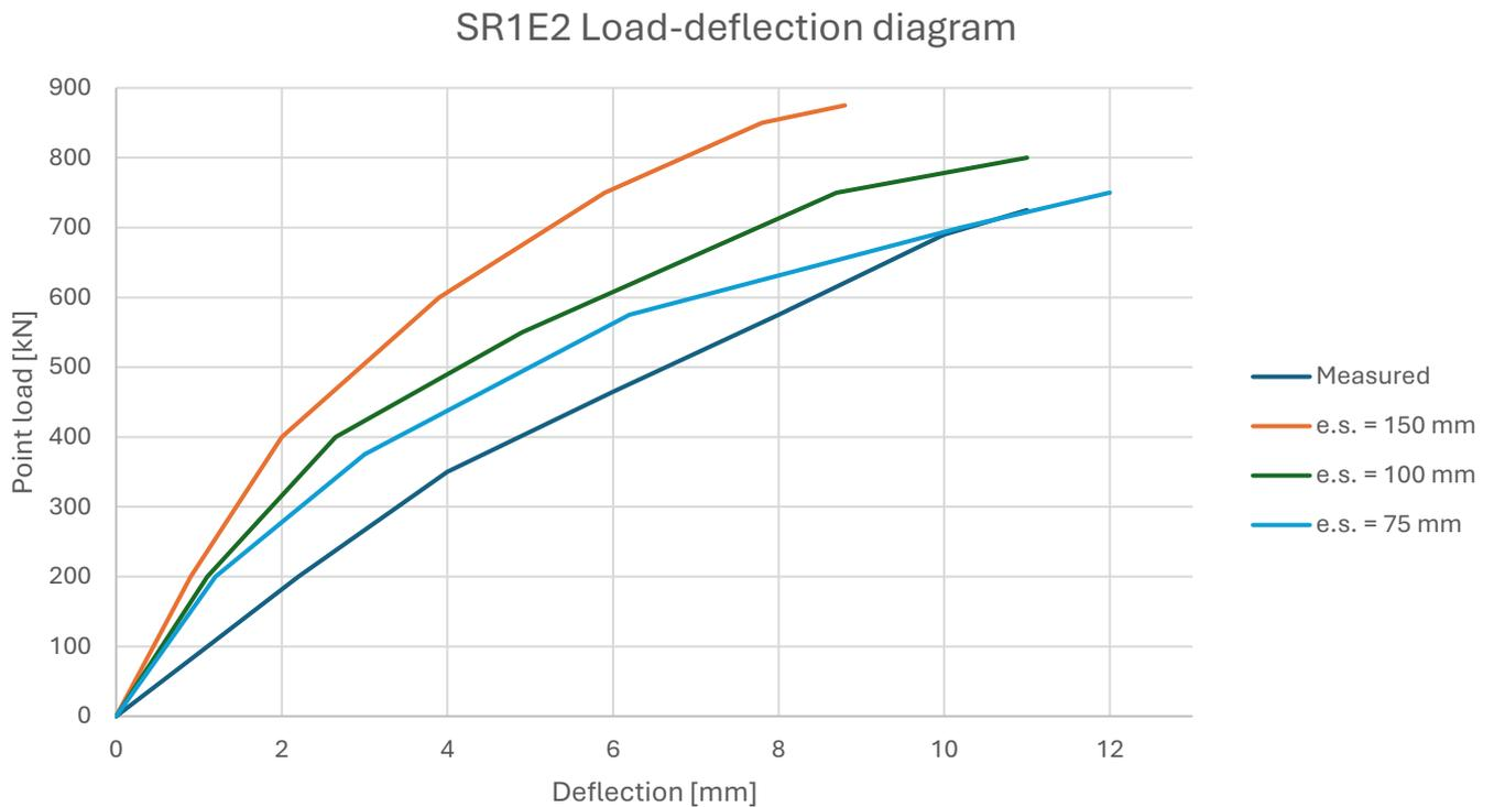
Figure 4.11: SR1E2 Load-deflection diagram.
