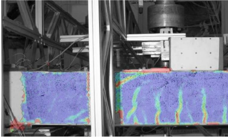
Figure 4.12: Crack pattern at failure load SR1E2 (Zarate Garnica & Lantsoght, 2021).
