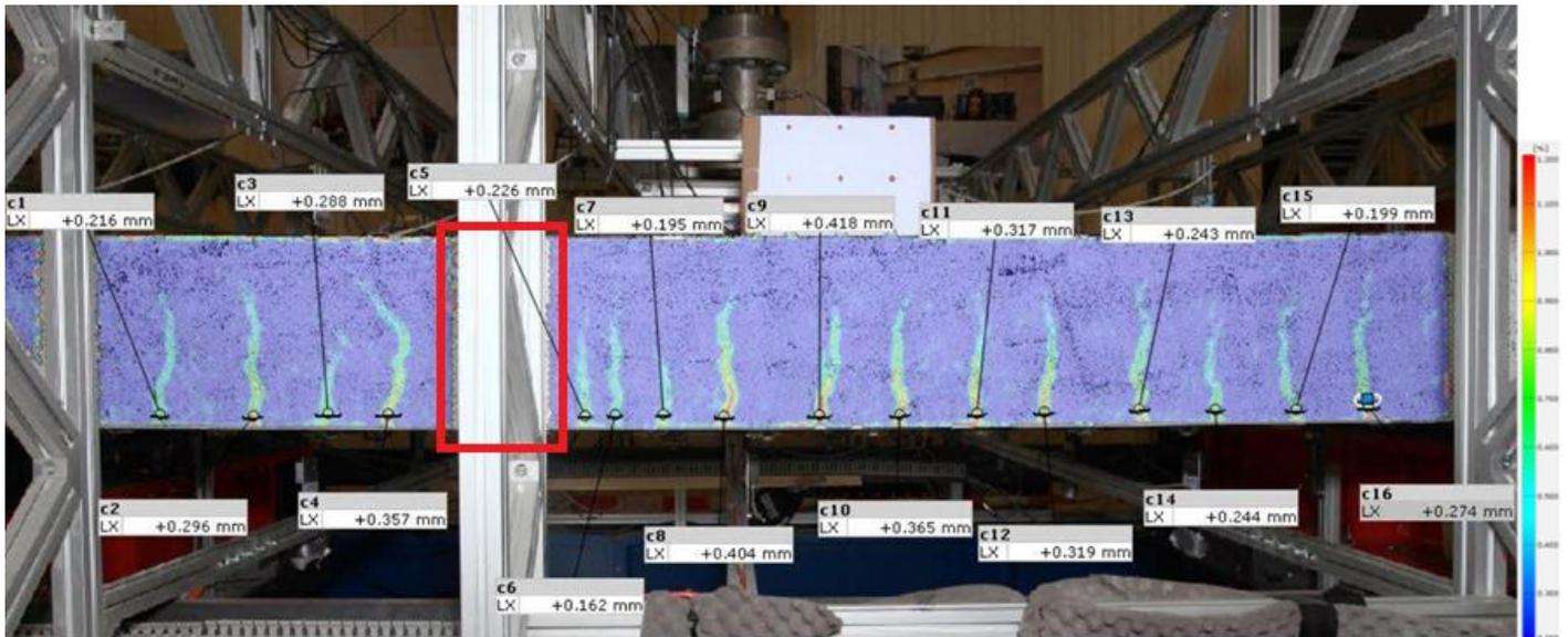
Figure 6.1: Crack width at 1100 kN with highlighted obscure area (Zarate Garnica & Lantsoght, 2021).
