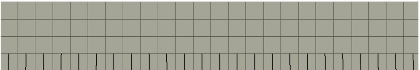
Figure 5.7: Crack forming at 1100 kN with element size of 60 mm.
