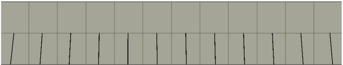
Figure 5.4: Crack forming at 900 kN with element size of 150 mm.
