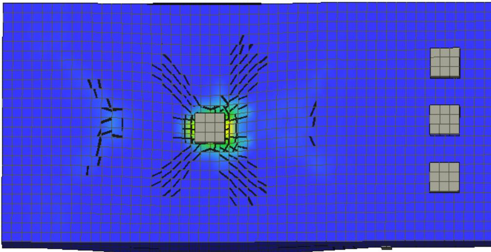
Figure 4.6: Top view of crack forming after failure.
