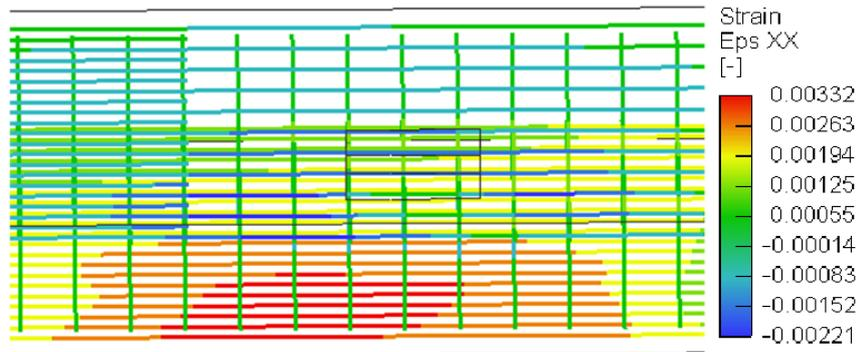
Figure 4.10: Reinforcement strain at a load of 700kN ATENA.
