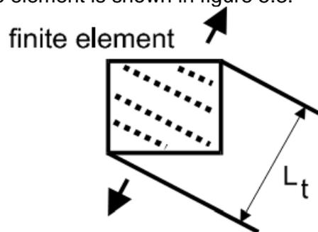
Figure 5.3: Characteristic length  $L_t$  of a finite element (Červenka et al., 2021).
