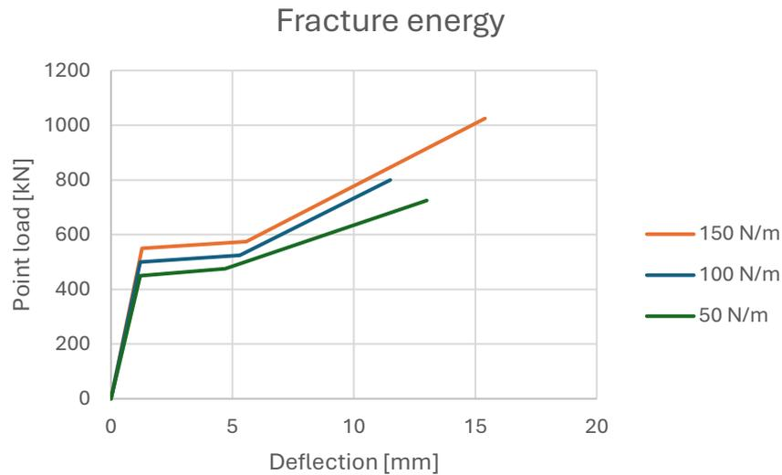
Figure 3.5: Load-deflection diagram for multiple fracture energies.
