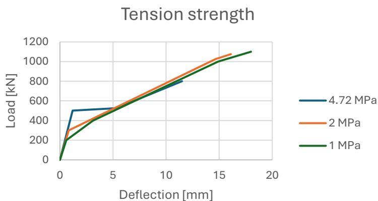
Figure 3.4: Load-deflection diagram for multiple tension strengths.
