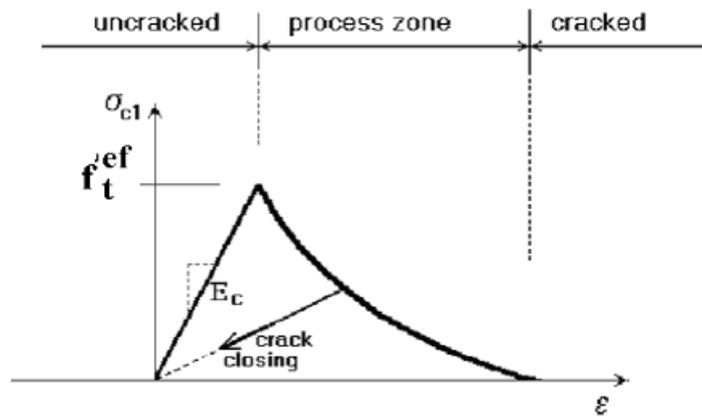
Figure 5.2: Stages of crack opening (Červenka et al., 2021).
