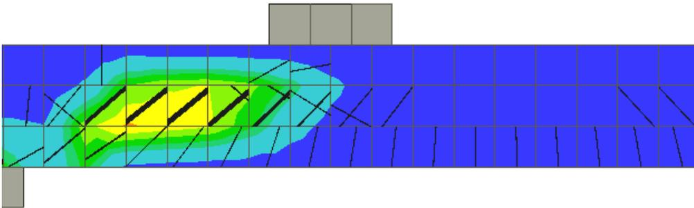
Figure 4.13: Crack pattern at failure load SR1E2 ATENA
