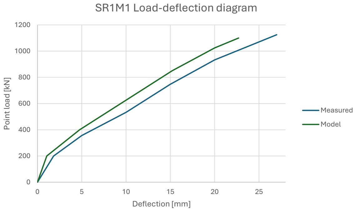
*Figure 3.6: Load-deflection diagram for chosen concrete properties*
