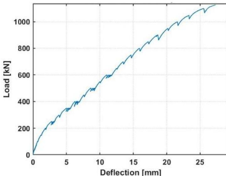
Figure 3.2: Load-deflection diagram SR1M1 test (Zarate Garnica & Lantsoght, 2021).
