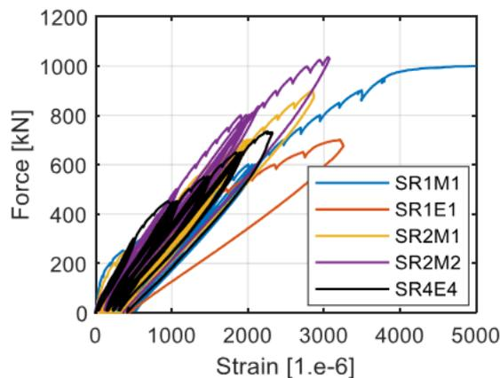
Figure 4.9: Load-strain diagram (Zarate Garnica & Lantsoght, 2021).
