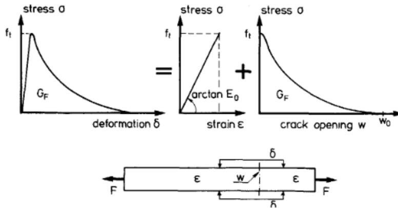
Figure 5.1: Stress-strain diagram Hordijk (Hordijk, 1991).
