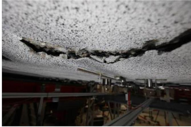
Figure 4.5: Bottom view after failure (Zarate Garnica & Lantsoght, 2021).
