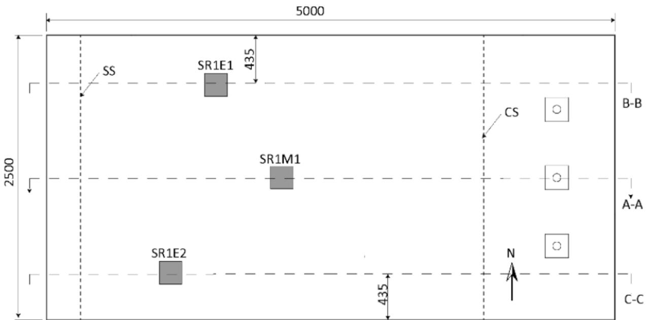
Figure 4.1: Load locations top view. Units in mm (Zarate Garnica & Lantsoght, 2021).
