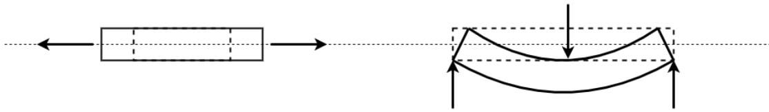
Figure A.2: 2D-loading types
