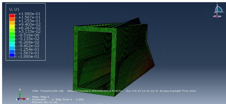
Figure 21: Maximum Displacement of beam 7
