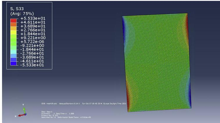
Figure 9: Maximum Stress of beam 1 only constrained in the z-axis
