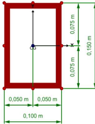
Figure 18: Dimensions of the rectangular closed cross-section
