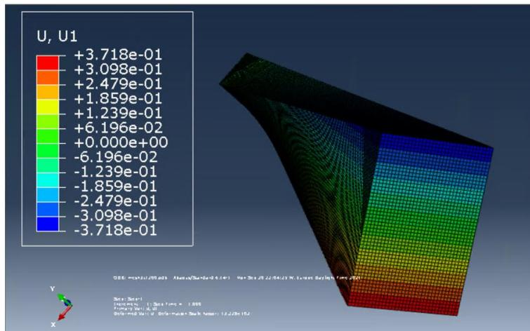
Figure 14: Maximum Displacement of beam 4
