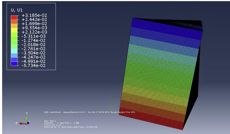
Figure 8: Maximum Displacement of beam 1 only constrained in the z-axis
