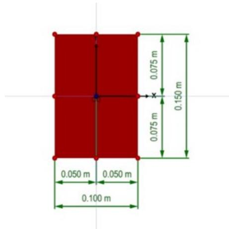
Figure 5: Dimensions of the solid cross-section
