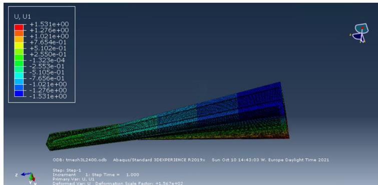
Figure 27: Maximum Displacement of beam 10
