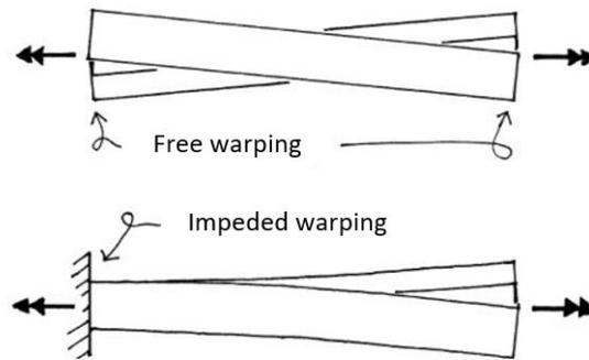
Figure 1: Top views of two I-sections considering respectively the set-up for the Saint-Venant theory and the Vlasov torsion theory (P.C.J.Hoogenboom, 2008)
