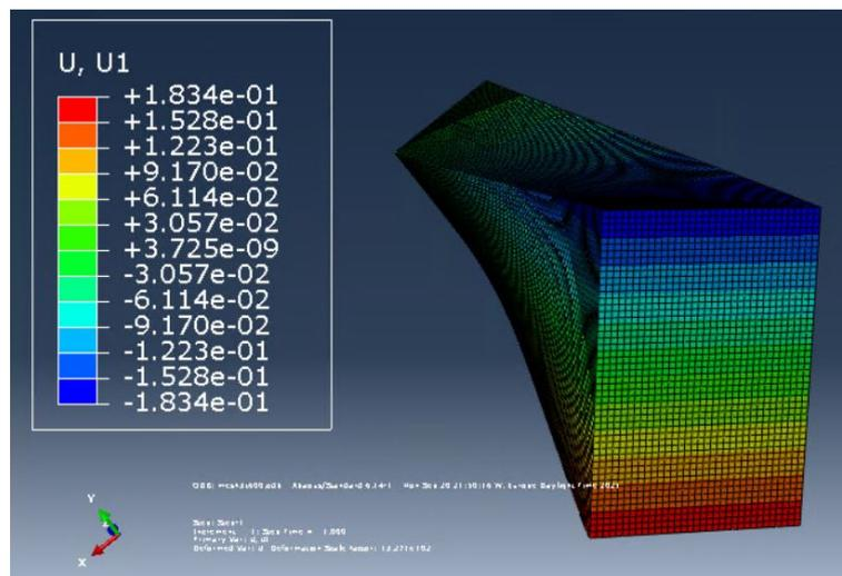
Figure 12: Maximum Displacement of beam 3
