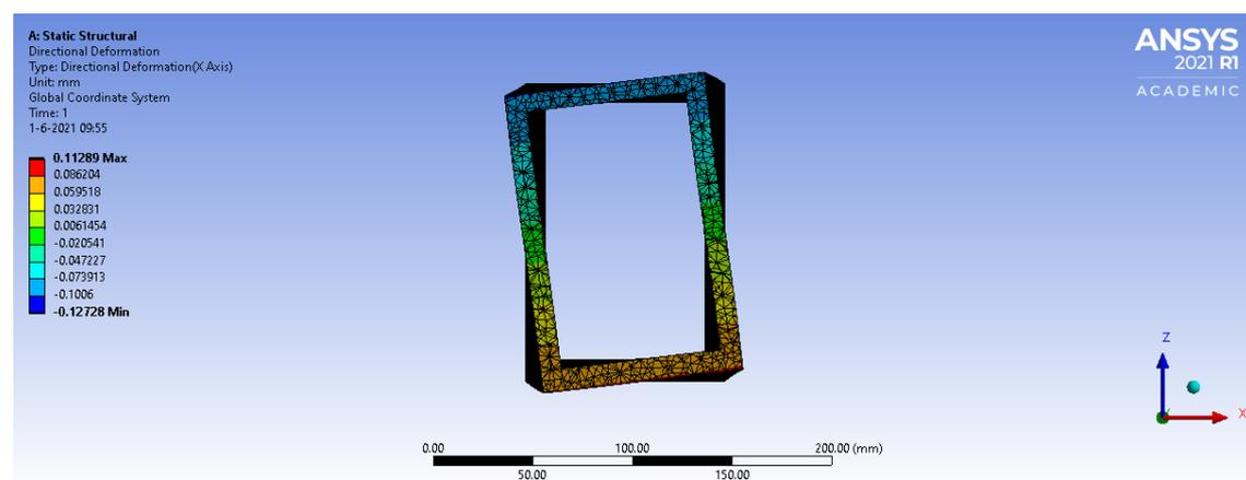
Figure 4.2: Deformation of beam 6 analysed in ANSYS Workbench
