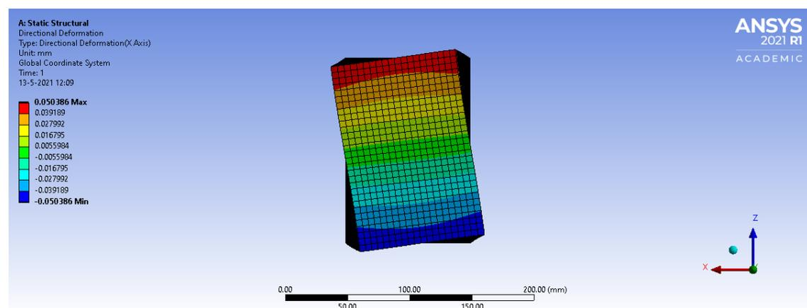
Figure 3.2: Deformation of beam 1 analysed in ANSYS Workbench
