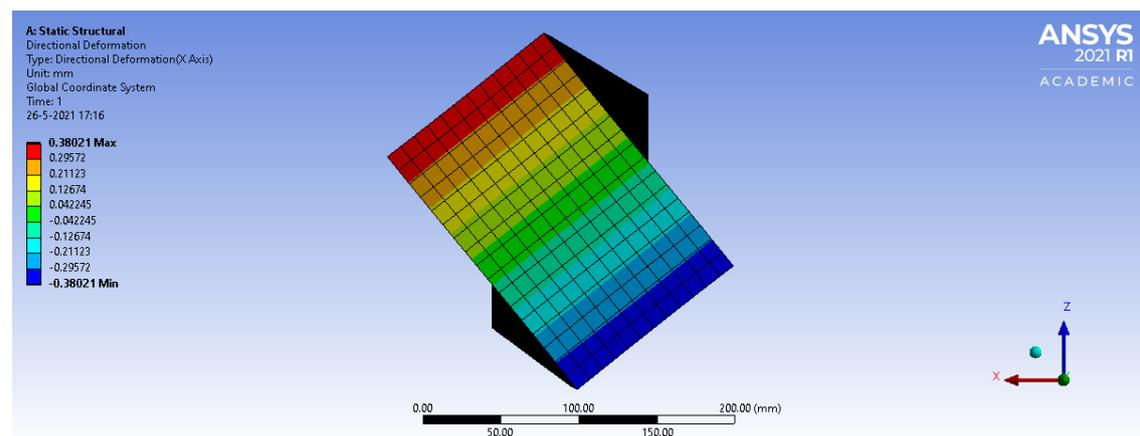
Figure 3.8: Deformation of beam 4 analysed in ANSYS Workbench
