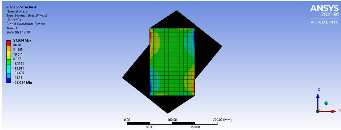
Figure 3.9: Normal stress in beam 4 analysed in ANSYS Workbench
