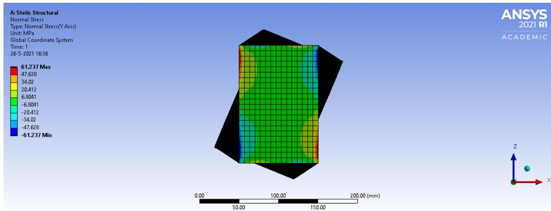
Figure 3.7: Normal stress in beam 3 analysed in ANSYS Workbench
