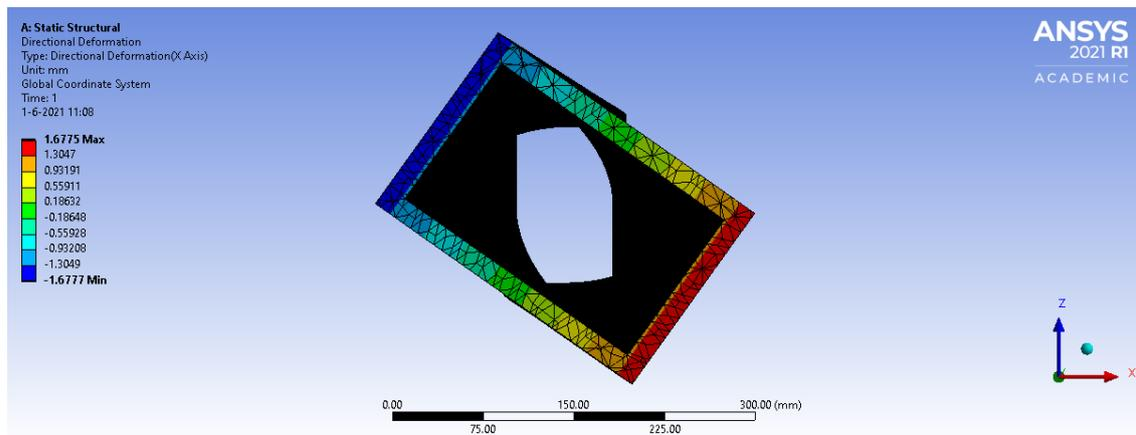
Figure 4.10: Deformation of beam 10 analysed in ANSYS Workbench
