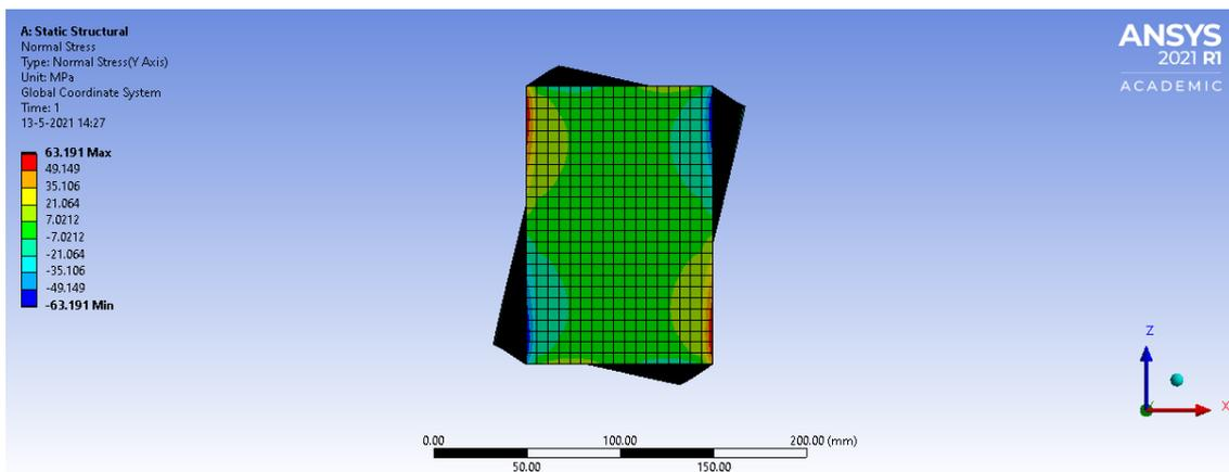
Figure 3.5: Normal stress in beam 2 analysed in ANSYS Workbench
