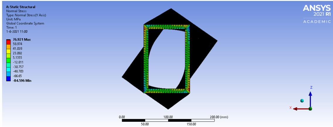
Figure 4.9: Normal stress in beam 9 analysed in ANSYS Workbench
