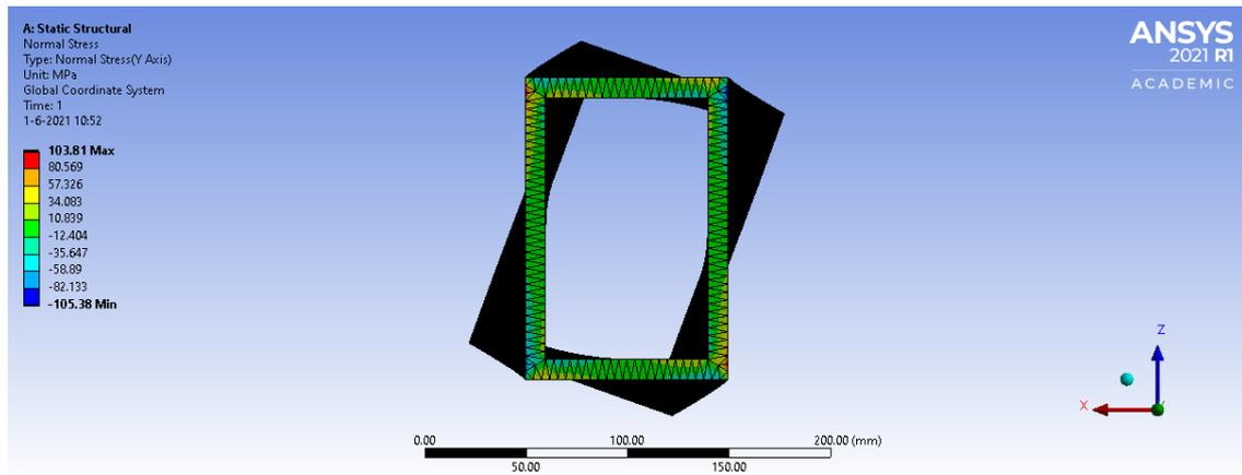
Figure 4.7: Normal stress in beam 8 analysed in ANSYS Workbench
