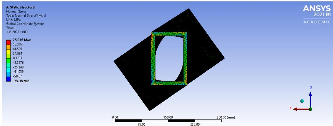
Figure 4.11: Normal stress in beam 10 analysed in ANSYS Workbench
