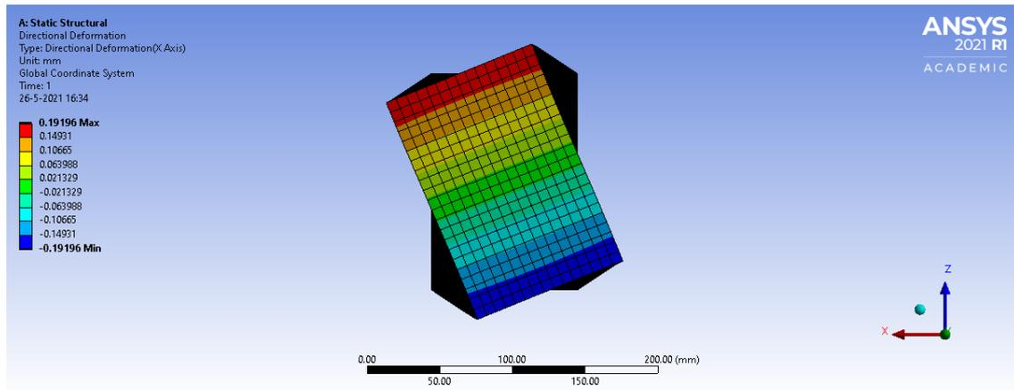
Figure 3.6: Deformation of beam 3 analysed in ANSYS Workbench
