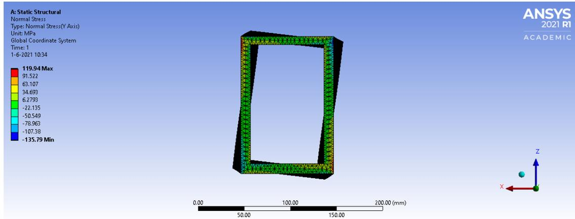
Figure 4.3: Normal stress in beam 6 analysed in ANSYS Workbench
