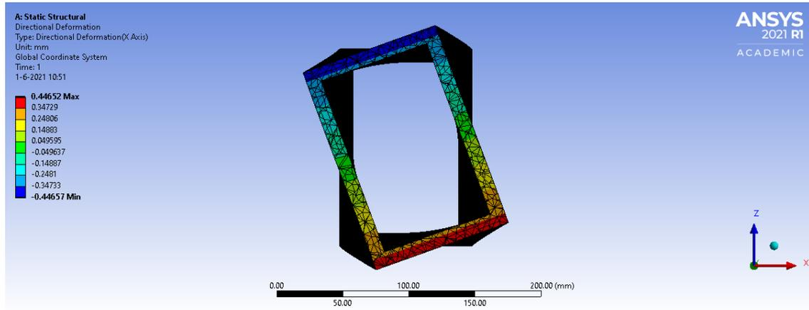
Figure 4.6: Deformation of beam 8 analysed in ANSYS Workbench
