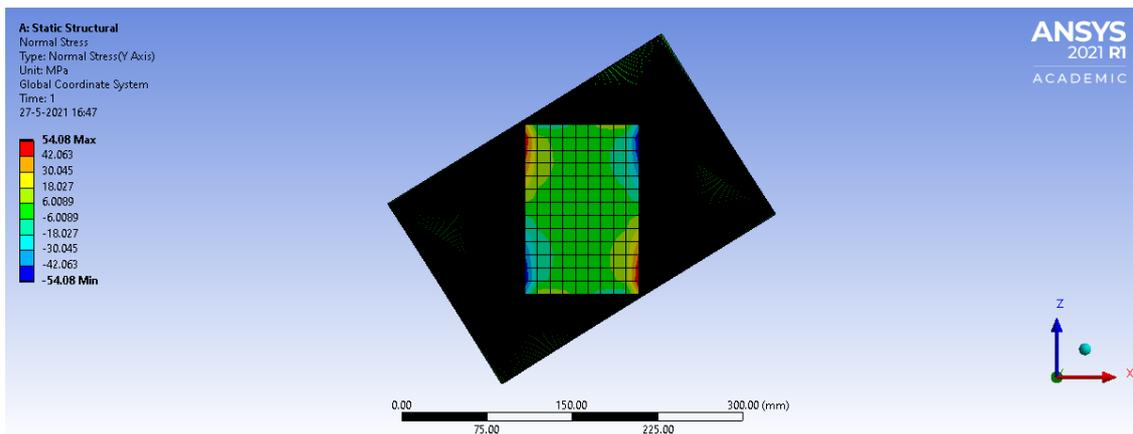
Figure 3.11: Normal stress in beam 5 analysed in ANSYS Workbench
