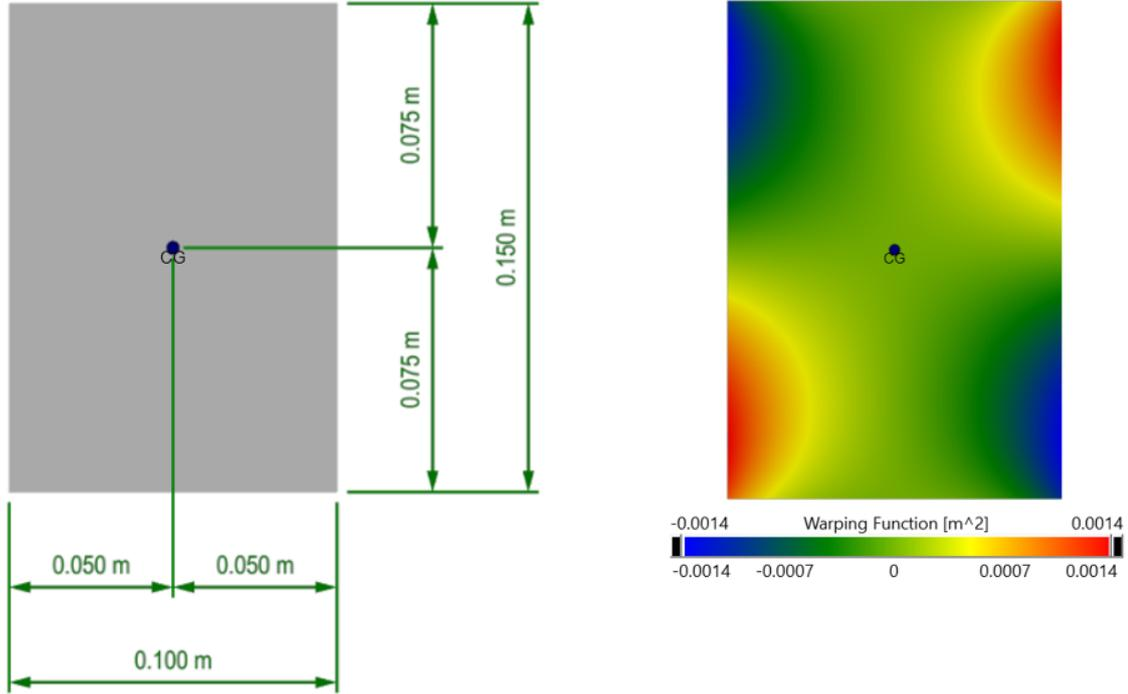
Figure 3.1: (a) Rectangular solid cross-section; (b) Warping function rectangular solid cross-section
