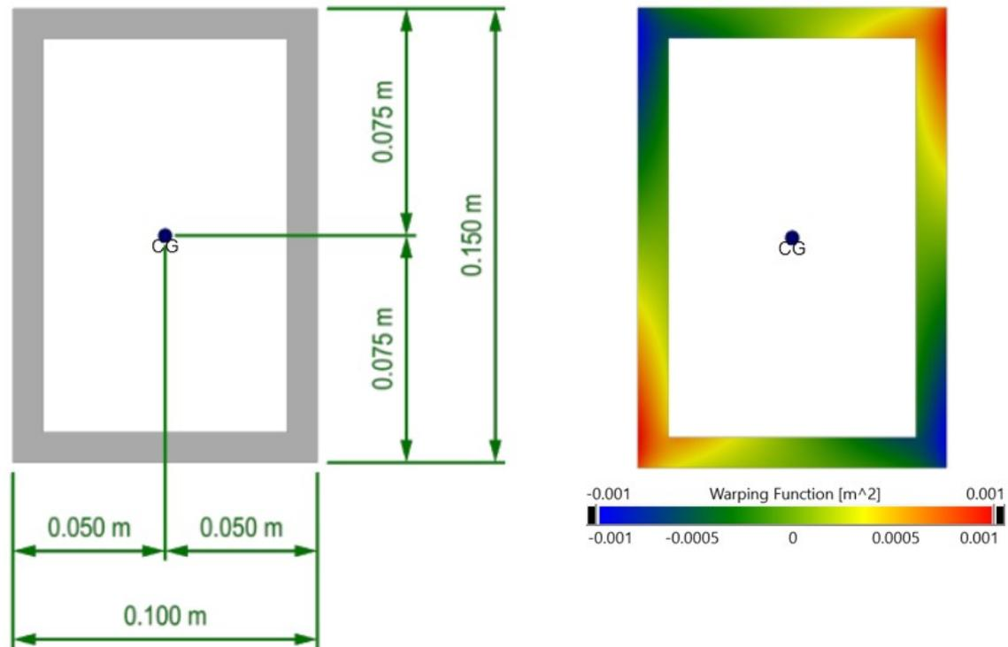
Figure 4.1: (a) Rectangular closed tube cross-section; (b) Warping function rectangular closed tube cross-section
