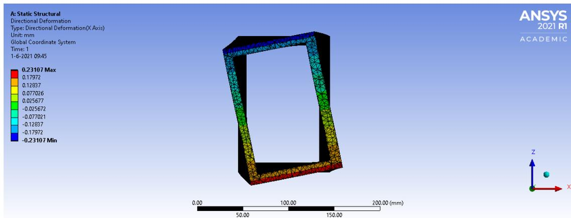
Figure 4.4: Deformation of beam 7 analysed in ANSYS Workbench
