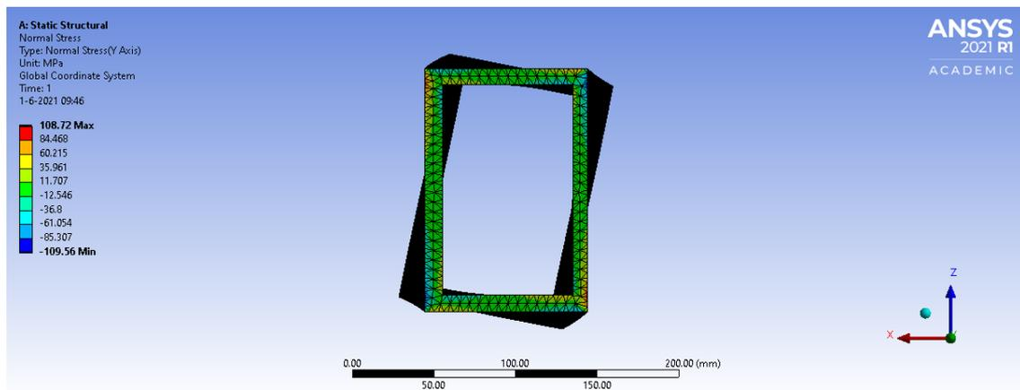
Figure 4.5: Normal stress in beam 7 analysed in ANSYS Workbench
