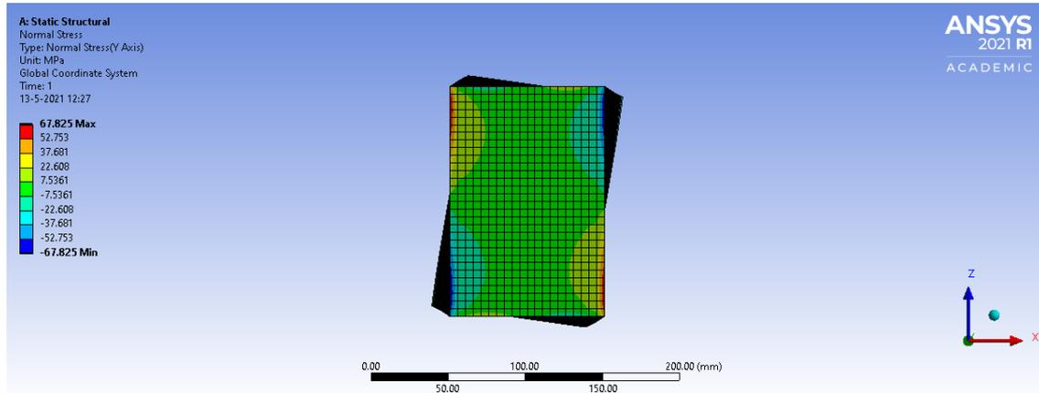
Figure 3.3: Normal stress in beam 1 analysed in ANSYS Workbench
