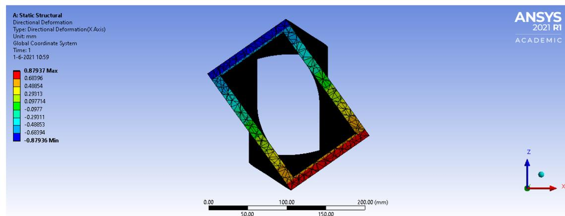
Figure 4.8: Deformation of beam 9 analysed in ANSYS Workbench
