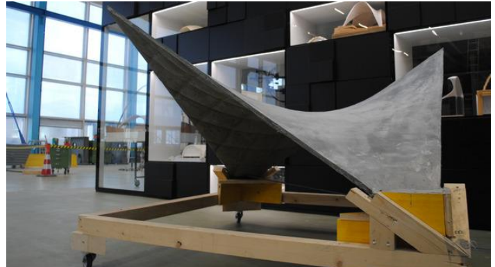
Figure 7 Concrete shell with hybrid cable-net and fabric formwork by D. Veenendaal and P. Block. From “Design process for prototype concrete shells using a hybrid cable-net and fabric formwork,” (Veenendaal & Block, 2014)
