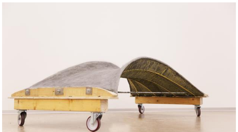
Figure 8 Concrete shell bridge with knitted formwork by M. Popescu et al. From “Building in Concrete with an Ultra-lightweight Knitted Stay-in-place Formwork: Prototype of a Concrete Shell Bridge” (M. Popescu et al., 2014)
