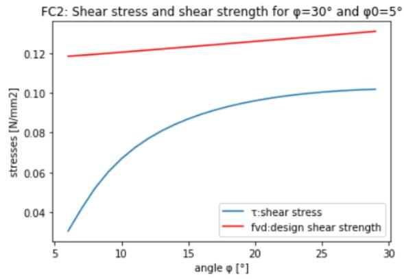
Figure D.20 Stresses at radius  $r = 4m$
