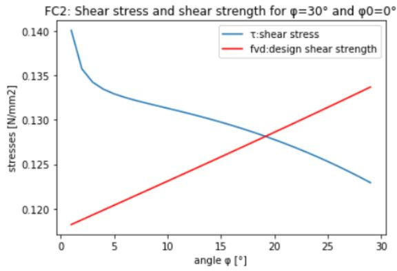
Figure D.11 stresses at radius  $r = 4m$
