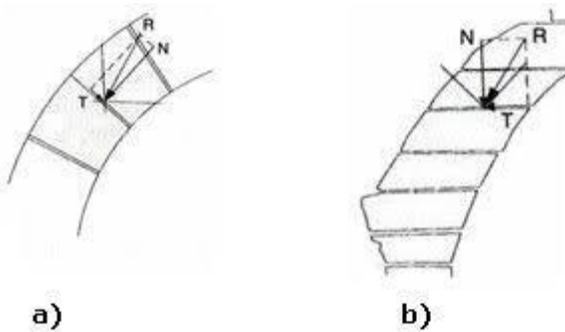
Figure 7.2 Shear forces a) ordinary dome, b) corbelled dome (Tempesta, 2018)
