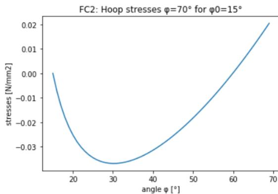
Figure 8.1 Hoop stresses for  $\phi_0=15$ ,  $r=1\text{m}$ , and  $\phi=70$
