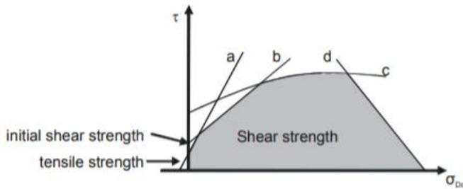
Figure 6.1: Failure mechanisms (Jäger, 2009)
