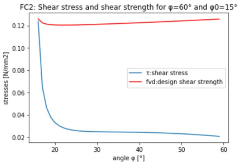
Figure E.2 Shear stresses for  $r = 2.5$  m
