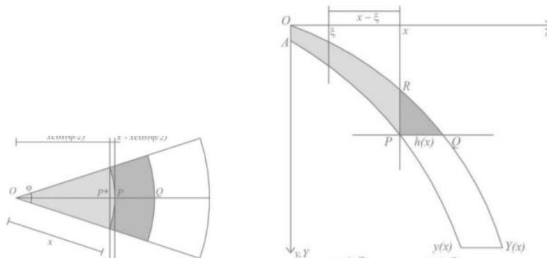
Figure 4.2 Infinitesimal meridian wedge of a dome which equilibrium is evaluated by the corbelling theory (Pilade Foti)
