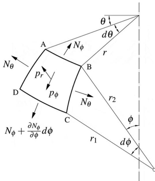
Figure 3.1 Surface element ABCD (Vittone, 2014)
