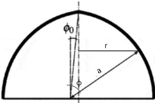
Figure 7.1 Cross-section mathematical shape dome
