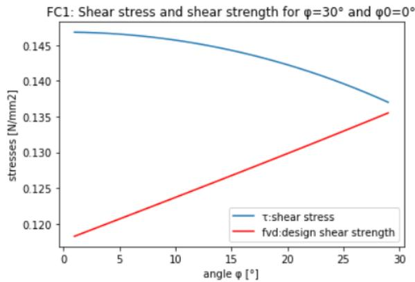
Figure D.8 Stresses at radius  $r = 4m$
