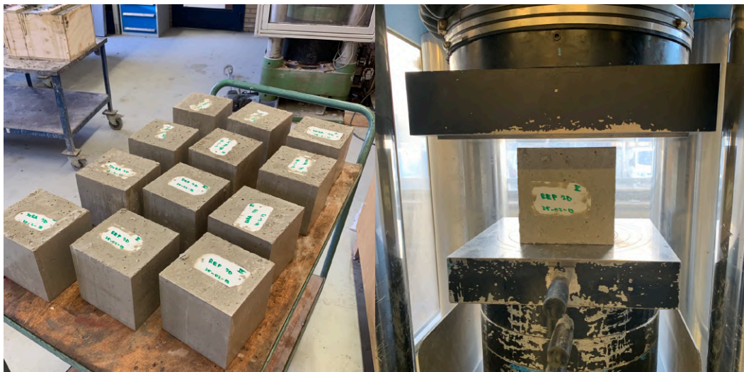
Figure E.5: To be tested cubes (left) and testing device (right)
