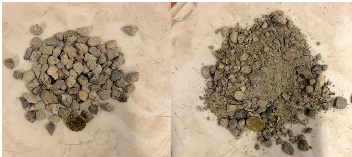
Figure D.1: Before and after product of Los Angeles abrasion test
