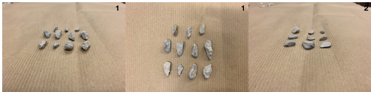
Figure 5.3: Flakiness and shape index particles [1/2]
