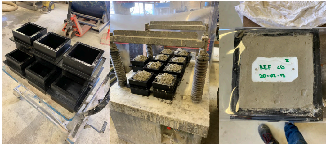
Figure E.4: Oiled cubes (left), vibration table (middle) and labelling (right)
