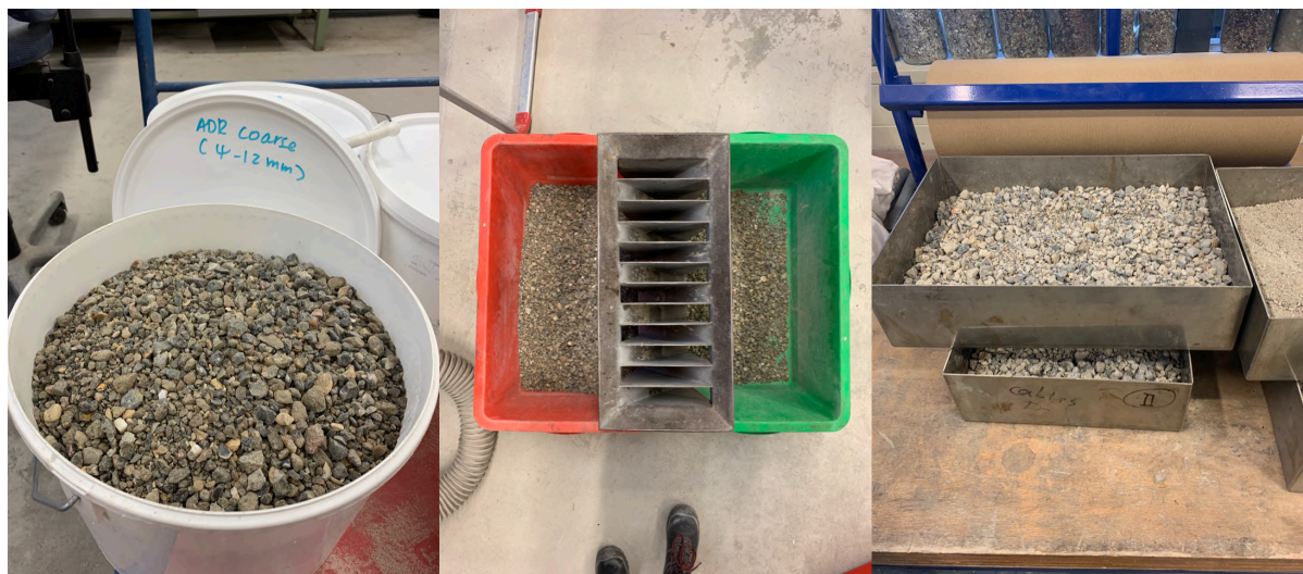
Figure C.1: Coarse aggregate samples
