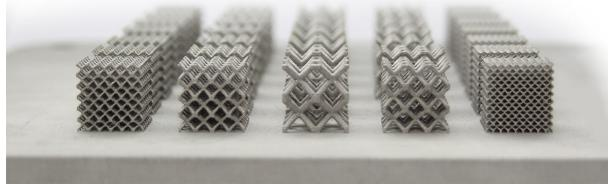
Figure 1: Lattice-structure built on Renishaw AM250 metal AM system (Renishaw, n.d.)
