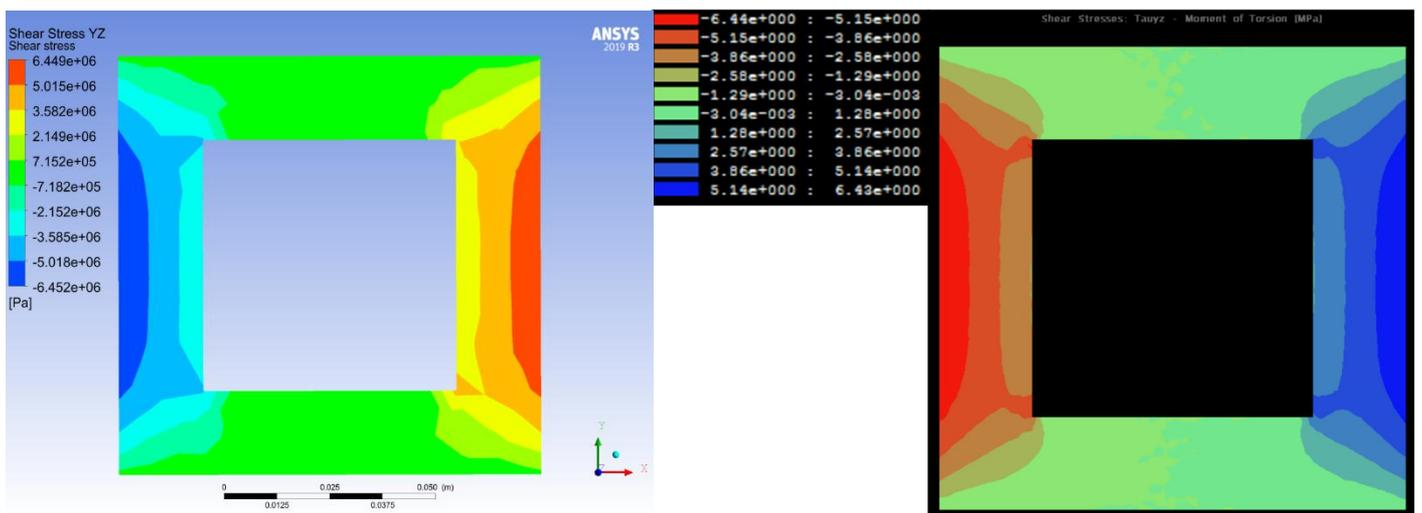
Figure 54 The contour plots of the shear stresses in the YZ plane. Left; Results from Ansys. Right; Results from ShapeDesigner
