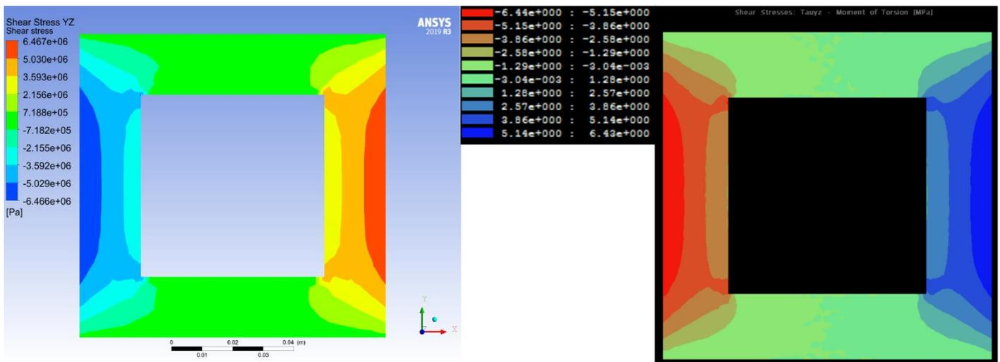
Figure 48 The contour plots of the shear stresses in the YZ plane. Left; Results from Ansys. Right; Results from ShapeDesigner
