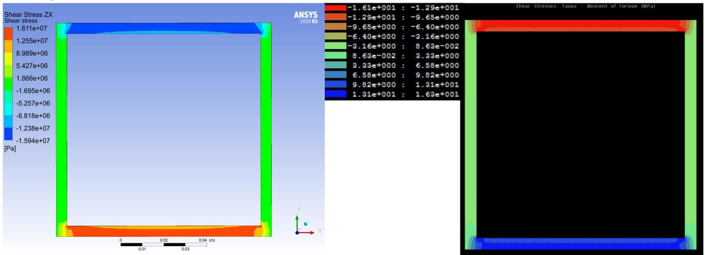
Figure 36 The contour plots of the shear stresses in the XZ plane. Left; Results from Ansys. Right; Results from ShapeDesigner
