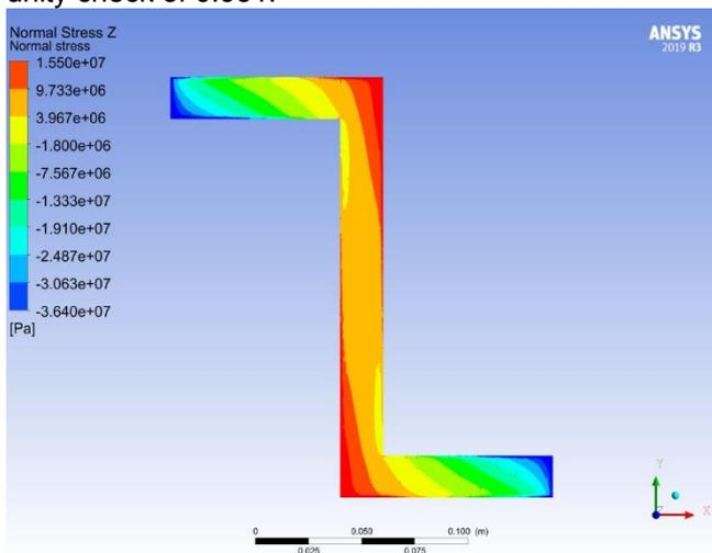
**Figure 24** The normal stress in Z-direction at the fixed end with a rescaled legend
