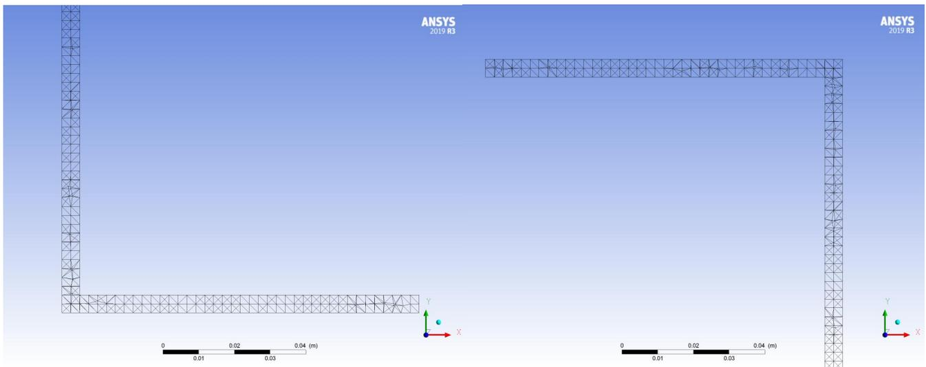
Figure B2 Meshing of beam 2. Left; Bottom flange. Right; Top flange
