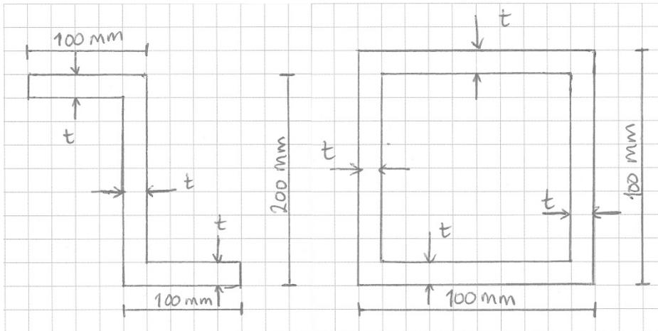
Figure 1 The dimensions of the Z profile (left) and the hollow square profile (right)
