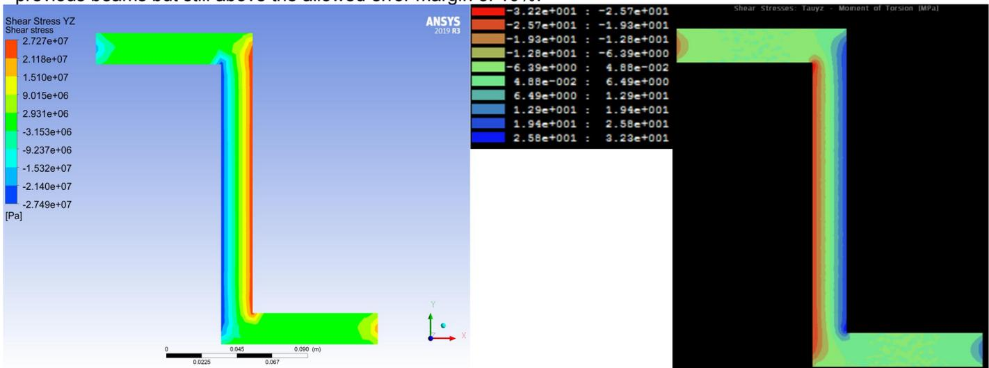
Figure 32 The contour plots of the shear stresses in the YZ plane. Left; Results from Ansys. Right; Results from ShapeDesigner
