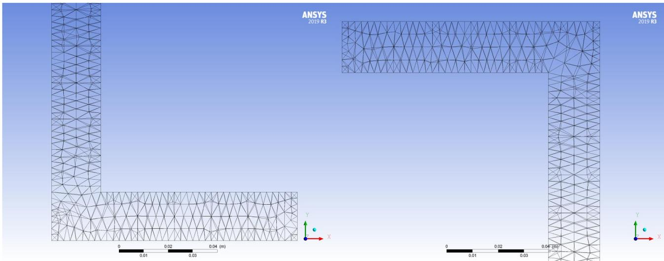
Figure B4 Meshing of beam 4. Left; Bottom flange. Right; Top flange
