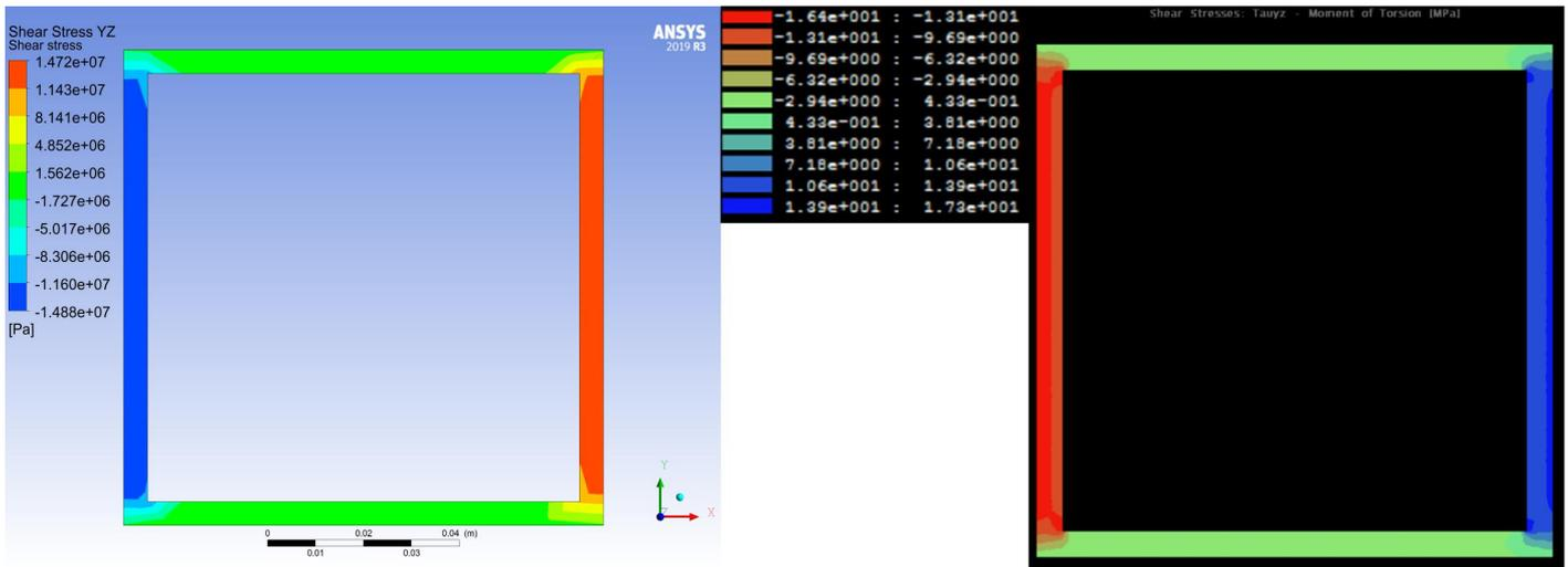
Figure 43 The contour plots of the shear stresses in the YZ plane. Left; Results from Ansys. Right; Results from ShapeDesigner
