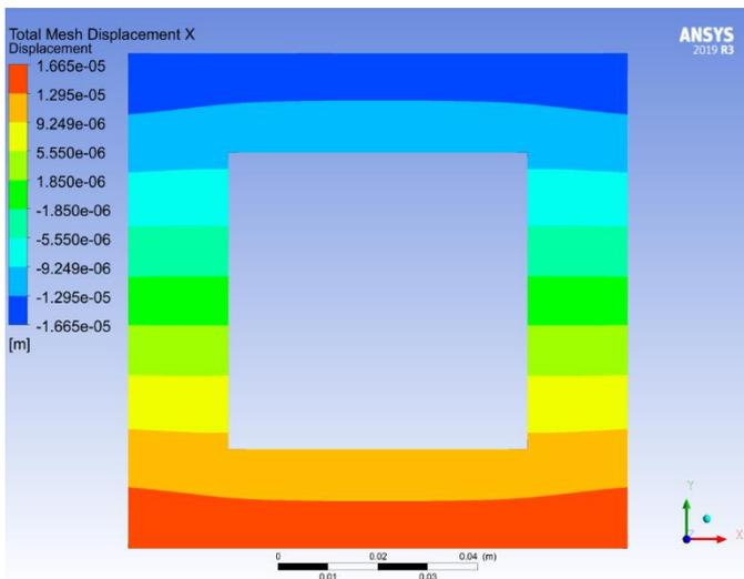
Figure 44 The horizontal displacement of beam 7 from Ansys
