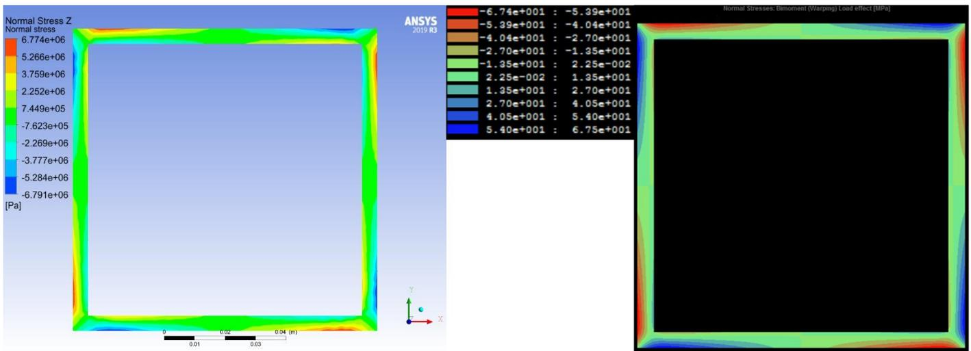
Figure 40 The contour plots of the normal stresses in Z-direction. Left; Results from Ansys. Right; Results from ShapeDesigner
