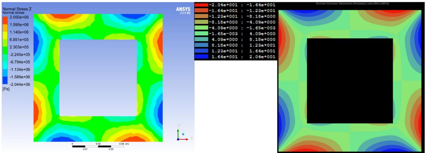
Figure 45 The contour plots of the normal stresses in Z-direction. Left; Results from Ansys. Right; Results from ShapeDesigner
