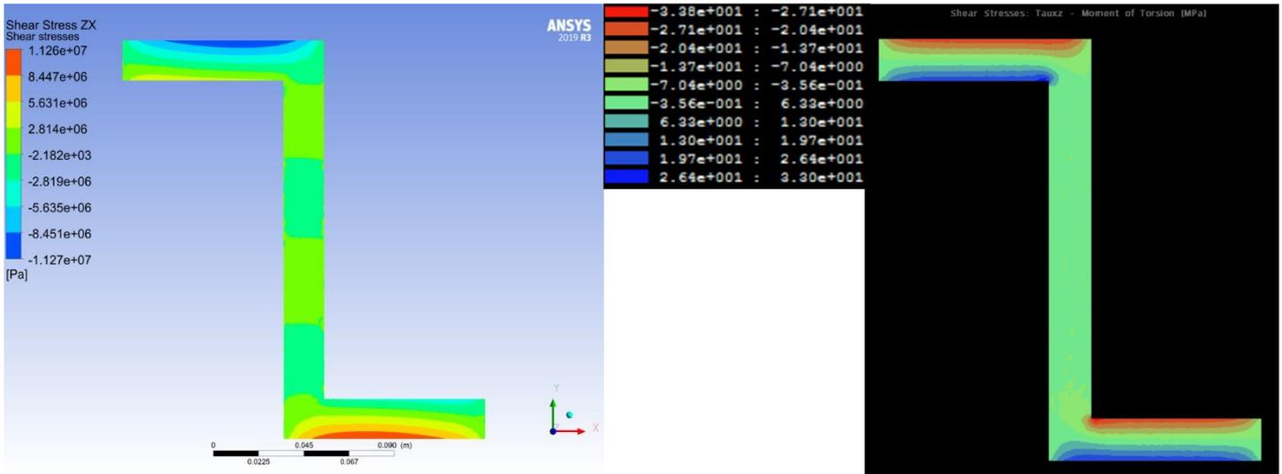
Figure 25 The contour plots of the shear stresses in the XZ plane. Left; Results from Ansys. Right; Results from ShapeDesigner
