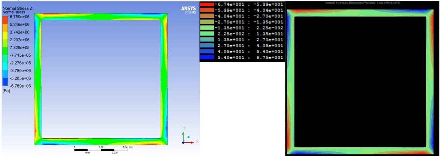
Figure 34 The contour plots of the normal stresses in Z-direction. Left; Results from Ansys. Right; Results from ShapeDesigner
