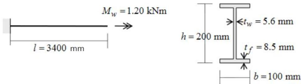
Figure 2 The clamped test beam with a length of 3.4 m undergoing a torsional load of 1.2 kNm, together with the dimensions of the test beam (Hoogenboom, 2019)
