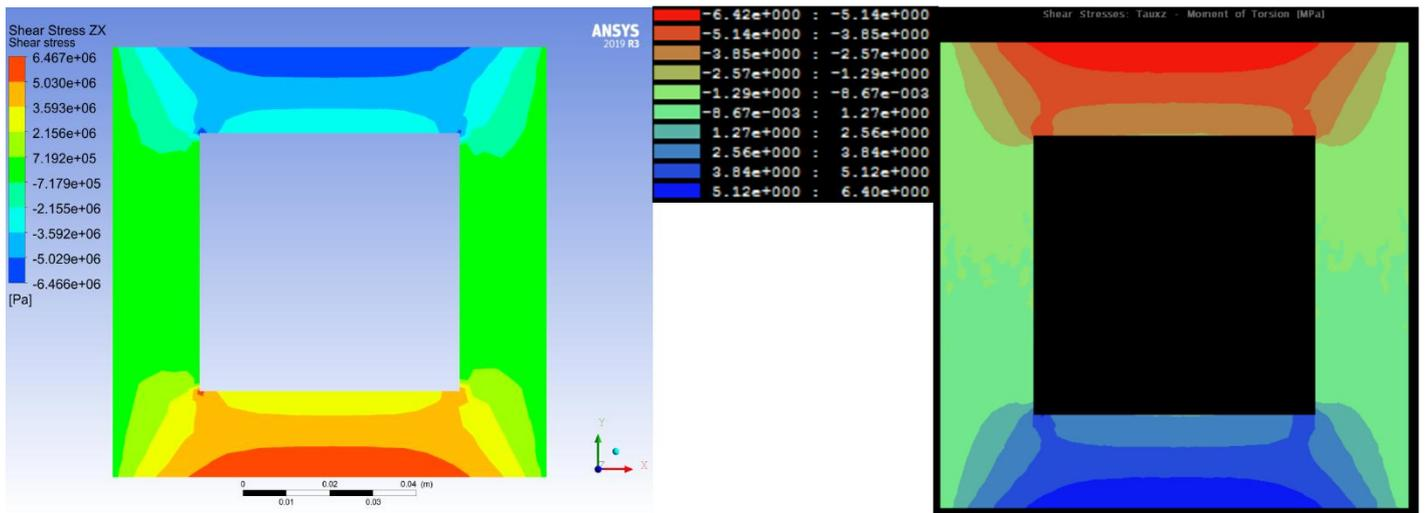
Figure 47 The contour plots of the shear stresses in the XZ plane. Left; Results from Ansys. Right; Results from ShapeDesigner
