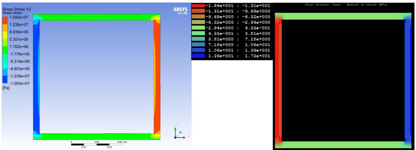
Figure 37 The contour plots of the shear stresses in the YZ plane. Left; Results from Ansys. Right; Results from ShapeDesigner
