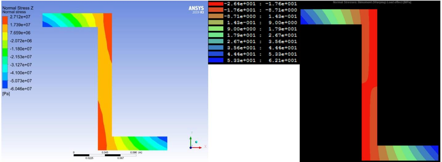
Figure 29 The contour plots of the normal stresses in Z-direction. Left; Results from Ansys. Right; Results from ShapeDesigner
