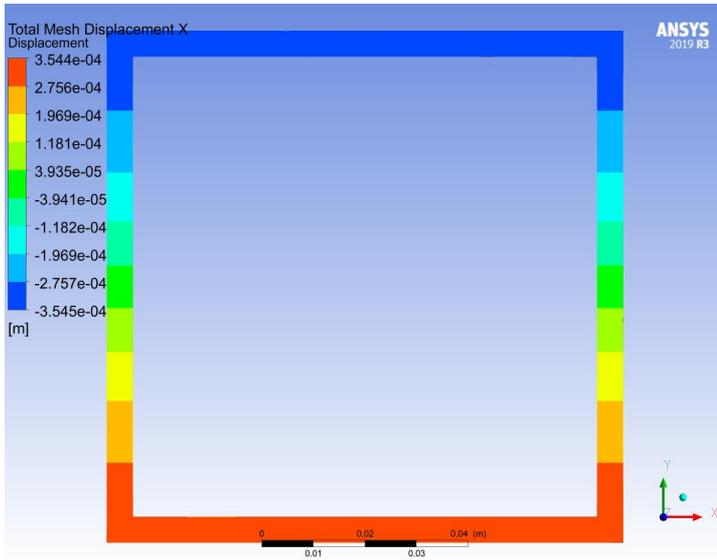
Figure 39 The horizontal displacement of beam 6 from Ansys
