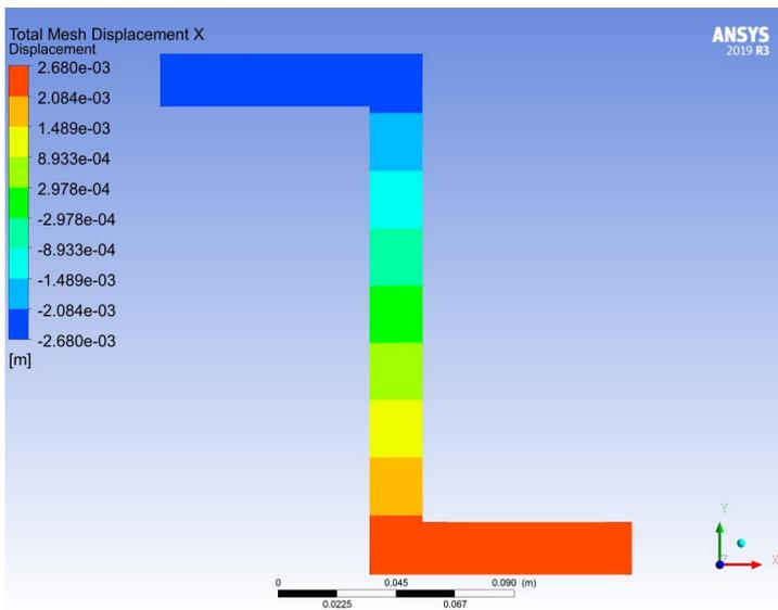
Figure 28 The horizontal displacement of beam 4 from Ansys
