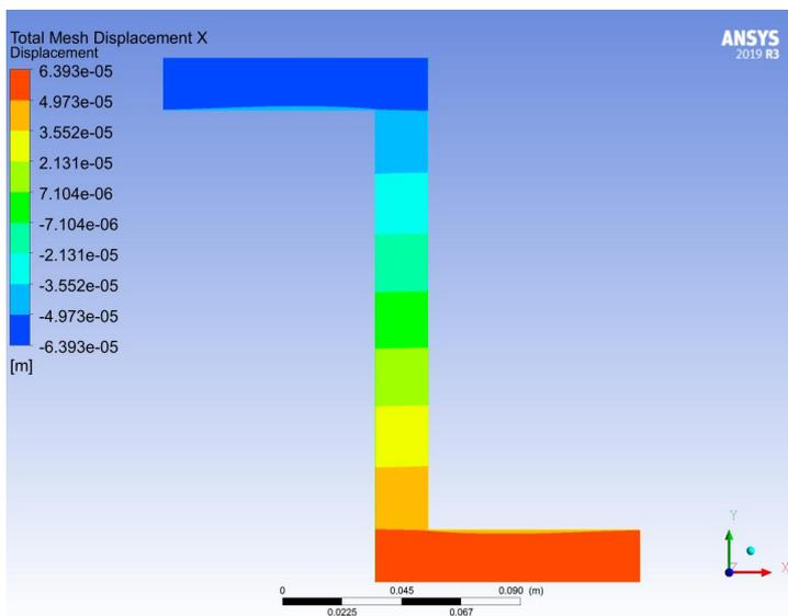
Figure 22 The horizontal displacement of beam 3 from Ansys
