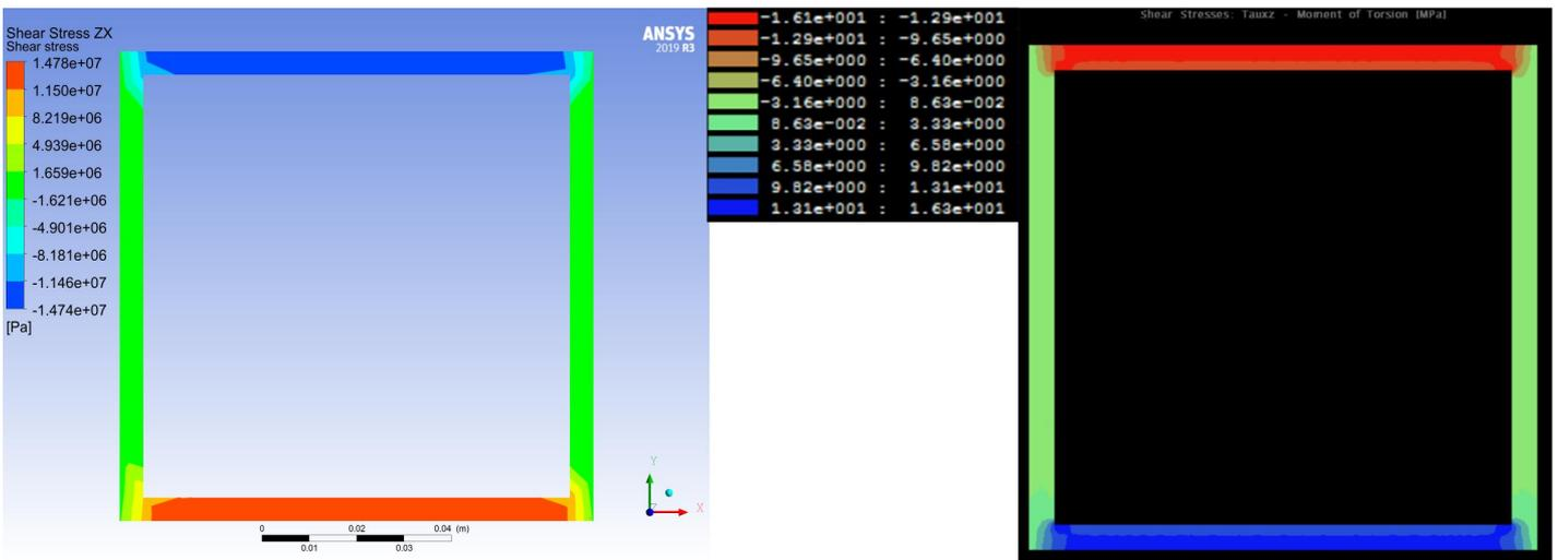
Figure 42 The contour plots of the shear stresses in the XZ plane. Left; Results from Ansys. Right; Results from ShapeDesigner
