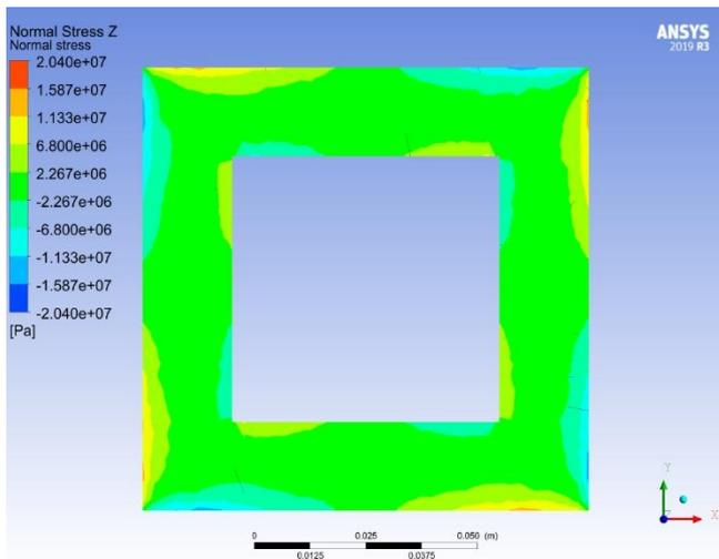
Figure 52 The normal stress in Z-direction at the fixed end with a rescaled legend
