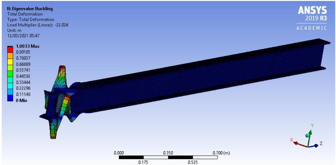
**Figure C1** The linear buckling (Eigenvalue buckling) of the test beam undergoing a torsional load. The deformations are displayed with a 0.17 factor.
