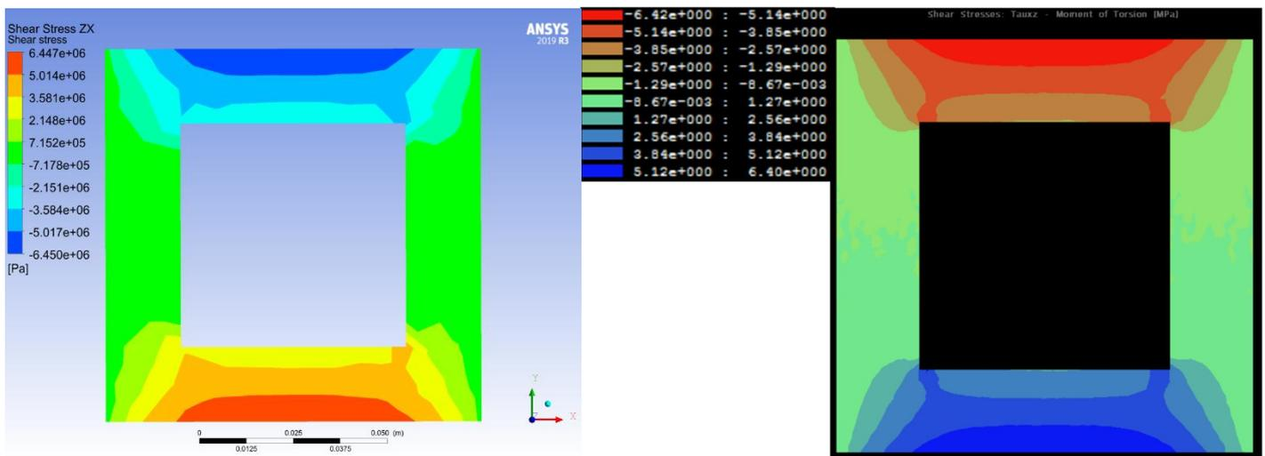
Figure 53 The contour plots of the shear stresses in the XZ plane. Left; Results from Ansys. Right; Results from ShapeDesigner
