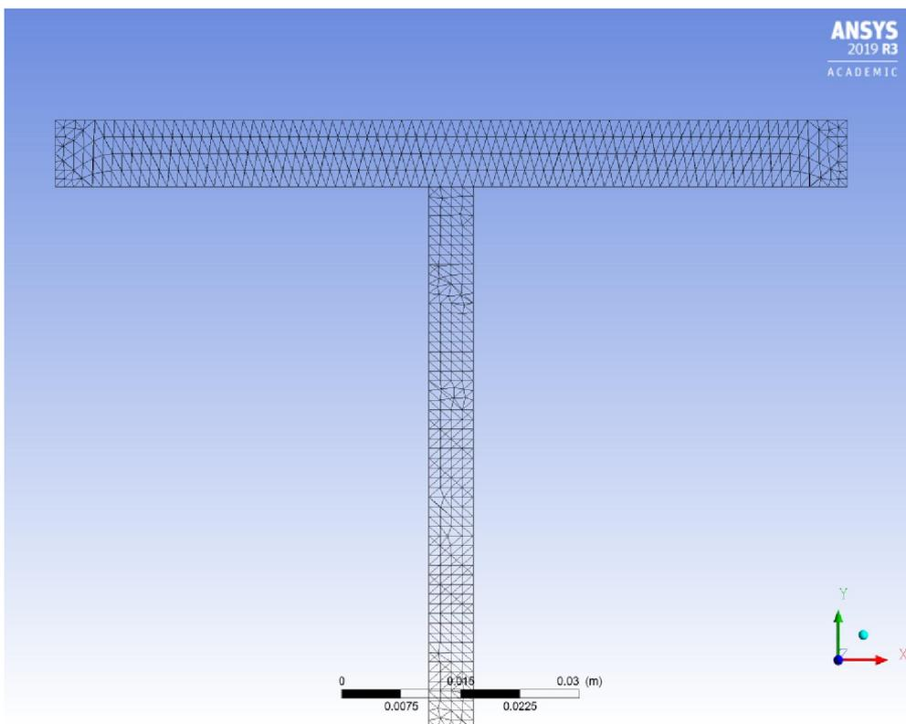
Figure 4 The mesh over the thickness of the flanges and the web on the free end
