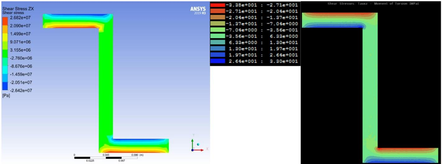
Figure 31 The contour plots of the shear stresses in the XZ plane. Left; Results from Ansys. Right; Results from ShapeDesigner
