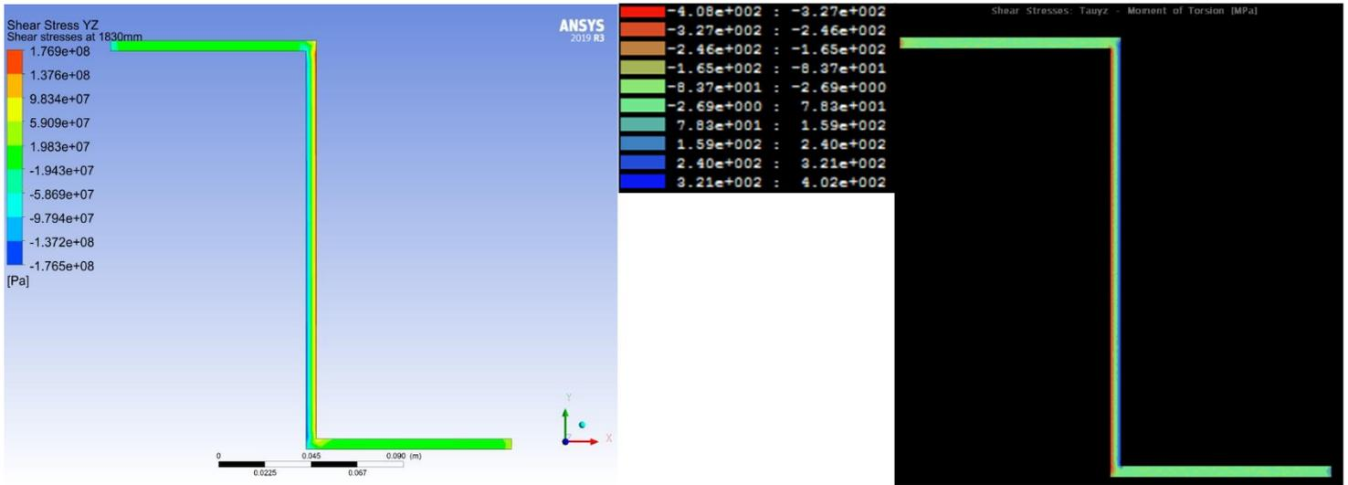
Figure 21 The contour plots of the shear stresses in the YZ plane. Left; Results from Ansys. Right; Results from ShapeDesigner
