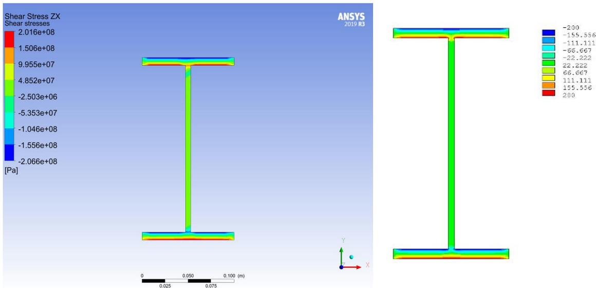
**Figure 6** Contour plots for the shear stress in XZ-plane. Left; Contour plot from this study. Right; Contour plot from Dr. Hoogenboom's reader
