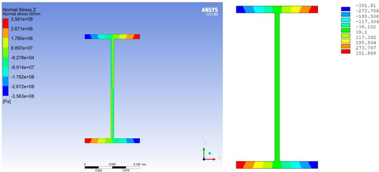
**Figure 8** The contour plots of the normal stresses in Z-direction. Left; Contour plots from this study. Right; Contour plots from Dr. Hoogenboom's reader
