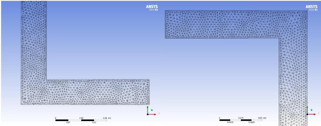
Figure B3 Meshing of beam 3. Left; Bottom flange. Right; Top flange
