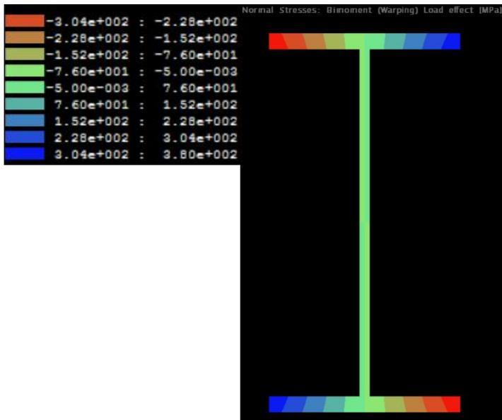
Figure 10 The contour plot for the normal stress from ShapeDesigner
