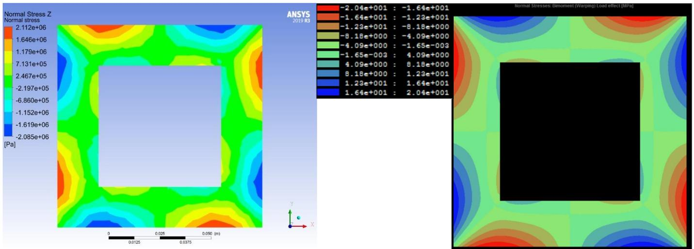
Figure 51 The contour plots of the normal stresses in Z-direction. Left; Results from Ansys. Right; Results from ShapeDesigner
