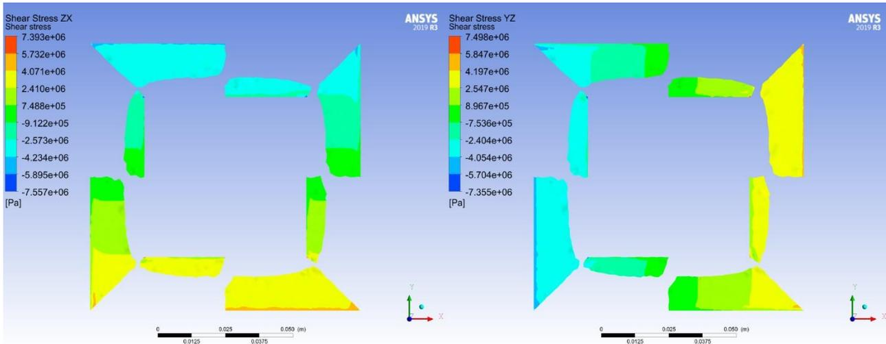
Figure 49 The shear stresses at the free end. Left; XZ plane. Right; YZ plane.
