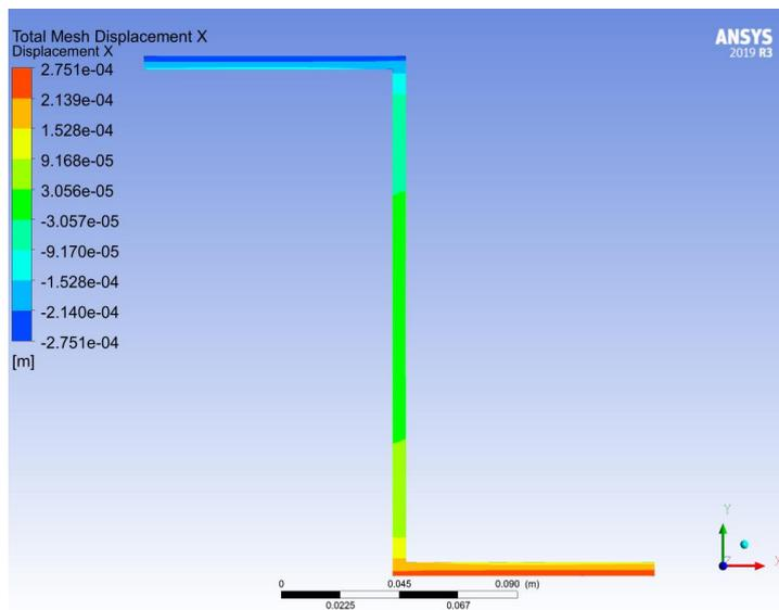
**Figure 11 The horizontal displacement of beam 1 from Ansys**
