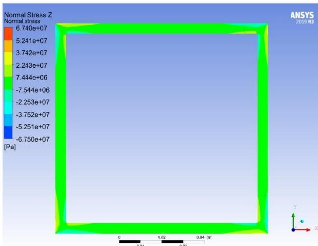
Figure 35 The normal stress in Z-direction at the fixed end with a rescaled legend
