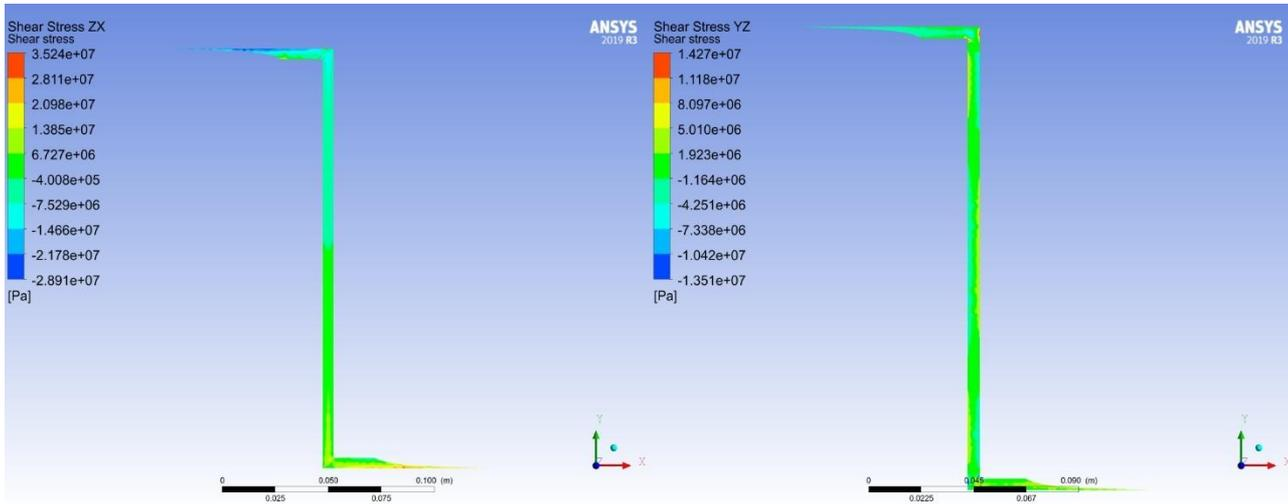
Figure 16 The shear stresses at the free end. Left; XZ plane. Right; YZ plane.
