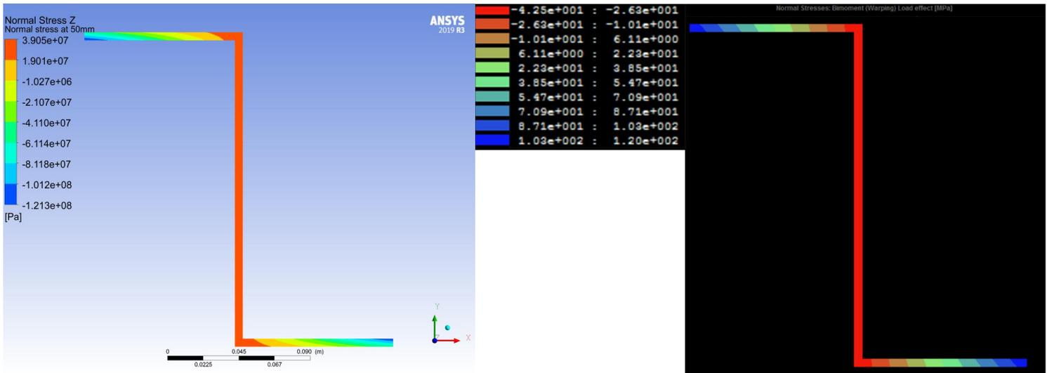
Figure 12 The contour plots of the normal stresses in Z-direction. Left; Results from Ansys. Right; Results from ShapeDesigner
