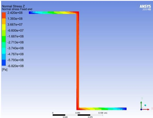
Figure 19 The normal stress in Z-direction at the fixed end with a rescaled legend
