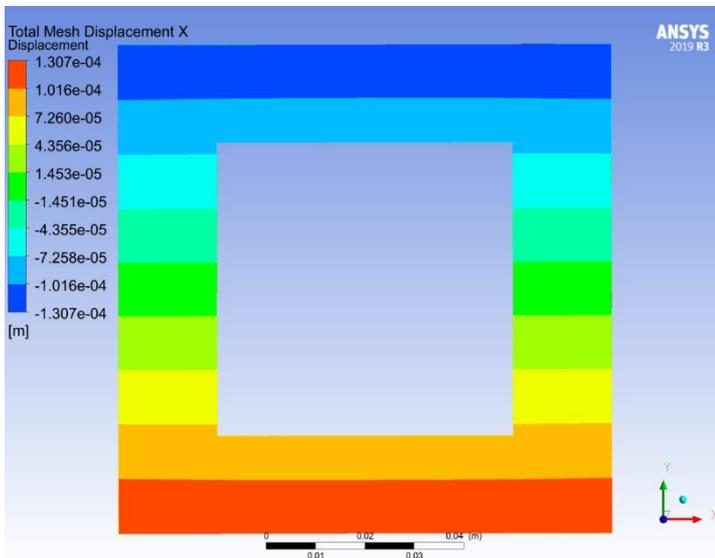
Figure 50 The horizontal displacement of beam 8 from Ansys
