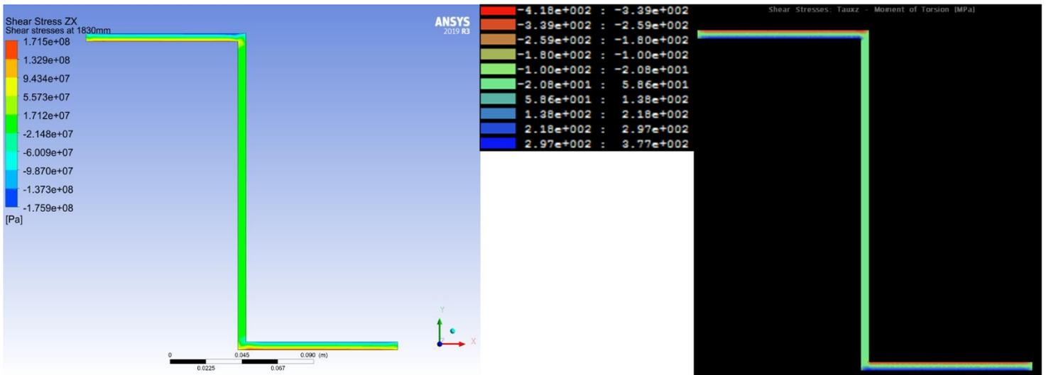
Figure 20 The contour plots of the shear stresses in the XZ plane. Left; Results from Ansys. Right; Results from ShapeDesigner
