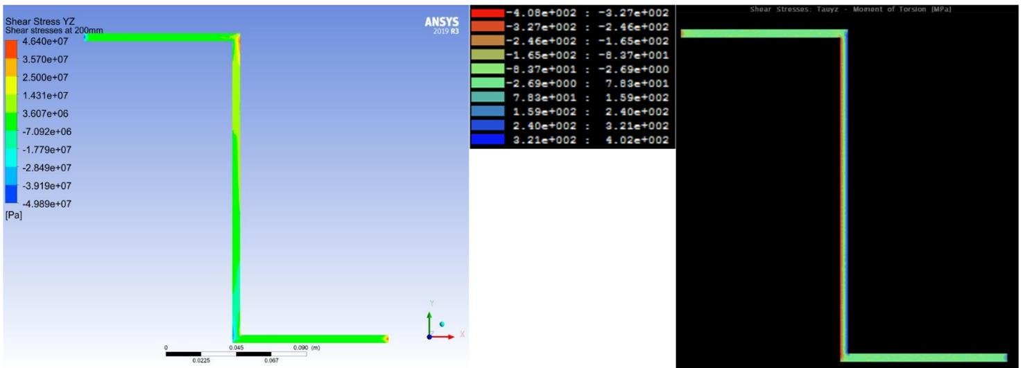
Figure 15 The contour plots of the shear stresses in the YZ plane. Left; Results from Ansys. Right; Results from ShapeDesigner
