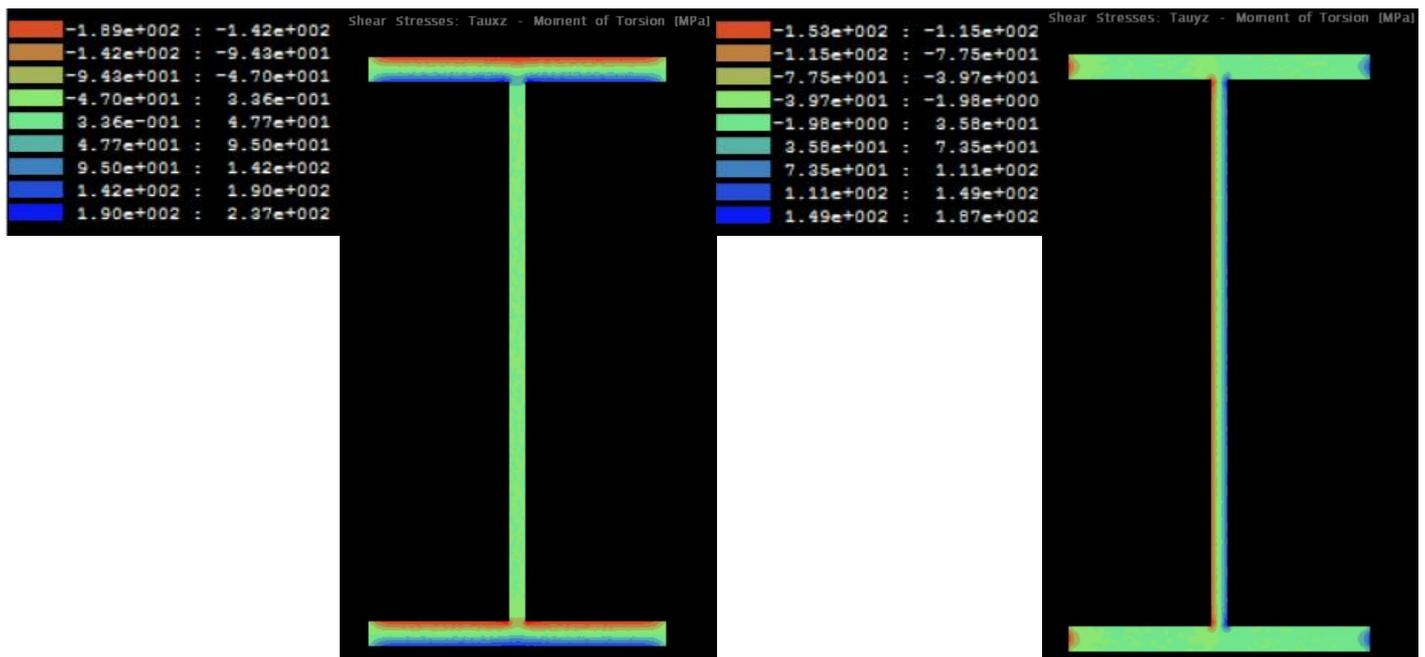
Figure 9 Left: The contour plot of the shear stress in XZ-plane. Right: The contour plot of the shear stress in YZ-plane
