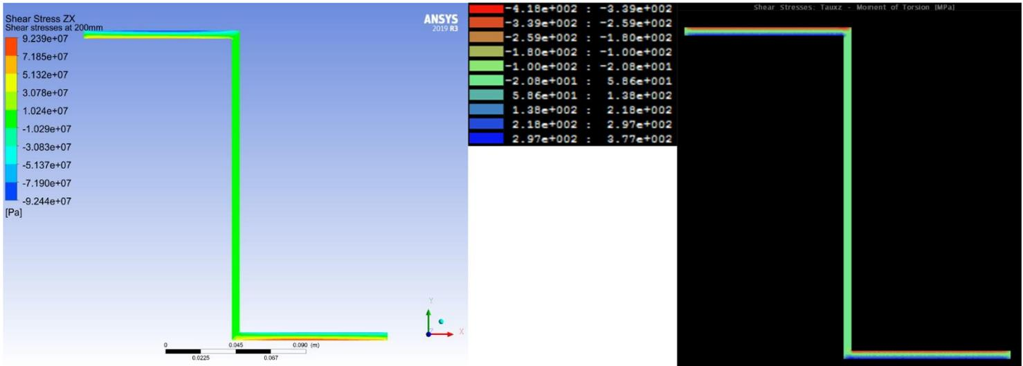
Figure 14 The contour plots of the shear stresses in the XZ plane. Left; Results from Ansys. Right; Results from ShapeDesigner
