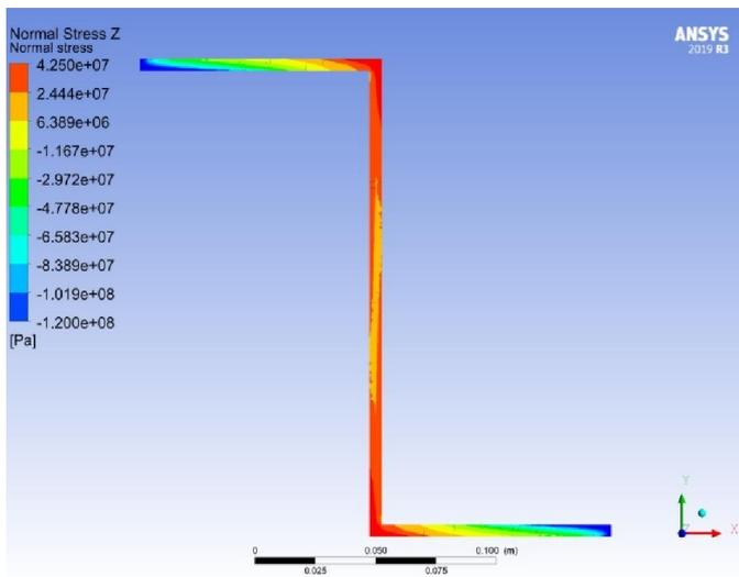
Figure 13 The normal stress in Z-direction at the fixed end with a rescaled legend
