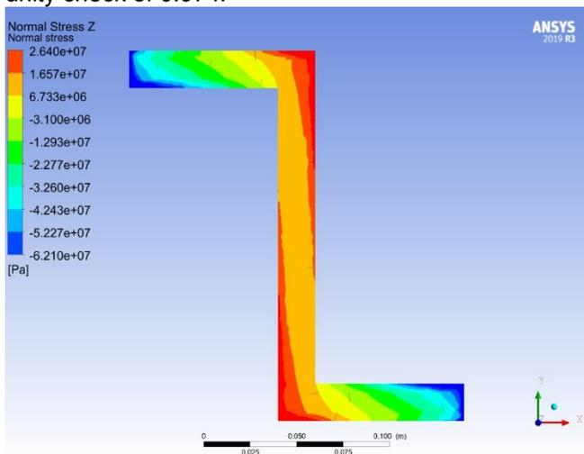
Figure 30 The normal stress in Z-direction at the fixed end with a rescaled legend
