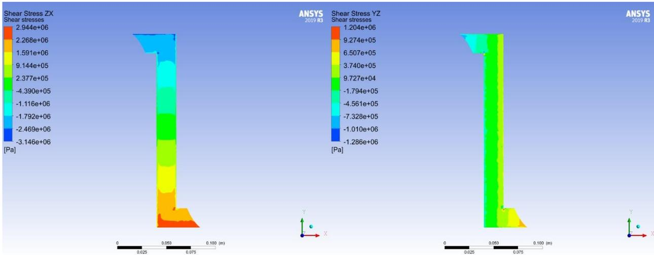
Figure 27 The shear stresses at the free end. Left; XZ plane. Right; YZ plane.
