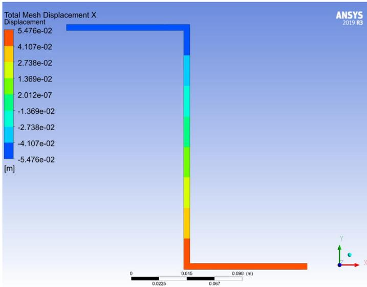
Figure 17 The horizontal displacement of beam 2 from Ansys
