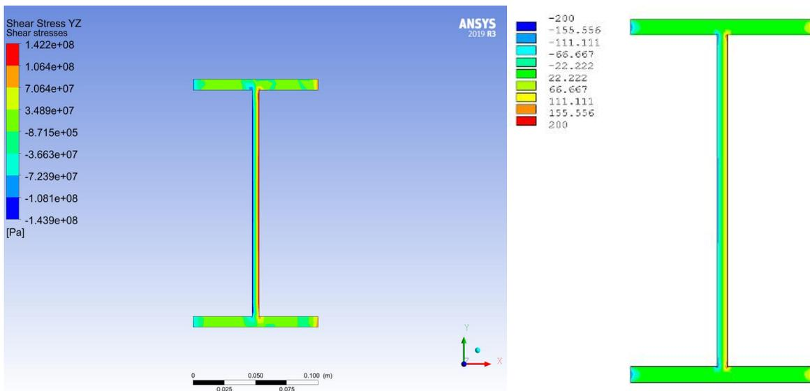
**Figure 7** Contour plots for the shear stress in YZ-plane. Left; Contour plot from this study. Right; Contour plot from Dr. Hoogenboom's reader
