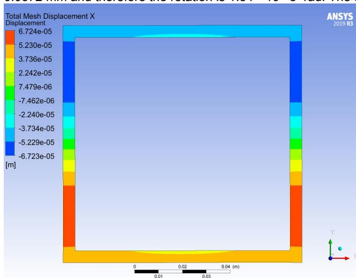
**Figure 33 The horizontal displacement of beam 5 from Ansys**
