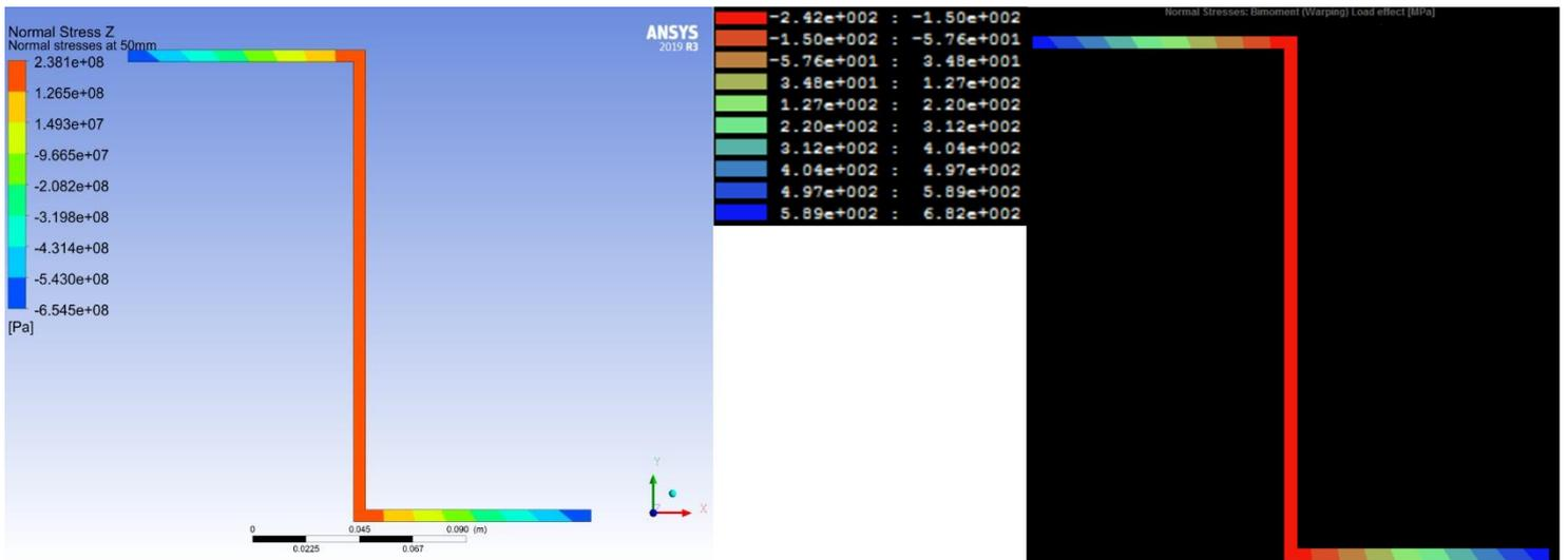
Figure 18 The contour plots of the normal stresses in Z-direction. Left; Results from Ansys. Right; Results from ShapeDesigner
