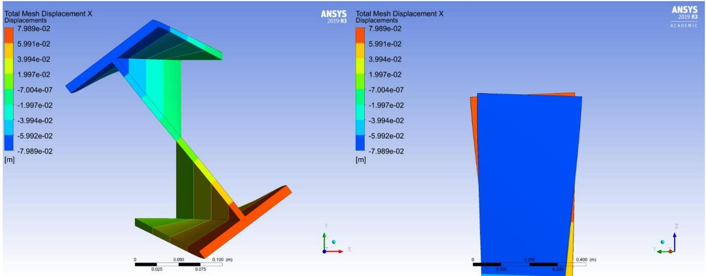
**Figure 5** The contour plot of the horizontal displacement view with true scale. Left; view on z-axis. Right; The warping of the flanges on the free end
