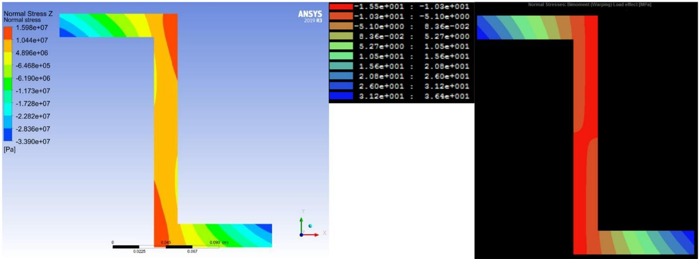
**Figure 23** The contour plots of the normal stresses in Z-direction. Left; Results from Ansys. Right; Results from ShapeDesigner
