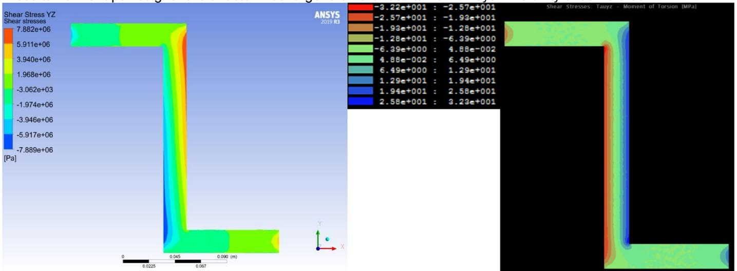
Figure 26 The contour plots of the shear stresses in the YZ plane. Left; Results from Ansys. Right; Results from ShapeDesigner
