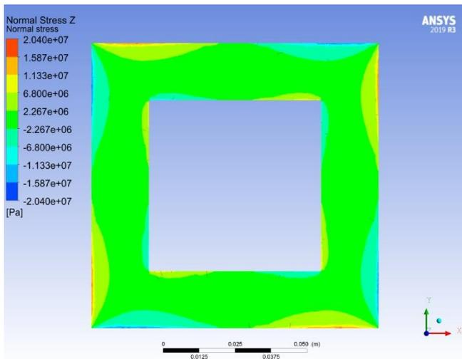
Figure 46 The normal stress in Z-direction at the fixed end with a rescaled legend
