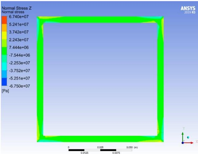
Figure 41 The normal stress in Z-direction at the fixed end with a rescaled legend
