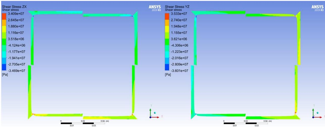
Figure 38 The shear stresses at the free end. Left; XZ plane. Right; YZ plane.
