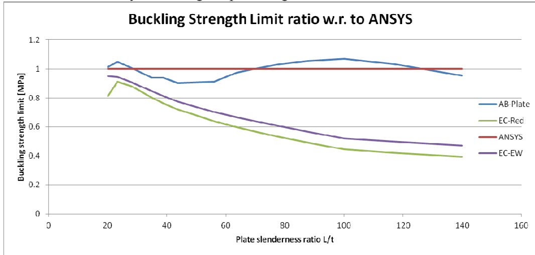
Figure 3.21 Normalized buckling strength limit with respect to ANSYS results
