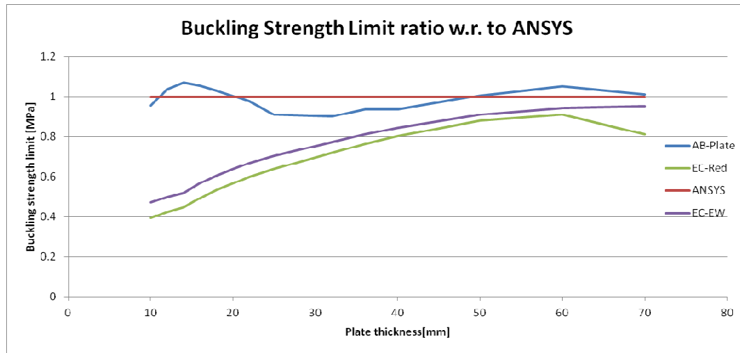
Figure 3.19 Buckling Strength Limit relative to ANSYS results
