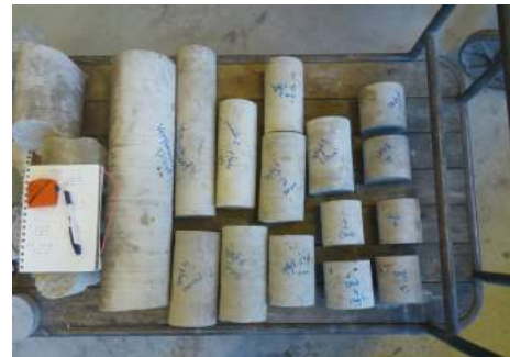
(b) Sawn drilled cores provided
