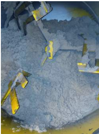
Figure III.2: Mixing step 2: saturating sands (replicating soil)
