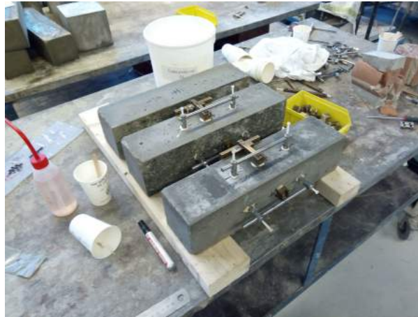
Figure V.7: Attaching the LVDT's
