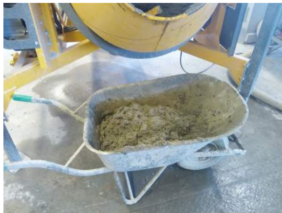
Figure III.3: Mixing step 3: adding cement and water
