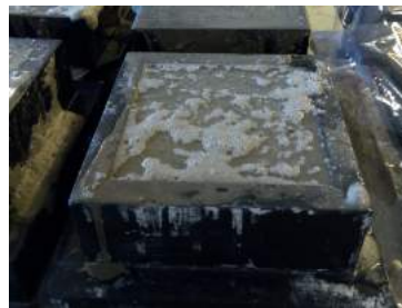
Figure III.11: Bleeding of a specimen after casting
