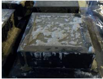
Figure 3.6: Bleeding of a specimen after casting
