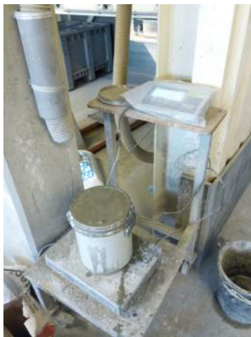
Figure III.7: Measuring of the density
