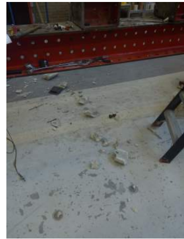
(c) Sample 1, explosive failure
