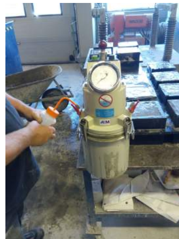
Figure III.8: Measuring of the air content
