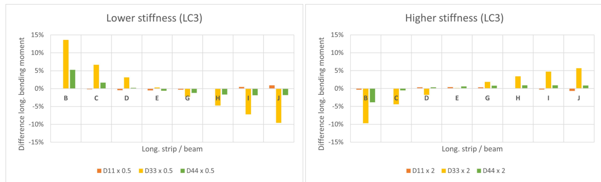
Figure 7.17: Difference longitudinal bending moment for lower/higher stiffnesses, LC3
