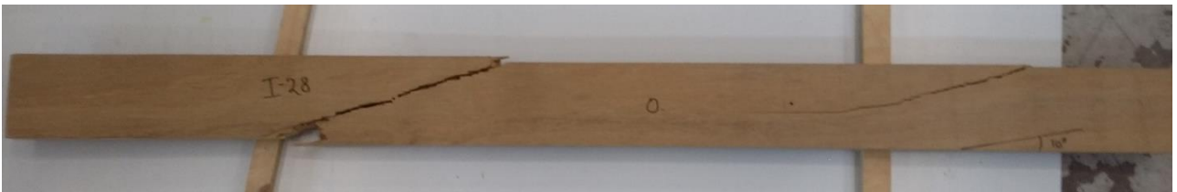
Figure 140: Failure of specimen I-28 (flipside).
