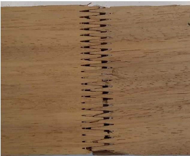
Figure 167: Failure of specimen II-7.
