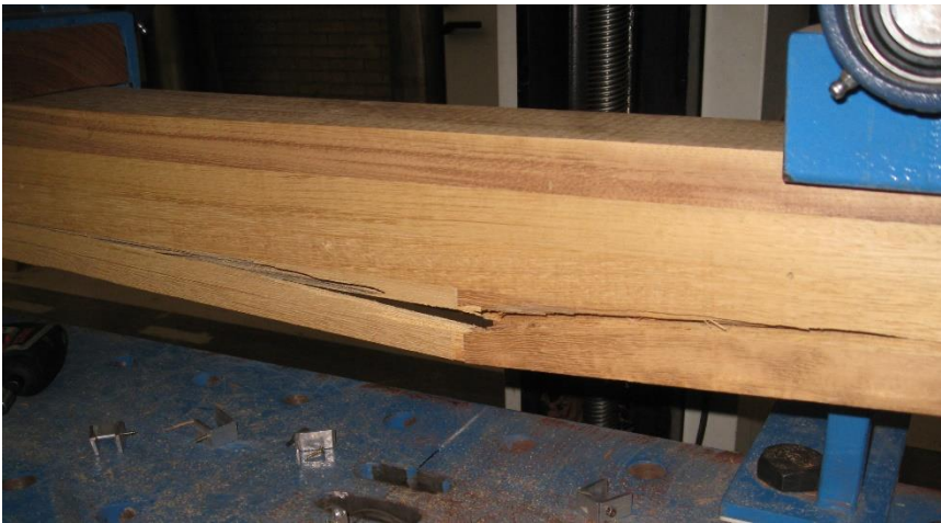
Figure 214: Failure of specimen IV-8 (crack detail).
