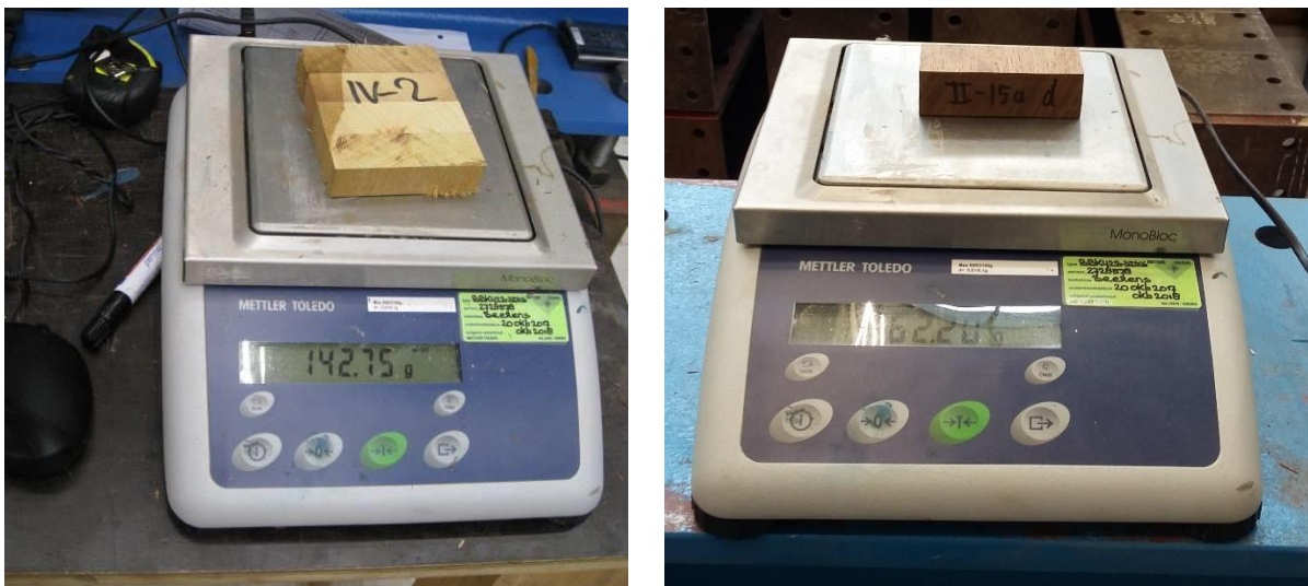
Figure 52: Small balance; weighing of the test slices.
