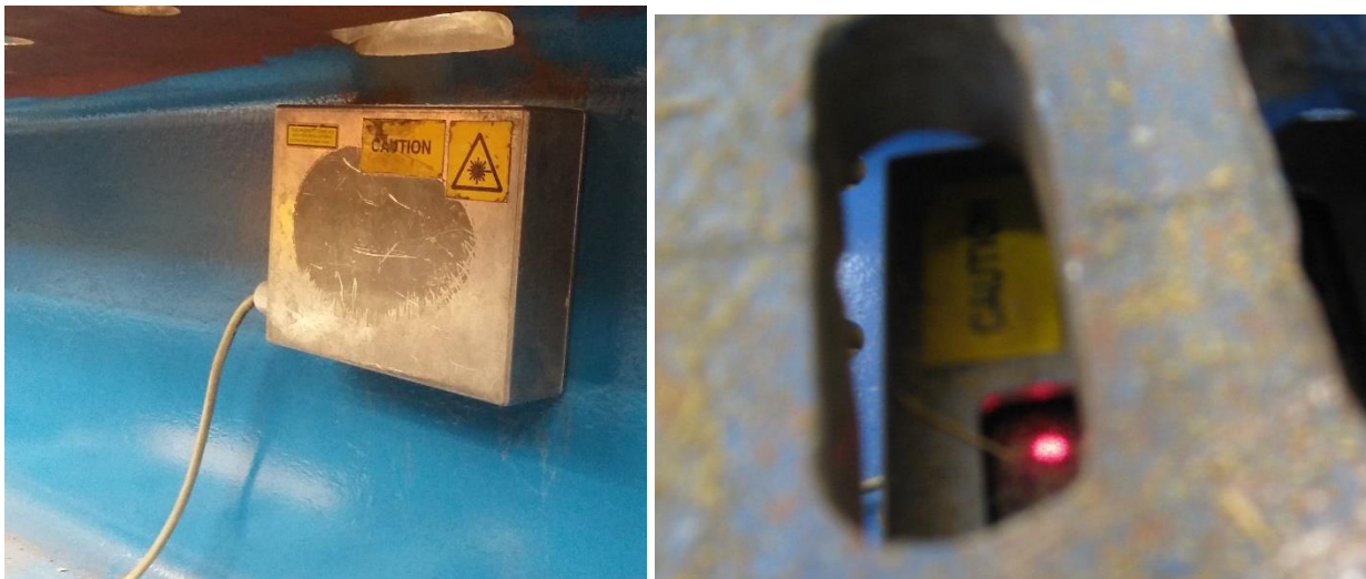
Figure 63: Lasers as to determine the global displacements.
