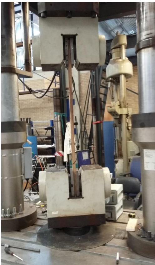
Figure 56: Lamella clamped in tension testing machine.
