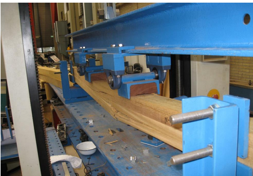
Figure 207: Failure of specimen IV-5.
