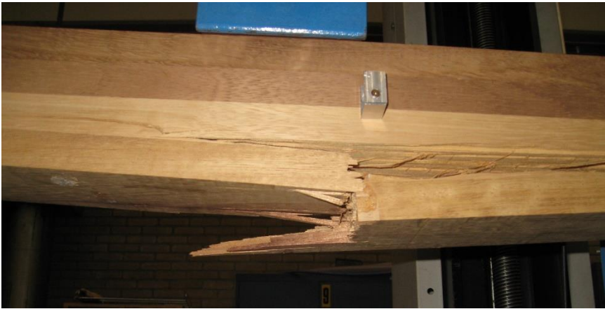
Figure 202: Failure of specimen IV-2 (crack detail).
