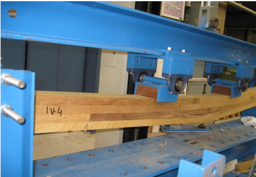
Figure 205: Failure of specimen IV-4.
