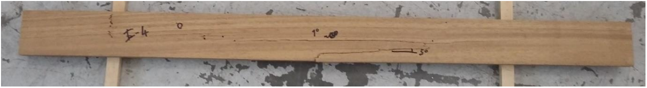
Figure 94: Failure of specimen I-4 (flip side).
