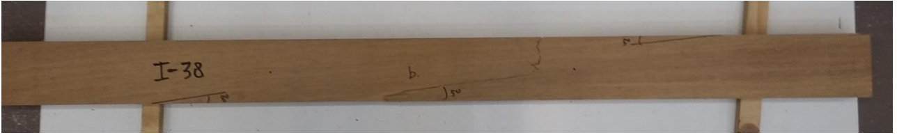
Figure 159: Failure of specimen I-38 (front side).
