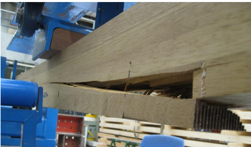
Figure 222: Failure of specimen IV-12 (crack detail).
