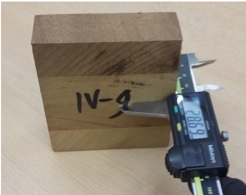
Figure 53: Measuring the thickness of a test slice with the vernier caliper.
