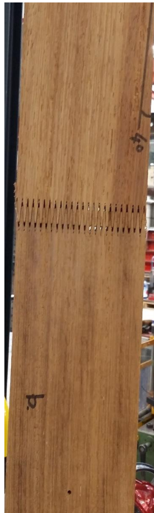
Figure 68: Glue failure (II-31).
