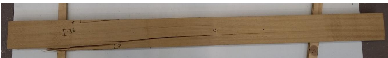
Figure 156: Failure of specimen I-36 (flipside).
