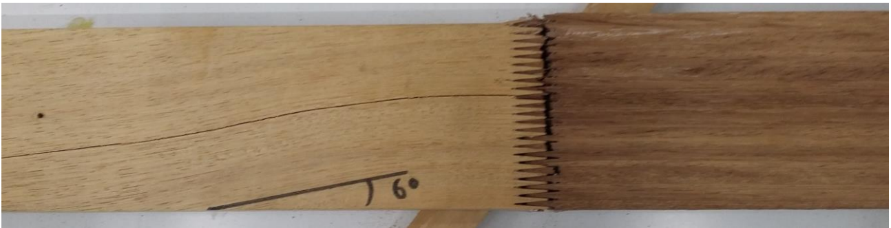
Figure 186: Failure of specimen II-26.
