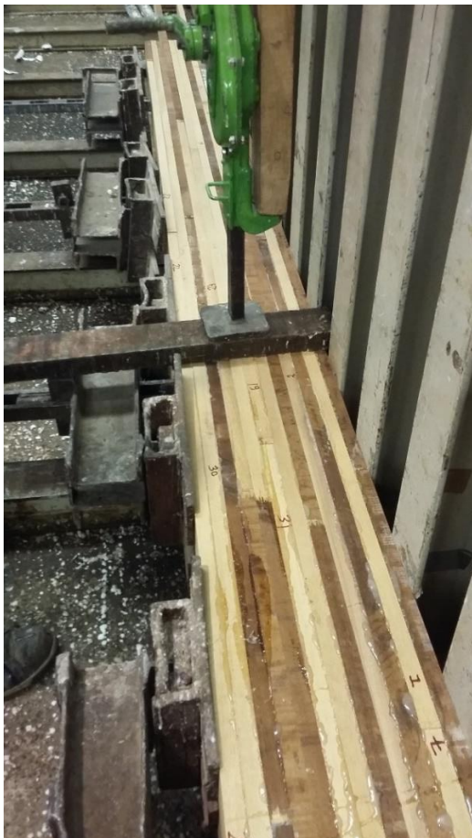
Figure 39: Pressing of the boards (a).
