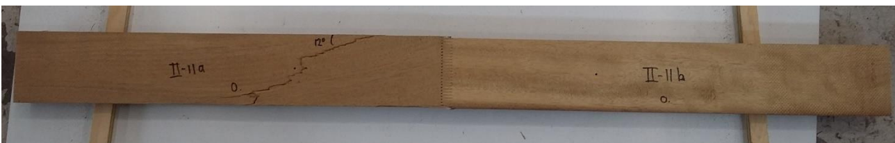
Figure 171: Failure of specimen II-11.
