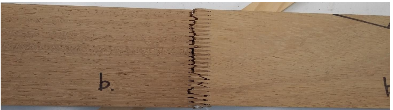
Figure 193: Failure of specimen II-33.
