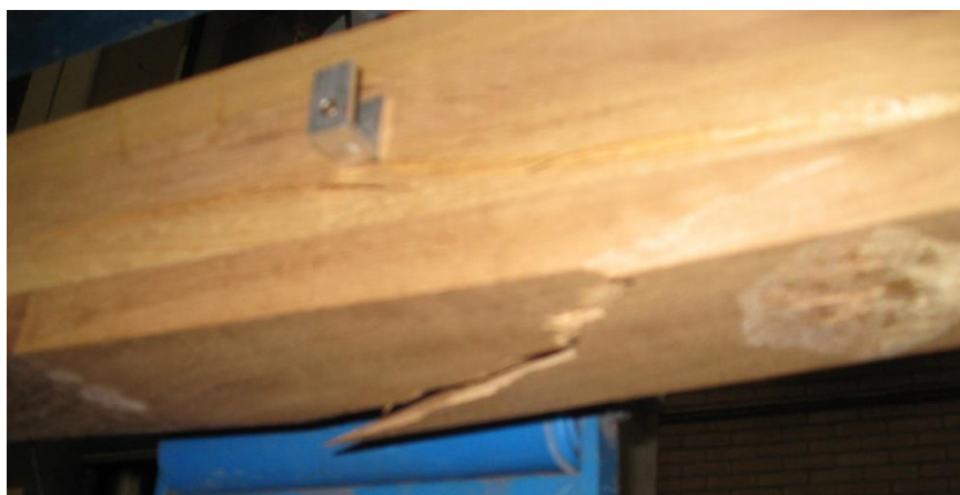
Figure 200: Failure of specimen IV-1 (crack detail).
