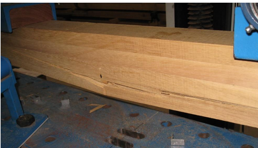
Figure 210: Failure of specimen IV-6 (crack detail).
