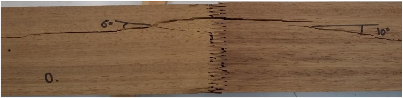
Figure 71: Failure of both wood and finger joint (II-29).
