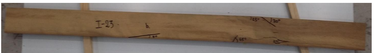
Figure 129: Failure of specimen I-23 (front side).
