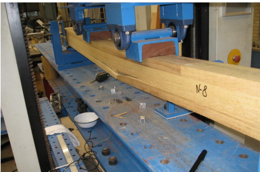
Figure 213: Failure of specimen IV-8.
