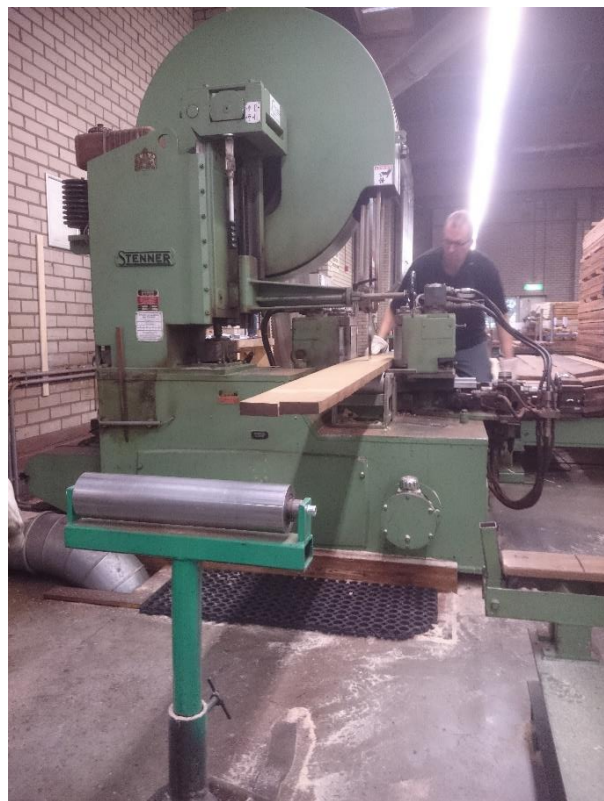
Figure 31: Cutting the planks in half.
