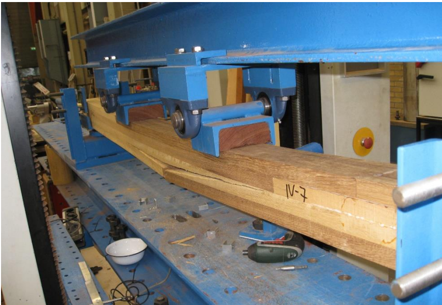
Figure 211: Failure of specimen IV-7.
