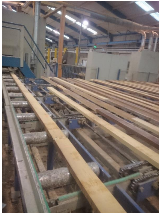
Figure 35: 24 finger jointed lamellas.
