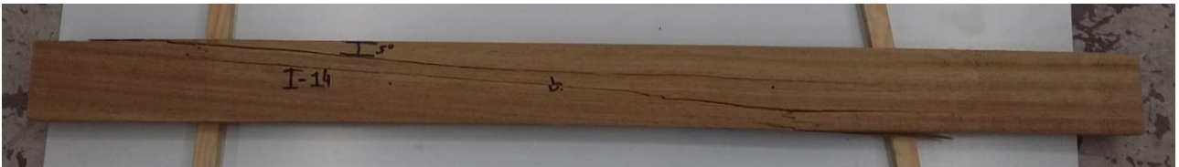
Figure 111: Failure of specimen I-14 (front side).
