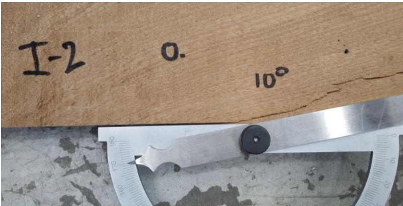
Figure 58: Measuring the angle at which failure occurred.
