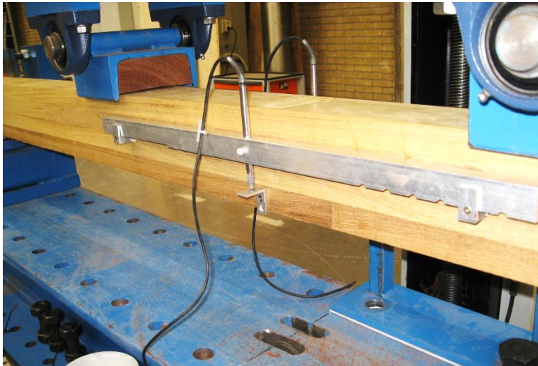
Figure 62: LVDT's placed in braces upon the test beam.
