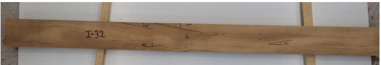
Figure 147: Failure of specimen I-32 (front side).
