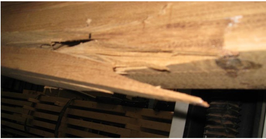
Figure 208: Failure of specimen IV-5 (crack detail).
