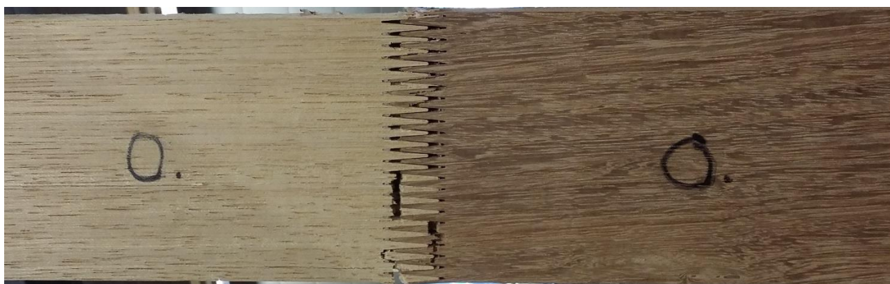
Figure 162: Failure of specimen II-2.
