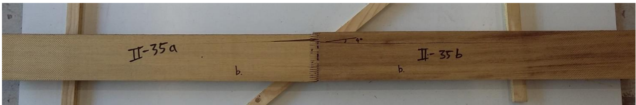
Figure 195: Failure of specimen II-35.
