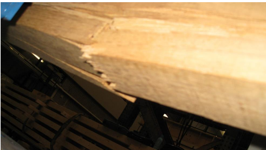
Figure 204: Failure of specimen IV-3 (crack detail).
