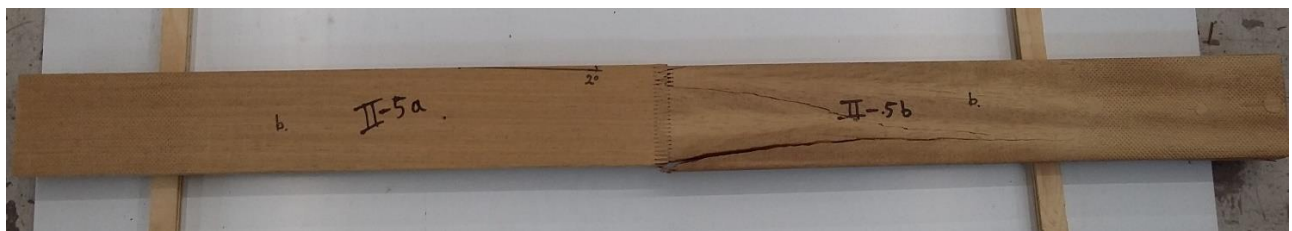
Figure 165: Failure of specimen II-5.
