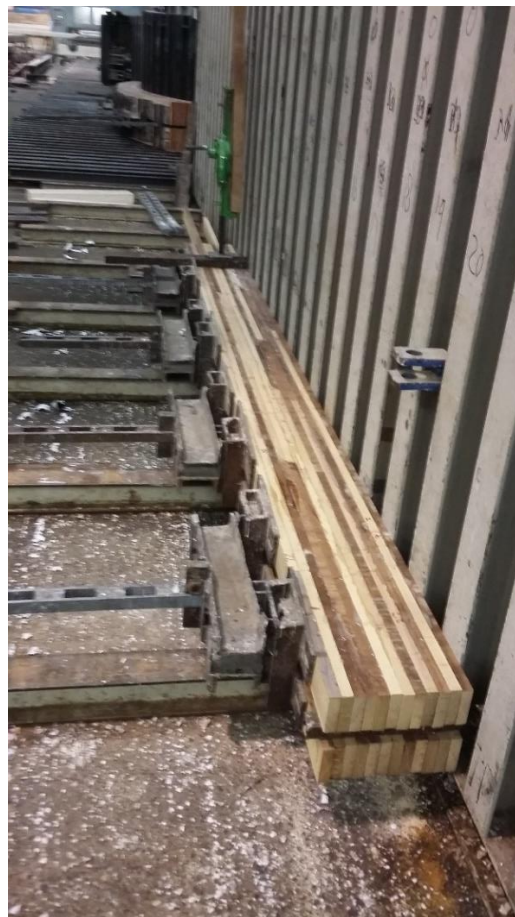
Figure 40: Pressing of the boards (b).
