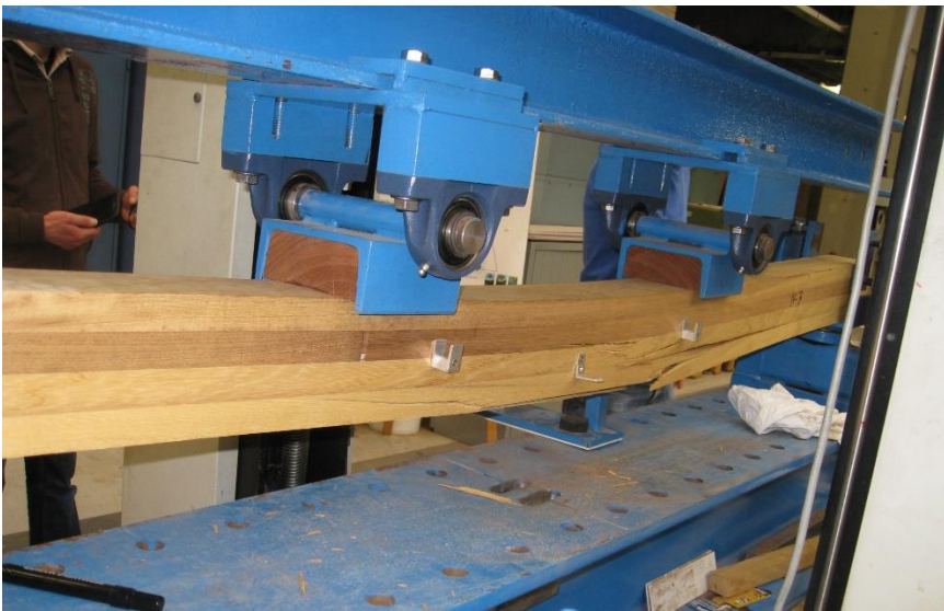
Figure 203: Failure of specimen IV-3.
