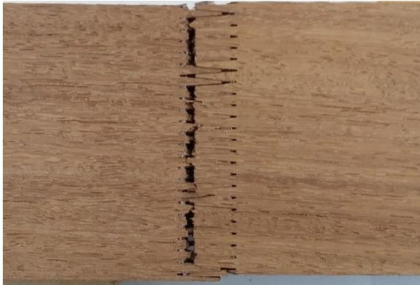
Figure 173: Failure of specimen II-13.
