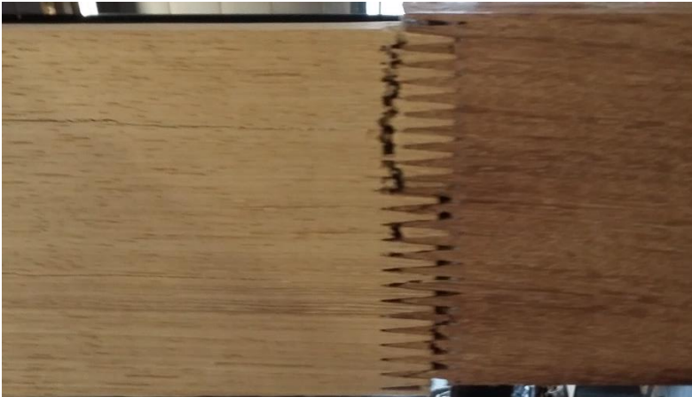
Figure 169: Failure of specimen II-9.
