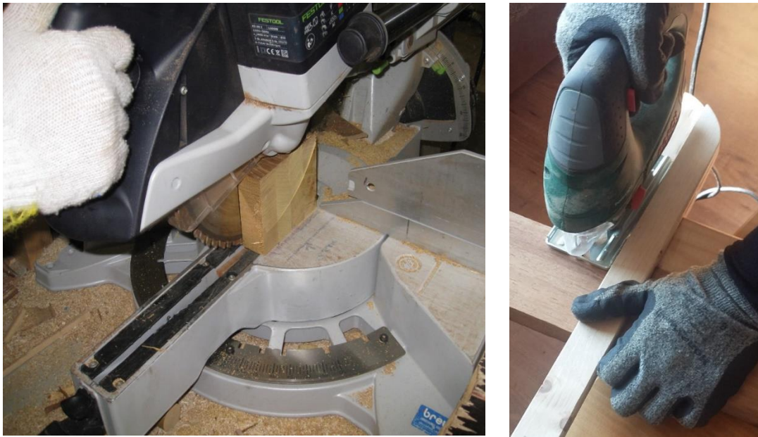
Figure 51: Cutting of the test slices from the specimens.
