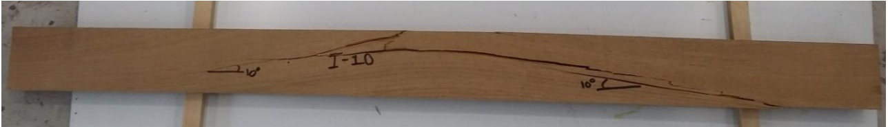
Figure 103: Failure of specimen I-10 (front side).
