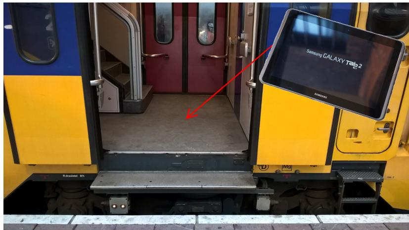
**Figure 4.3:** Photo of experimental setup, location of measuring device on vestibule floor of train.
