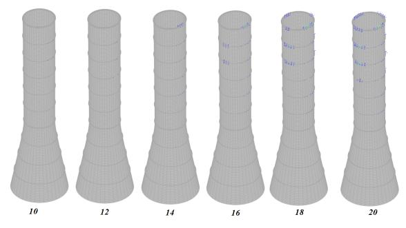
Figure 8.15: The crack initiation of 1% Recentered Nonlinear Model from load step 10 to 20.
