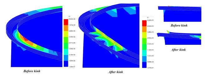
Figure 8.26: The principal strain distribution of top ring for 1% Recentered Nonlinear Model
