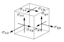
Figure C.1: Cauchy stress on a unit cube in their positive direction (DIANA (2016))
