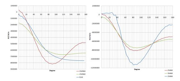
Figure D.8: The comparison of meridional stress distribution at the windward direction at the thorat height over the circumference for 1%RNM, 2%RNM, DLM; the comparison of meridional stress distribution at the windward direction at the thorat height over the circumference for 2%NM, 3%NM, 1%NM
