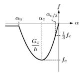
Figure A.2: Parabolic curve for concrete in compression (DIANA (2016))
