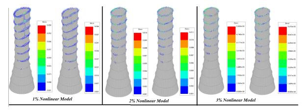
Figure 8.8: The crack strain distribution exceeds the allowable value of the model 1% Nonlinear Model; 2% Nonlinear Model; 3% Nonlinear Model
