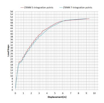
Figure 7.2: Load steps-displacement curve for 1%NM integration scheme of 5-points Simpson and 7-points Simpson in thickness direction
