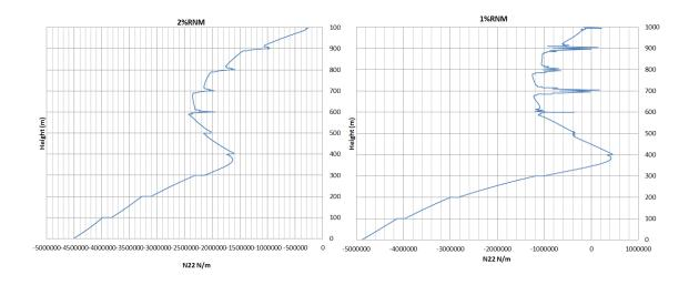
Figure D.5: The meridional stress distribution at the winward direction for 2%RNM,1%RNM
