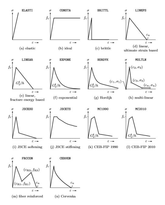
Figure A.5: Stress-strain relation of different concrete cracking model (DIANA (2016))
