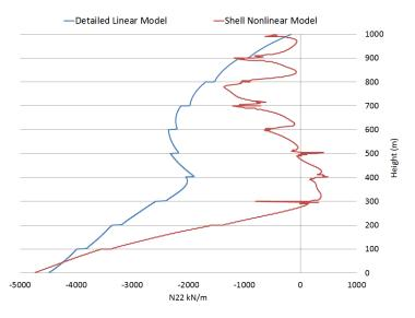
Figure 7.19: N22 stress resultant distribution over height for Shell Nonlinear Model and Detailed Linear Model at 1D+1W
