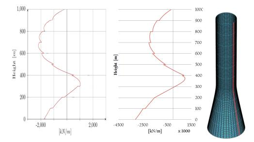
Figure 5.4: Comparison of in-plane meridional stress resultant distribution over height between literature Eck et al. (2015)(left) and Simple Linear Model(middle), the location that stress resultant distribution is calculated (right)
