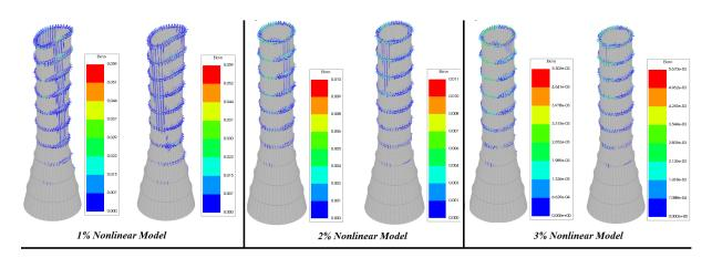
Figure 8.7: The crack strain distribution of the model 1% Nonlinear Model; 2% Nonlinear Model; 3% Nonlinear Model
