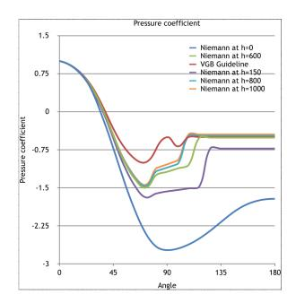
Figure A.7: Pressure coefficient over circumference of solar updraft tower
