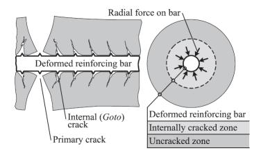
Figure 6.2: The formation of secondary crack (Goto.Y. (1971))
