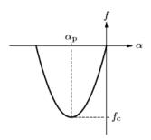
Figure A.3: Hognestad stress-strain relation for concrete in compression (DIANA (2016))
