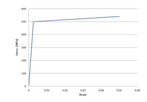
Figure 6.8: Stress-strain relation for reinforcement bar
