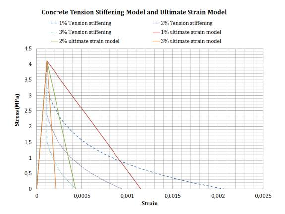
Figure A.6: The tension stiffening model and the linear ultimate strain model used in the FEM
