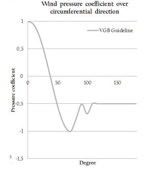
Figure 3.7: Pressure coefficient in the circumferential direction
