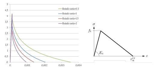
Figure 6.4: The tension stiffening curve with varying reinforcement ratios(left) Stress-strain relationship of concrete in tension(right)
