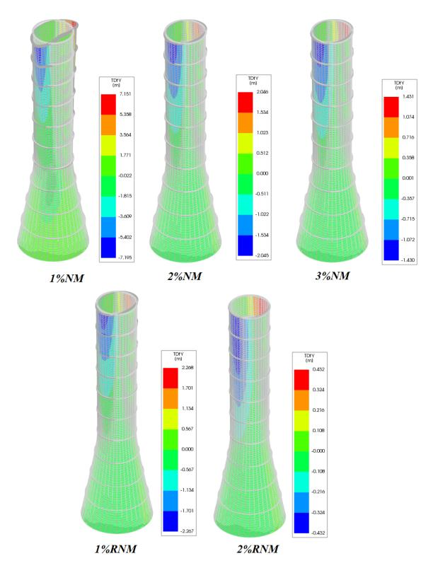
Figure D.1: Displacement in y direction for models 1%NM, 2%NM, 3%NM, 2%RNM,1%RNM
