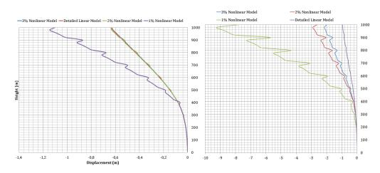
Figure 8.6: the global displacement in the windward direction over height (1D+1W) for model 1% Nonlinear Model, 2%Nonlinear Model, 3%Nonlinear Model (left),The local displacement in the windward direction over height (1D+1W) for model 1% Nonlinear Model, 2% Nonlinear Model, 3% Nonlinear Model(right)
