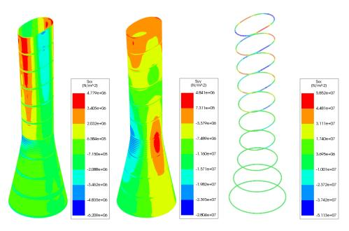
Figure 5.5: Cricumferential stress distribution on the shell walls (left) meridional stress distribution on the shell walls(middle) and circumferential stress distribution on the stiffening rings(right) for Simple Linear Model (1D+1.5W)
