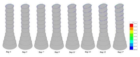
Figure 7.7: The crack distribution of SNM from load step 3 to 17
