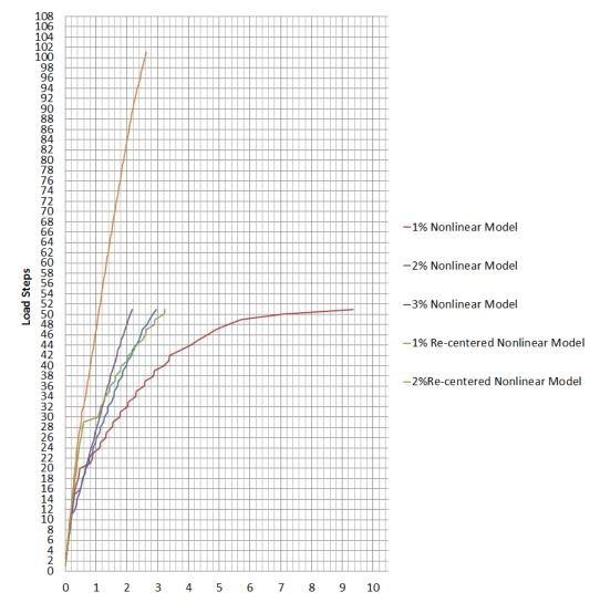
Figure E.1: Load steps-displacement curve for 1%NM, 2%NM, 3%NM 2%RNM, 1%RNM
