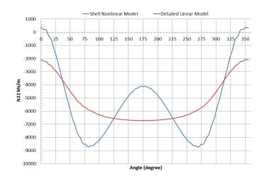
Figure 7.21: N22 in the circumferential direction at throat height for Shell nonlinear Model and Beam Nonlinear Model
