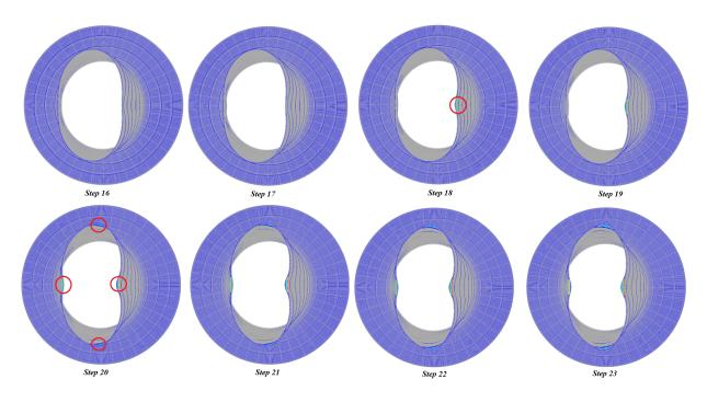
Figure 7.12: The deformation of Beam Nonlinear Model from load step 16 to 23 with normalized deformation
