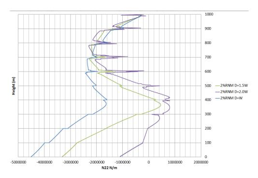
Figure E.6: The meridional stress resultant over height for model 2%RNM at D+W, D+1.5W and D+2W
