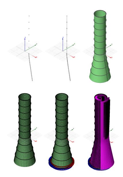
Figure 4.1: Procedures for building up the FEM,  $1^{st}$  Determine the compound points,  $2^{nd}$  Connect point by 3D lines,  $3^{rd}$  Revolution around central z axis,  $4^{th}$  Mesh the geometry,  $5^{th}$  Setting boundary conditions,  $6^{th}$  Adding loads.
