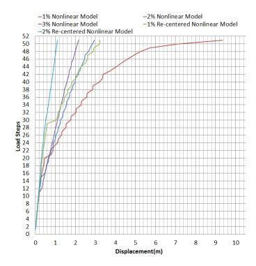
Figure 10.1: Load steps-deflection curve
