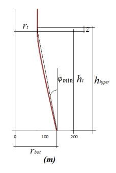
Figure 2.2: Minimum tilt angle of hyperbola at the base.
