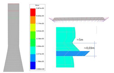
Figure 7.5: The crack strain distribution on the shell wall under self-weight(left); the crack distribution on the stiffening rings (right up); the deflected shape of stiffening rings under self-weight(right-down) (SNM)
