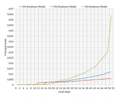
Figure 8.4: The maximum tensile principal strain development at inner shell layer for model 1% Nonlinear Model, 2% Nonlinear Model, 3% Nonlinear Model
