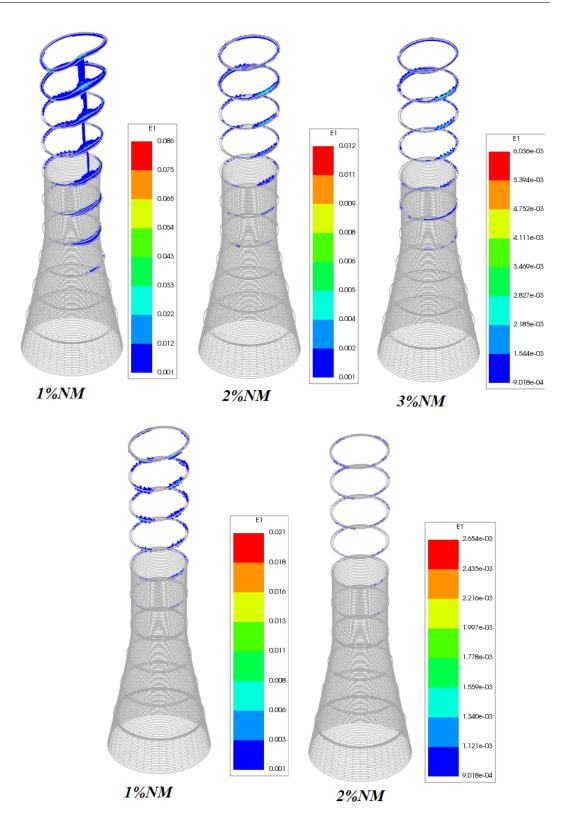
Figure D.3: The maximum pricipal strain distribution(0.0009018-max) for models 1%NM, 2%NM, 3%NM, 2%RNM,1%RNM
