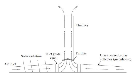
Figure 1.1: The solar updraft tower power plant schematic (Gannon (2002)).
