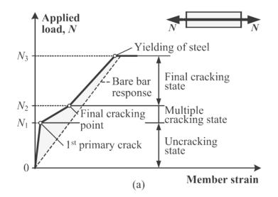
Figure 6.3: Stages of load-deformation behavior of a reinforced concrete tensile member (Goto.Y. (1971))
