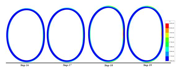
Figure 7.8: Principal strain distribution of the intermediate ring (900m) for SNM
