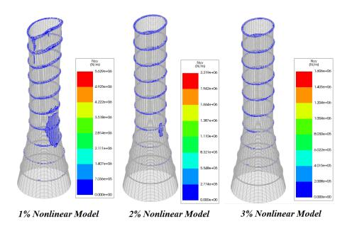
Figure 8.12: The tensile stress resultant in the meridional direction distribution 1% Nonlinear Model, 2% Nonlinear Model, 3% Nonlinear Model
