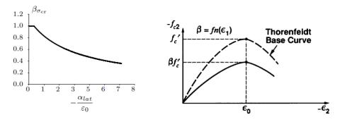
Figure 6.6: The reduction factor by lateral crack(left) The stress-strain compressive curve for concrete after the lateral crack is taken into account(right) (DIANA (2016))
