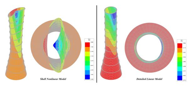
Figure 7.13: deformed shape for SNM and DLM with factor of 10 and the contour plot is the displacement in windward direction
