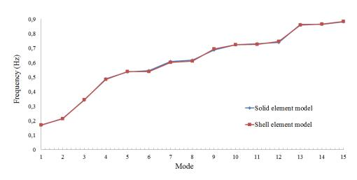
Figure 4.7: Natural frequencies of curved shell element model and 3D solid element model
