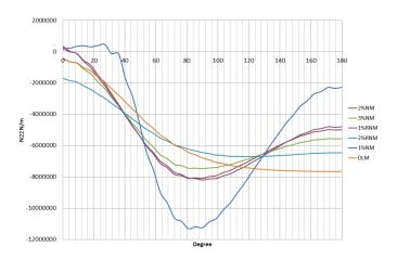
Figure D.9: The comparison of meridional stress distribution at the windward direction at the thorat height over the circumference for 2%NM, 3%NM, 1%NM, 1%RNM, 2%RNM, DLM
