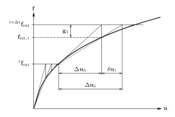
Figure 7.1: Modified Newton-Raphson iteration (DIANA (2016))
