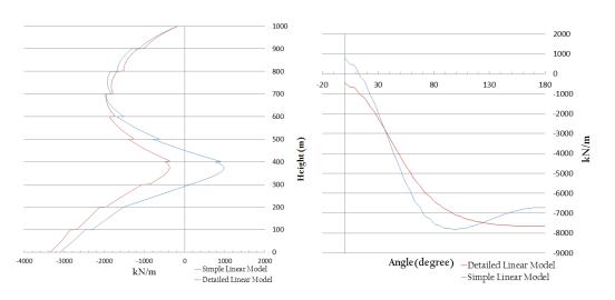
Figure 5.9: In-plane meridional stress resultant distribution over height of Simple Linear Model and Detailed Linear Model(left) and In-plane meridional stress resultant distribution at throat height over the circumference (right) (1D+1.5W)
