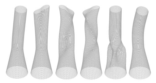
Figure 5.7: First 6 free vibration mode shapes for Detailed Linear Model  $(1^{st}(most left)-6^{th}(most right))$
