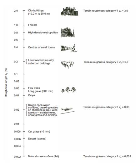
Figure 3.3: Description of terrain roughness lengths,  $z_o$  (ISO04353 (2012)).
