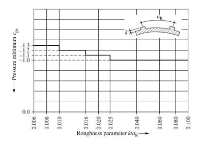
Figure 3.6: Surace roughness and types of pressure distribution (Phillip L. Gould; Wilfried B (2005)).
