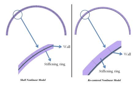
Figure 8.13: The configuration of the ring-wall connection for the Shell Nonlinear Model and Recentered Nonlinear Model
