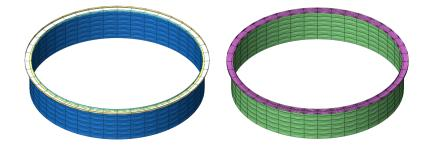
Figure 4.4: The mesh refinement of the top stiffening ring before(left) and after refinement(right)
