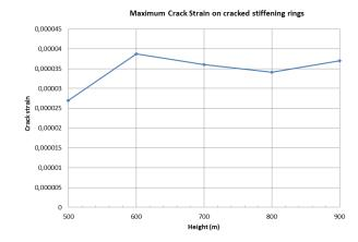
Figure 7.6: The maximum crack strain at the stiffening rings under self-weight (SNM)
