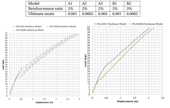
Table 8.2: The reinforcement ratio and ultimate strain of different models
