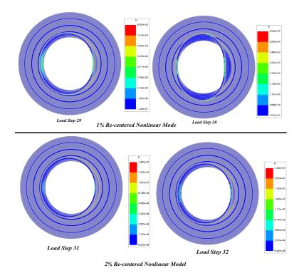
Figure 8.20: The principal strain distribution of 1%RNM and 2%RNM before and after the discontinuity
