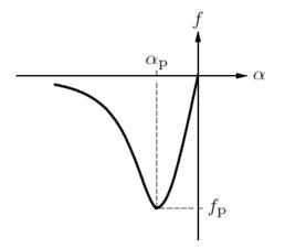
Figure 6.5: Thorenfeldt curve for concrete compressive behavior (DIANA (2016))
