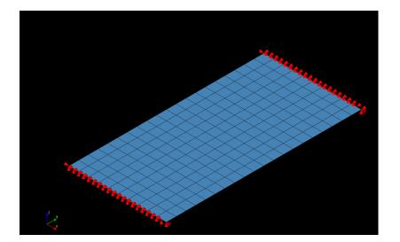
Figure B.1: 5x10m slab model with meshing and boundary conditions details
