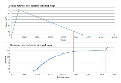
Figure 7.9: The comparison between concrete cracking model of the stiffening rings with maximum crack growth until load step 20 for SNM
