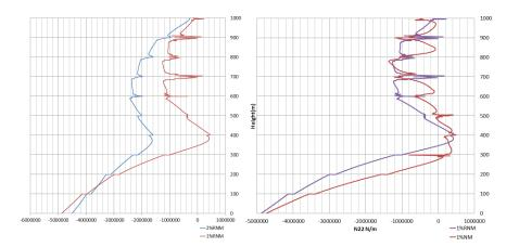
Figure D.7: The comparison of meridional stress distribution at the windward direction for 2%RNM, 1%RNM(left); the comparison of meridional stress distribution at the windward direction for 1%RNM, 1%NM,(right)
