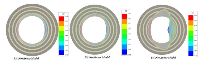
Figure 8.5: The deformed shape for 3%NM(left), 2%NM(middle), 1\$NM(right)
