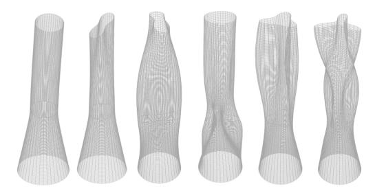
Figure 5.2: The first 6 free vibration mode shapes for Simple Linear Model the  $1^{st}$  (most left) and the  $6^{th}$  (most right)
