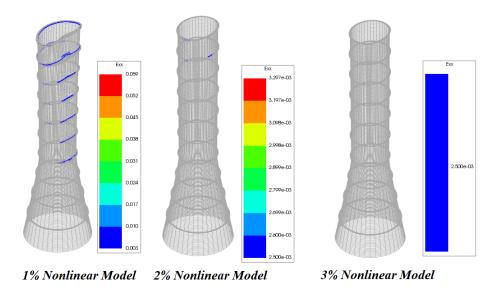
Figure 8.11: The yielding reinforcement distribution in circumferential direction of the model 1% Nonlinear Model, 2% Nonlinear Model, 3% Nonlinear Model
