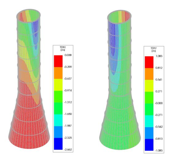
Figure E.2: The deformed shape with displacement distribution in x direction (left) and y direction (right) for 2%RNM under D+2W
