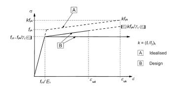
Figure 4.2: Stress-strain relation for reinforcement (EN1992-1-1 (2011))
