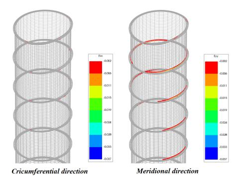
Figure 7.18: The distribution of concrete crushing in the circumferential direction(left) and the meridional direction(right) for SNM at 1D+1W
