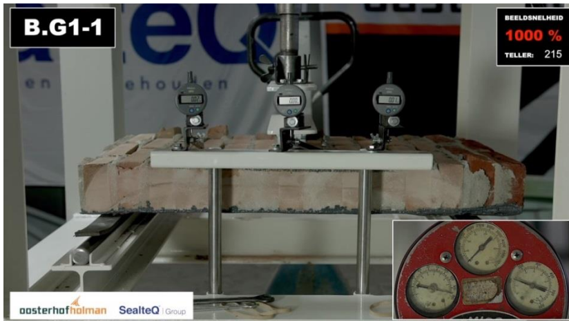
Figure 45: Test setup used for the OP bending test (screenshot taken from a Youtube movie of the Quake-Shield Youtube channel [43])
