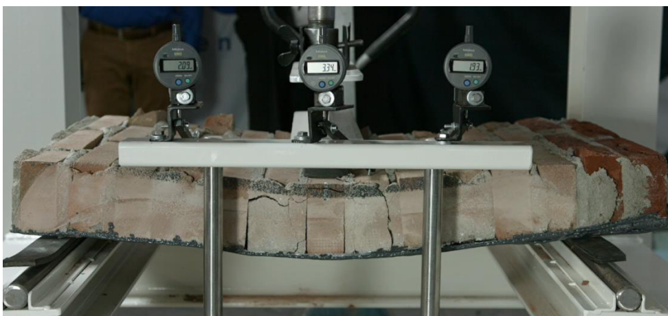
Figure 80: Test sample (BG1-1) at 33,4 mm displacement [43]
