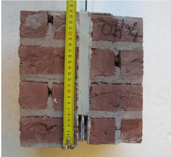
Figure 59: A sample from the pull-out tests performed by the TU/e [46]
