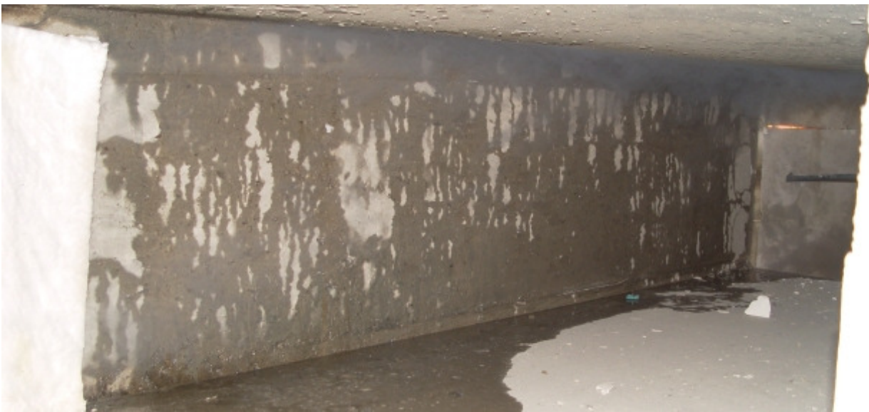
Water emerging from the middle wall after 30 minutes of heating. The photograph is taken from the unheated tunnel tube.
