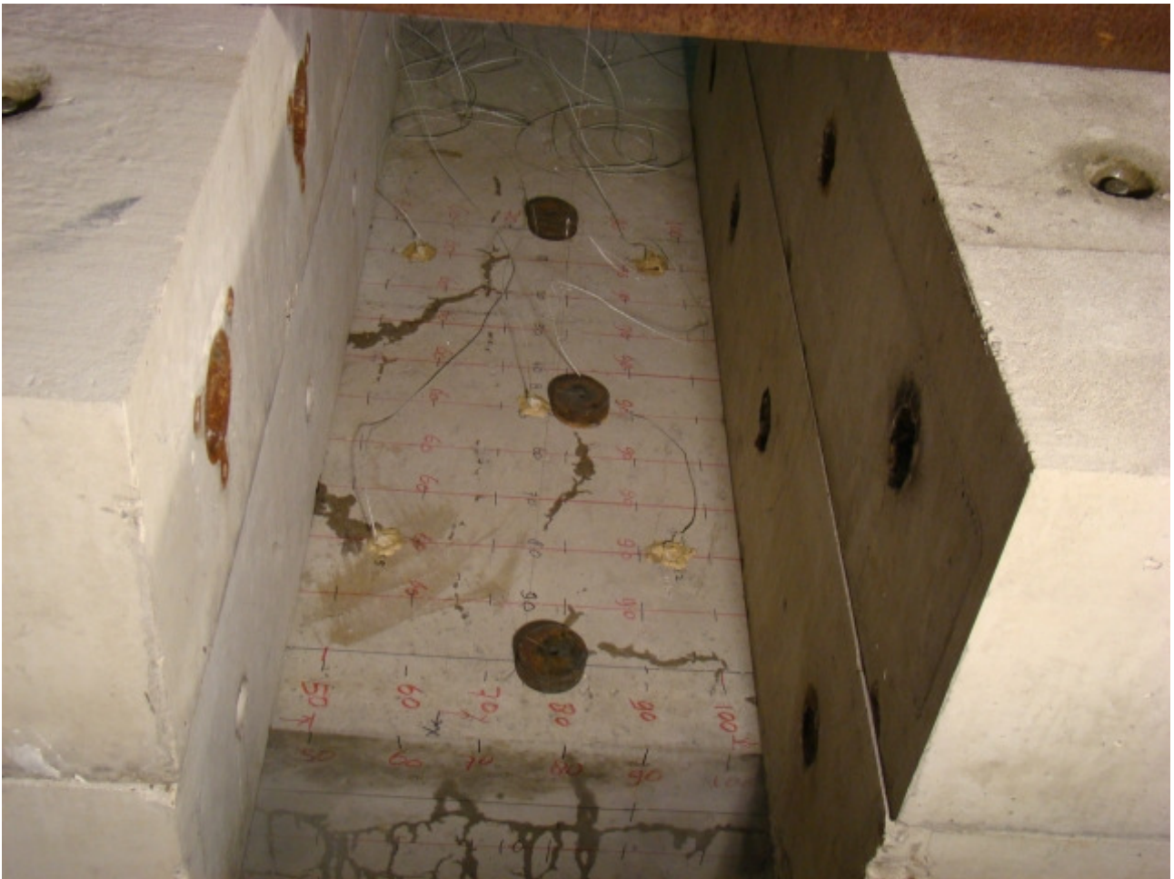
Only the small surface area between the blocks remained free for assessing crack widths.
