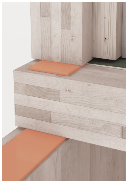
Figure 4.7: Application of resilient interlayer between walls and floor [60]
