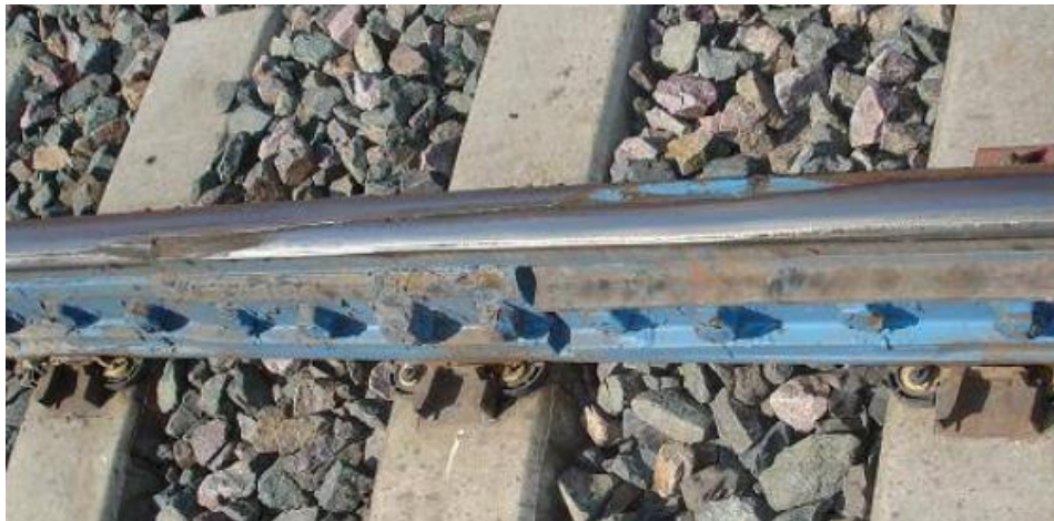
Figure 2.3: Long tapered test joint from (Akhtar,2007)
