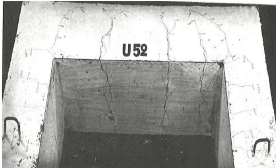
c). Crack pattern for corner without haunch
