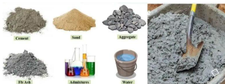
Figure 35 - Composition of raw materials concrete [44].
