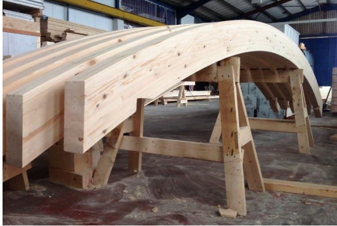
Figure 11 - Curved glued laminated beams [16].
