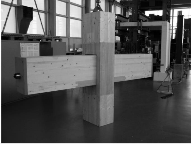
Figure 3 - Posttensioned timber connection made of glulam, darker areas indicate ash reinforcement.
