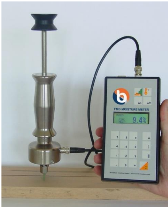
Figure 88 - FMD Moisture meter by Brookhuis. [57]
