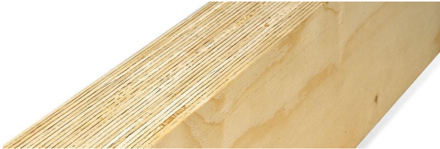
Figure 13 - Laminated veneer lumber, Kerto LVL S-beam [18].
