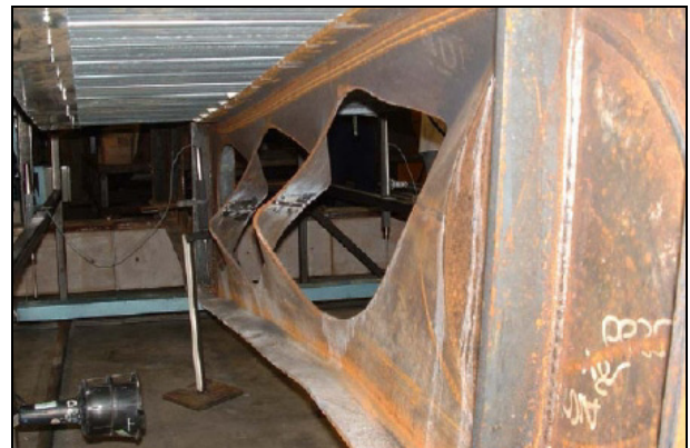
Figure 3.7 Web-post lateral-torsional buckling due to (vertical) shear
