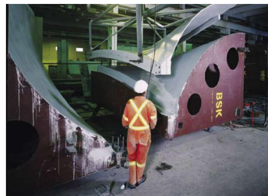
Fig.D21b. High precision steel mould for precast element LRT station [55]
