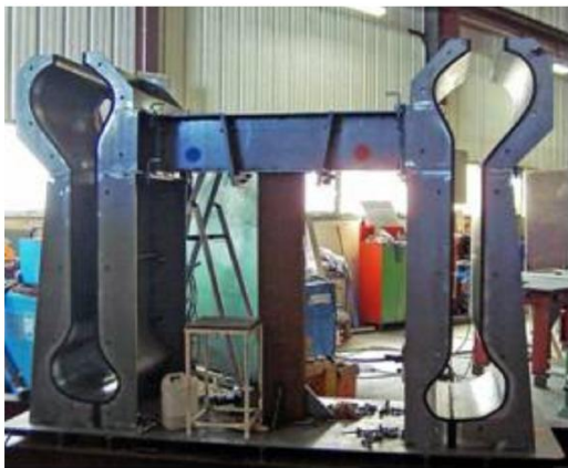
Fig.D21a. High precision steel mould for precast element Pont du Diable [56]
