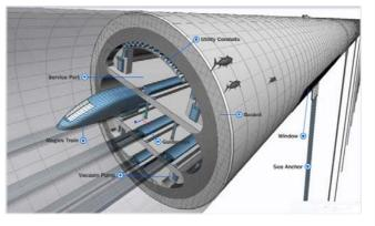
water and is moored to the seafloor by springs. The motion of the tunnel in water will be described using the Morrison equation for the hydrodynamic drag and the added mass concept. The train will be modelled as a set of uniformly moving loads.
