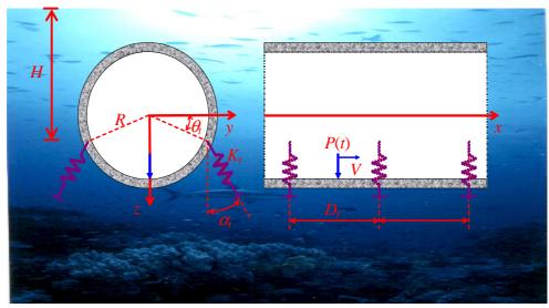
The aim of this project is to estimate the level of the tunnel vibrations induced by the train.
