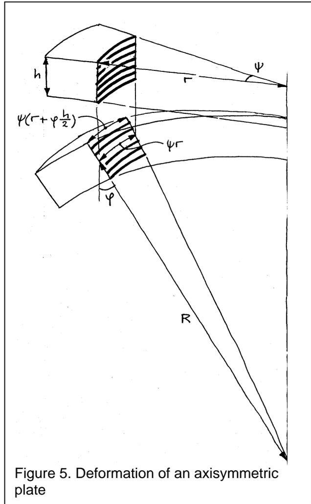
Figure 5. Deformation of an axisymmetric plate
