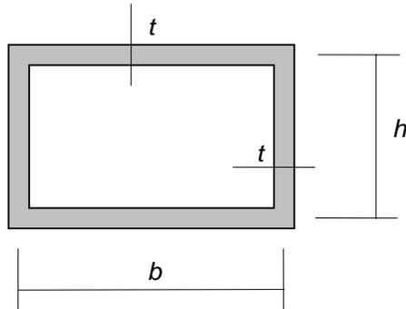
Figure 2. Cross-section of a rectangular tube
