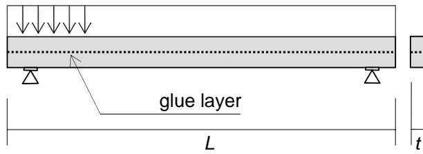
Figure 6. Glued timber beam
