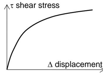
Figure 7. Shear stress-displacement diagram of a glue layer
