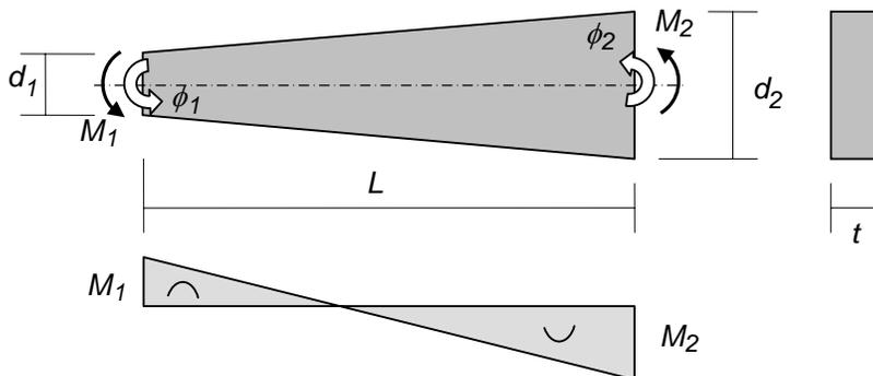
Figure 1. Non-prismatic beam element and moment distribution
