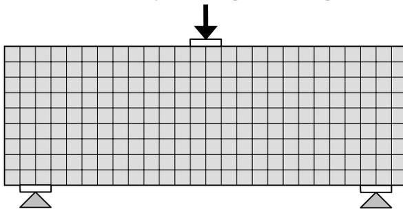
Figure 5. Finite element model of a deep beam
