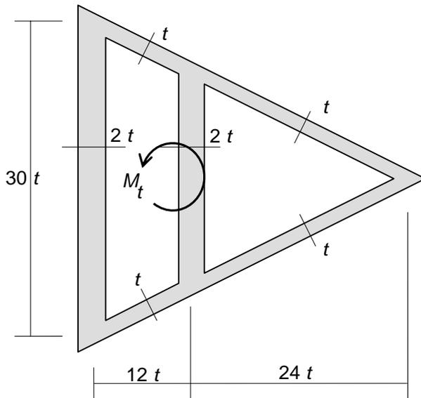
Figure 4. Cross-section of the core of a high-rise building
