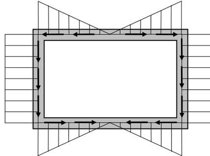
Figure 3. Shear stress distribution
