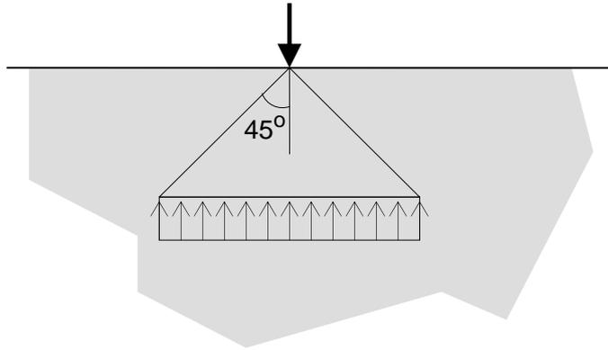
Figure 2. Point load on the edge of a large plate
