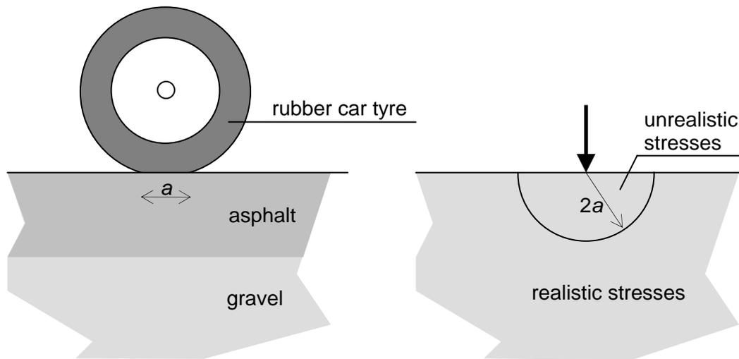
Figure 6. Car wheel on asphalt pavement
