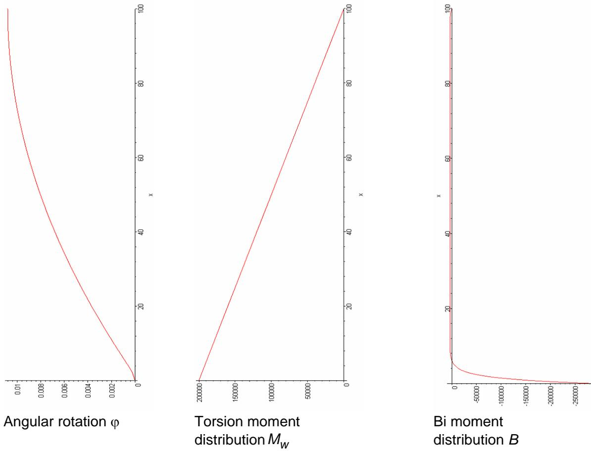
Figure 5. Torsion response of a 100 m high building
