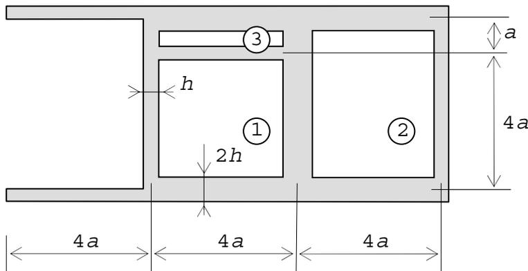
Figure 4. Cross-section of a stability core
