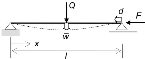
Figure 3. Simply supported beam
