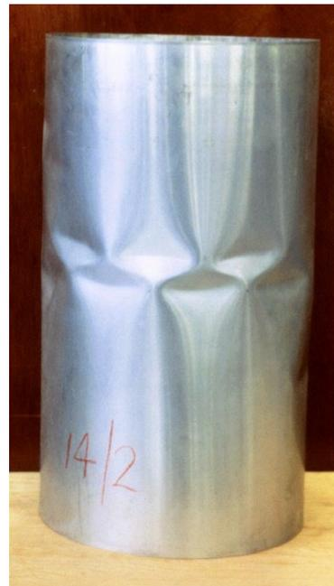
Figure 183. Yoshimura buckling of an aluminium cylinder
