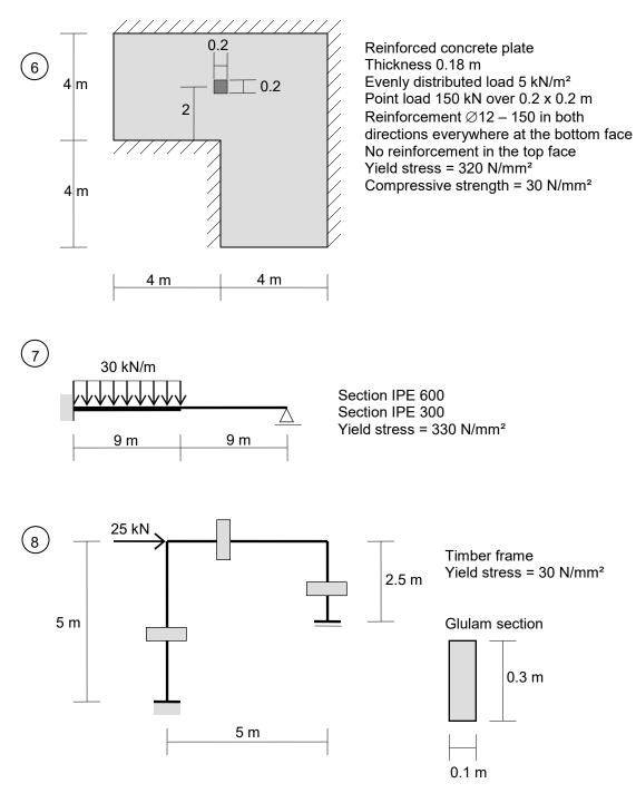
The moment capacity of the joints is the same as the moment capacity of the members.
