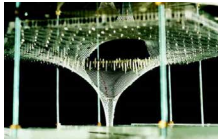
(b) Tension model of Frei Otto [67].
