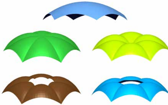
FIGURE 8.9 Diverse numerical inverted hanging geometry [149].
