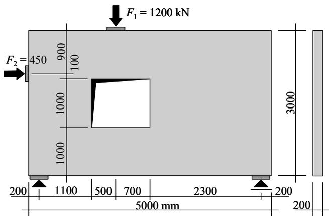
Fig. 5 Deep beam with opening
