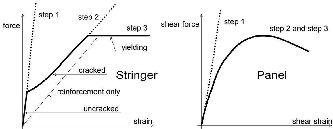
**Fig. 2** Non-linear constitutive behaviour of stringers and panels in SPanCAD
