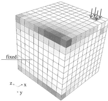
Figure 4. The normal stress  $\sigma_{xx}$  on the surface of the concrete block. The largest value is  $6.17 \text{ N/mm}^2$ . The smallest value is  $-8.52 \text{ N/mm}^2$ .
