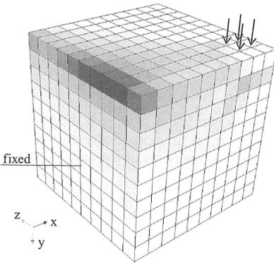
Figure 5. Optimal reinforcement ratio  $\rho_x$ . The largest value is 1.48%.
