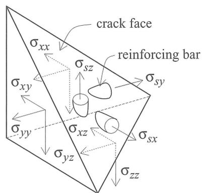
Figure 1. Elementary part of reinforced concrete. Shown are a crack and the reinforcing bars that bridge this crack.
