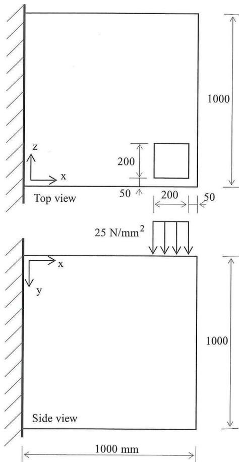
Figure 3. Concrete block loaded by a vertical force (dimensions in mm).
