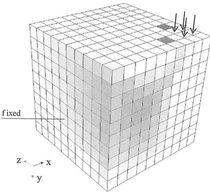
Figure 6. Optimal reinforcement ratio  $\rho_y$ . The largest value is 0.56%.
